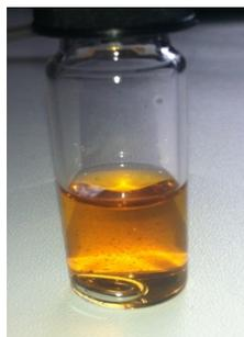
**Figure S6.** Catalytic mixture containing 100  $\mu\text{L}$  of liquid mercury
