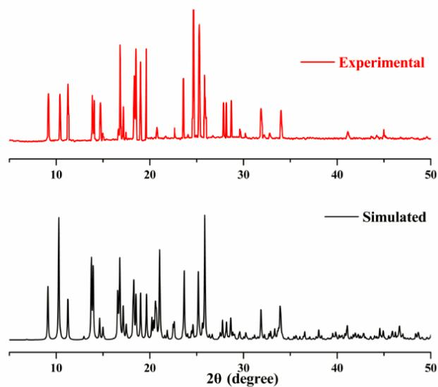
**Figure S9.** Powder X-ray diffraction patterns of complex **4**
