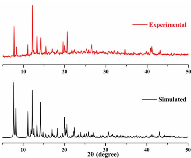
**Figure S10.** Powder X-ray diffraction patterns of complex **5**
