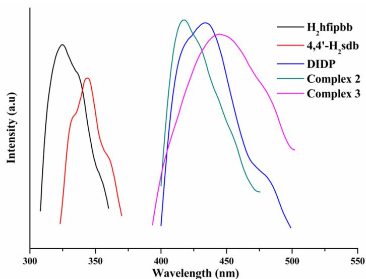
Figure S12. Solid-state photoluminescent spectra of **2**, **3** and corresponding ligands at room temperature
