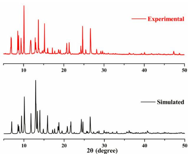
**Figure S6.** Powder X-ray diffraction patterns of complex 1
