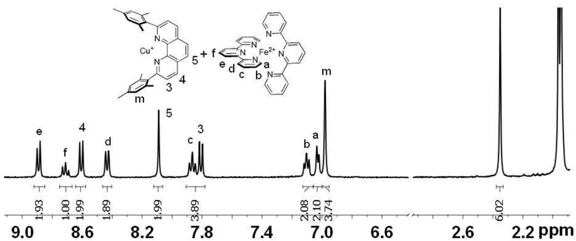
**Figure S24:** <sup>1</sup>H NMR spectrum (400 MHz, CD<sub>2</sub>Cl<sub>2</sub>, 298 K) obtained after adding 0.5 equiv. of Fe<sup>2+</sup> to [Cu(2)(3)]<sup>+</sup>. The spectrum indicates presence of [Cu(2)]<sup>+</sup> and [Fe(3)<sub>2</sub>]<sup>2+</sup>.
