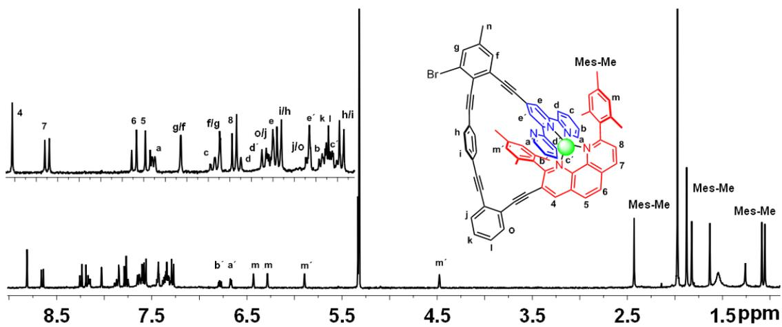
Figure S13:  $^1\text{H}$  NMR spectrum (400 MHz,  $\text{CD}_2\text{Cl}_2$ , 298 K) of complex  $[\text{Cu}(\mathbf{1})]^+$ .
