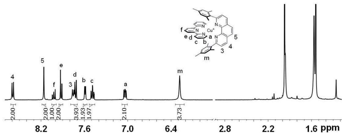
**Figure S23:** <sup>1</sup>H NMR spectrum (400 MHz, CD<sub>2</sub>Cl<sub>2</sub>, 298 K) of complex [Cu(2)(3)]<sup>+</sup>.
