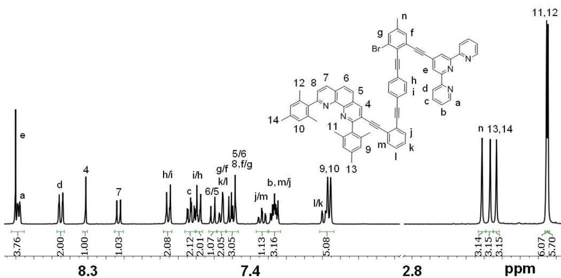
Figure S11:  $^1\text{H}$  NMR spectrum (400 MHz,  $\text{CD}_2\text{Cl}_2$ , 298 K) of nanoswitch 1.
