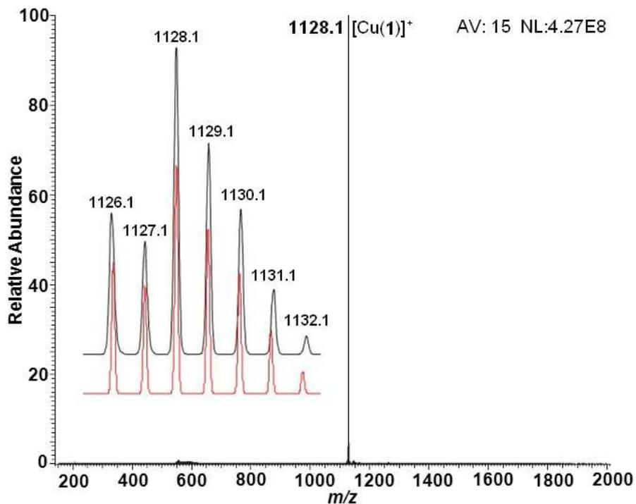
Figure S31: ESI-MS spectrum of complex [Cu(1)]<sup>+</sup> in DCM.
