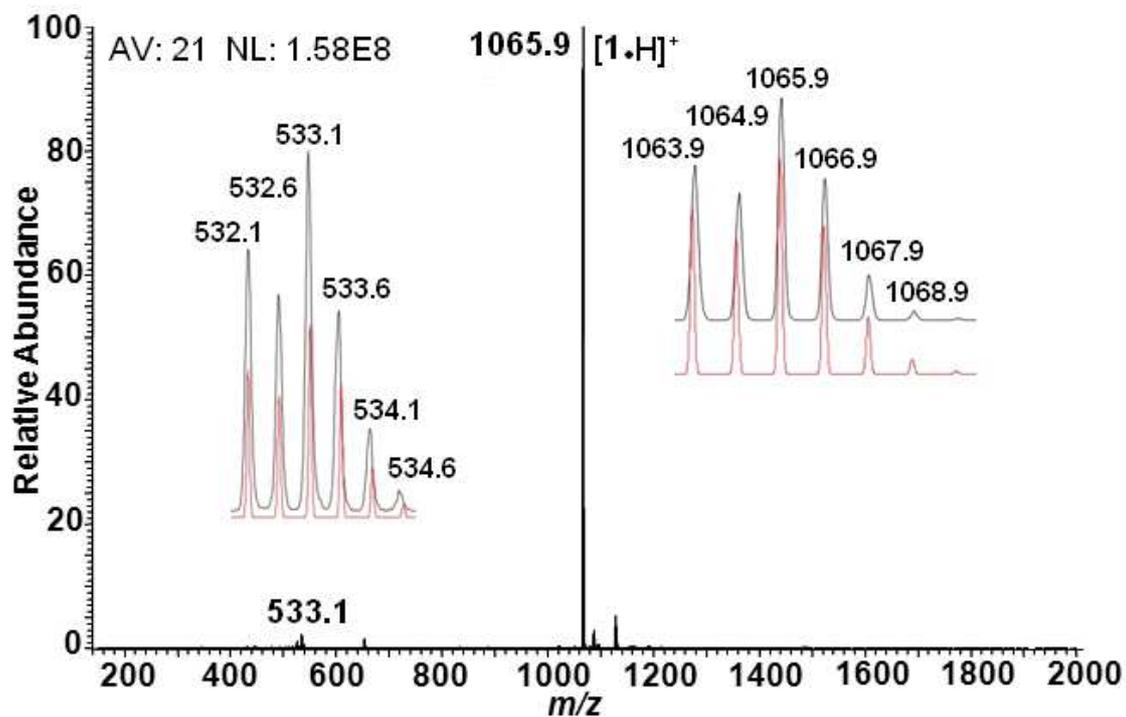
Figure S30: ESI-MS spectrum of nanoswitch [1•H]<sup>+</sup> in DCM.
