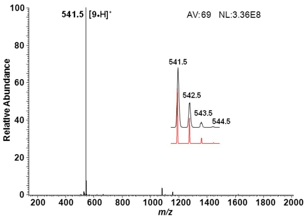
Figure S28: ESI-MS of compound **9** in CH<sub>2</sub>Cl<sub>2</sub> at 298K.
