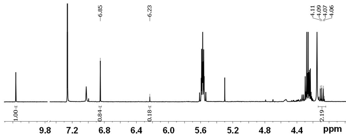
**Figure S35:**  $^1\text{H}$  NMR obtained after heating a mixture of **11** and **12** at 55 °C for 4 h in presence of 10 mol% of  $[\text{Cu}(\mathbf{2})]^+$  ( $\approx 1$  mM). The peaks at 4.06-4.11 ppm show the formation of cyclopropanated product **13** and the peaks at 6.23 and 6.85 ppm represent **14** and **15** respectively. The cyclopropanated product **13** was obtained in 49% yield along with 19% of **14** and 4% of **15**.
