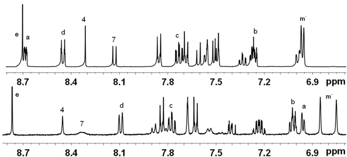
**Figure S21:** Partial  $^1\text{H}$  NMR spectrum (400 MHz, 298 K) of (top) nanoswitch **1** in  $\text{CD}_2\text{Cl}_2$ , (bottom) after addition of 0.5 equiv. of  $\text{Fe}^{2+}$  to nanoswitch **1** in  $\text{CD}_2\text{Cl}_2$ :  $\text{CD}_3\text{CN}$  = 3: 1 (v/v). The upfield shifts of protons a-, b-, d-H and downfield shifts of c-, e-H are indicative of the formation of  $[\text{Fe}(\mathbf{1})_2]^{2+}$ .
