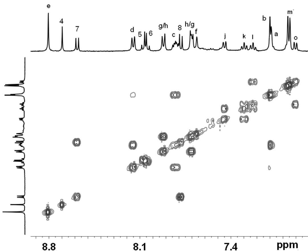
**Figure S19:**  $^1\text{H}$ - $^1\text{H}$  COSY spectrum (400 MHz,  $\text{CD}_2\text{Cl}_2$ :  $\text{CD}_3\text{CN}$  = 3: 1, 298 K) of complex  $[\text{Fe}(\text{Cu}(\mathbf{1}))_2]^{4+}$ . Aromatic region is expanded.
