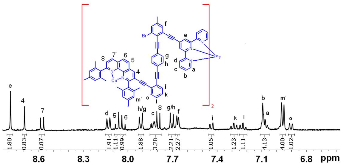
**Figure S18:**  $^1\text{H}$  NMR spectrum (400 MHz,  $\text{CD}_2\text{Cl}_2$ :  $\text{CD}_3\text{CN}$  = 3: 1, 298 K) of complex  $[\text{Fe}(\text{Cu}(\mathbf{1}))_2]^{4+}$ . Aromatic region is expanded.
