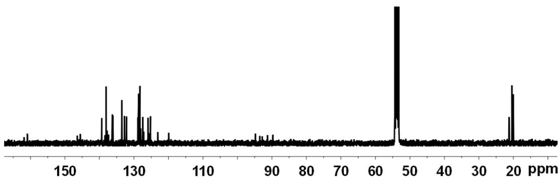
Figure S 10:  $^{13}\text{C}$  NMR spectrum (100 MHz,  $\text{CD}_2\text{Cl}_2$ , 298 K) of compound 10.
