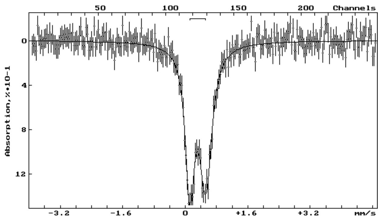
Figure S4.  $^{57}\text{Fe}$  Mössbauer spectrum of  $\{\text{FeBd}_2(\text{IGm})(\text{BF})_2\}_2$
