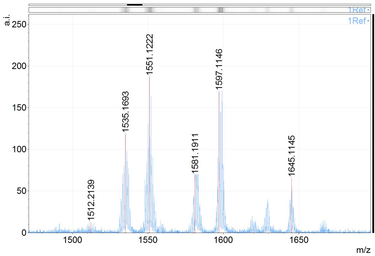
Figure S5. MALDI-TOF mass spectrum of  $\{\text{FeBd}_2(\text{BrGm})(\text{BF})_2\}_2$
