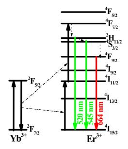
Fig. s1 Simplified energy level diagrams of Yb<sup>3+</sup>/Er<sup>3+</sup>. The green and red light centered at 520/545 and 664 nm, which can be attributed to the electronic transition  ${}^{2}\text{H}_{11/2}{}^{/4}\text{S}_{3/2} \rightarrow {}^{4}\text{I}_{15/2}$  and  ${}^{4}\text{F}_{9/2} \rightarrow {}^{4}\text{I}_{15/2}$  of Er<sup>3+</sup> ions.
