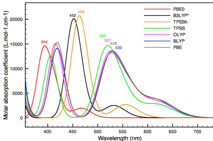
**Figure S1** : TDDFT absorption spectrum computed with the seven tested functionals in the 355-755 nm range
