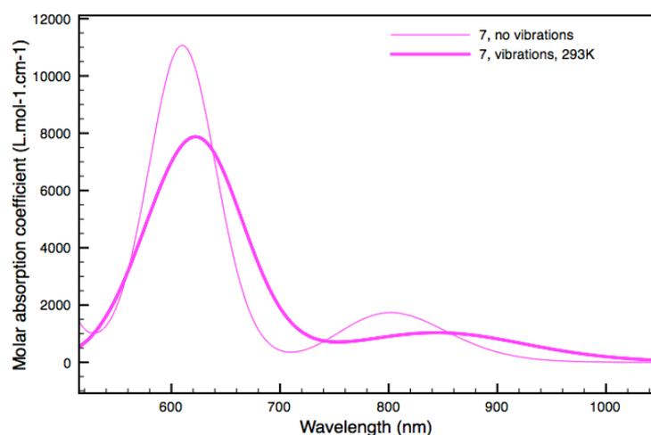
**Figure S2** : Including vibrations (thick lines) in the calculation of the TDDFT absorption spectra (thin lines) of complexes **1** (top), **5** (centre) and **7** (bottom).
