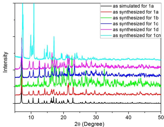
**Figure S3A.** The powder X-ray diffraction (PXRD) patterns for 1a-1cn
