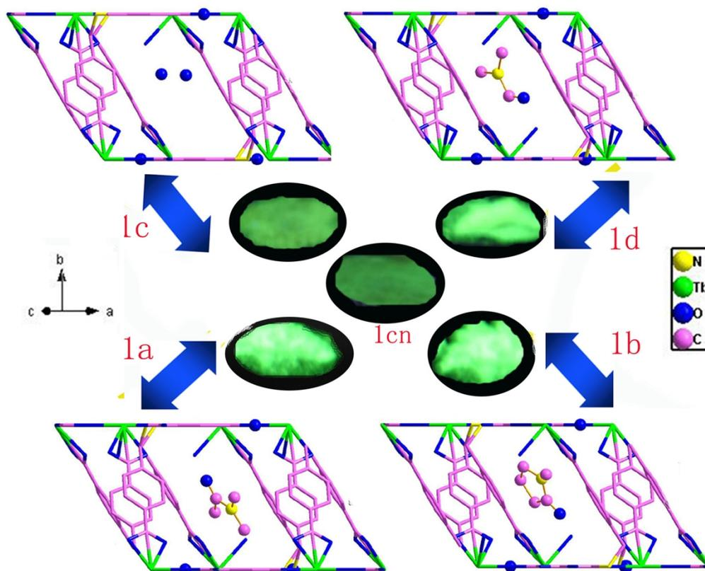
**Fig. S13.** The frameworks and luminescence photos of **1a-1d**: guest molecules (DMA, NMP, H<sub>2</sub>O and DMF) are filling in the frameworks (viewing from [101] direction).
