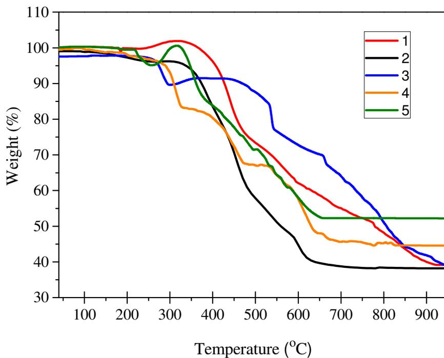
**Figure S8.** Thermogravimetric data, collected under a flowing O<sub>2</sub> atmosphere, for compounds 1-5.
