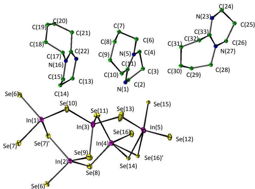
**Figure S4.** Local coordination diagram of non-hydrogen atoms for  $[\text{C}_9\text{H}_{17}\text{N}_2]_3[\text{In}_5\text{Se}_{8.74}(\text{Se}_2)_{0.26}]$  (**2**) showing the atom labelling scheme and ellipsoids at 50% probability.
