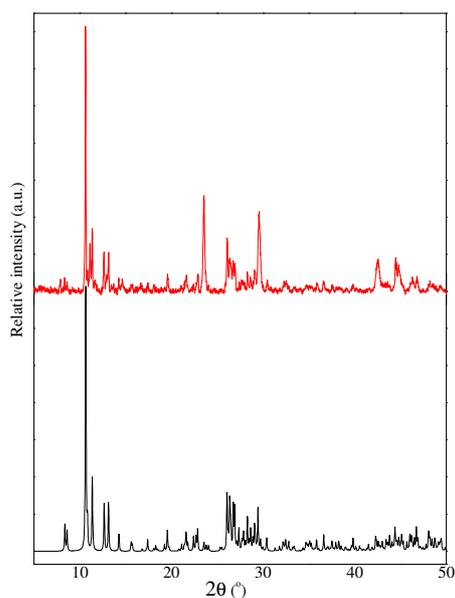
**Figure S2.** Experimental powder X-ray diffraction pattern (red) for the bulk product of the reaction producing **5**. The pattern calculated using the structure determined by single crystal X-ray diffraction is shown in black.
