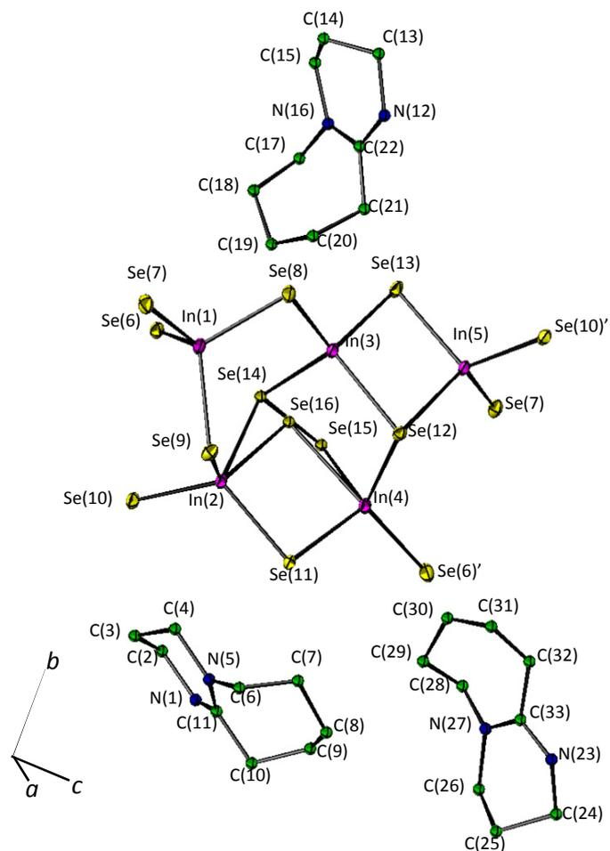
**Figure S3.** Local coordination diagram of non-hydrogen atoms for  $[\text{C}_9\text{H}_{17}\text{N}_2]_3[\text{In}_5\text{Se}_{8.07}(\text{Se}_2)_{0.93}]$  (**1**) showing the atom labelling scheme and ellipsoids at 50% probability.
