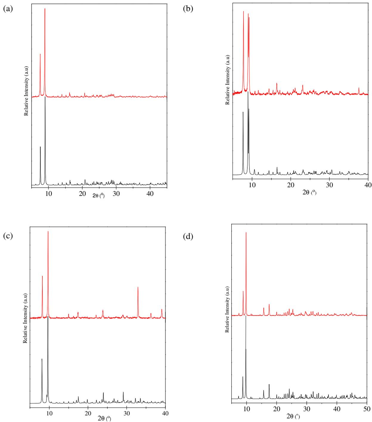
**Figure S1.** Experimental powder X-ray diffraction pattern (red) for the bulk product of the reaction producing (a) **1**, (b) **2**, (c) **3** and (d) **4**. The pattern calculated using the structure determined by single crystal X-ray diffraction is shown in black.
