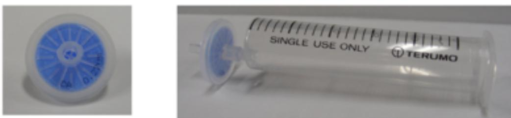
**Figure S7.** Photograph of prepared filter fixed with the micro crystal **1-SO<sub>4</sub>** (left), and the syringe (right) attached with the filter.
