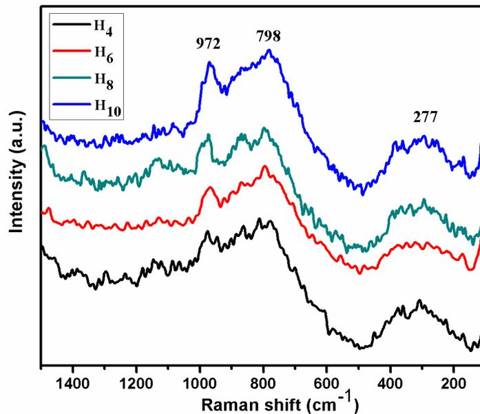
**Fig. S2** Raman spectra of  $\text{WO}_3$  thin film deposited at different hydrothermal time.
