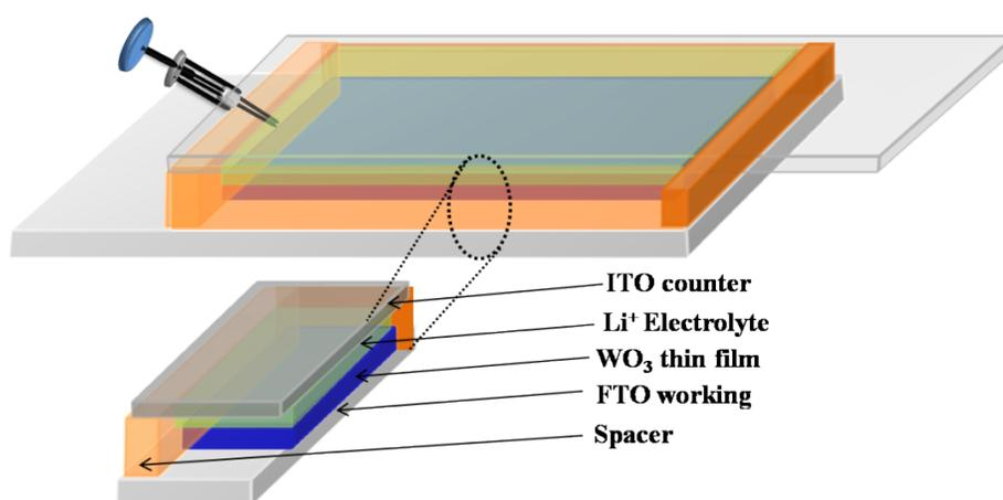
**Fig. S1**A schematic representation of EC device fabrication of honeycomb nanostructured  $WO_3$  thin film.
