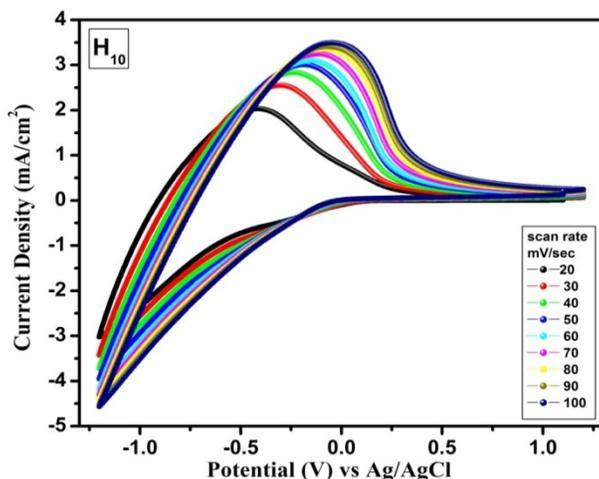
**Fig. S4** Cyclic voltammograms of nanostructured  $\text{WO}_3$  thin film recorded at different scan rate.
