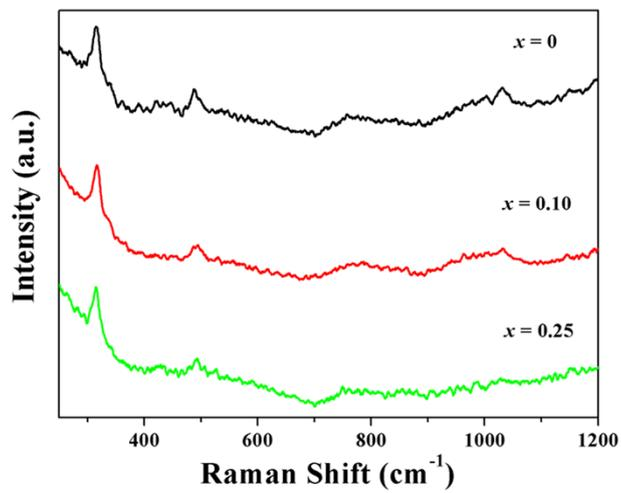
5 **Fig. S3** The Raman spectra of  $\text{Ca}_{0.99+x}\text{Gd}_{1-x}\text{Al}_{1-x}\text{Si}_x\text{O}_4:\text{Eu}_{0.01}$  ( $x = 0, 0.10$  and  $0.25$ ) samples.
