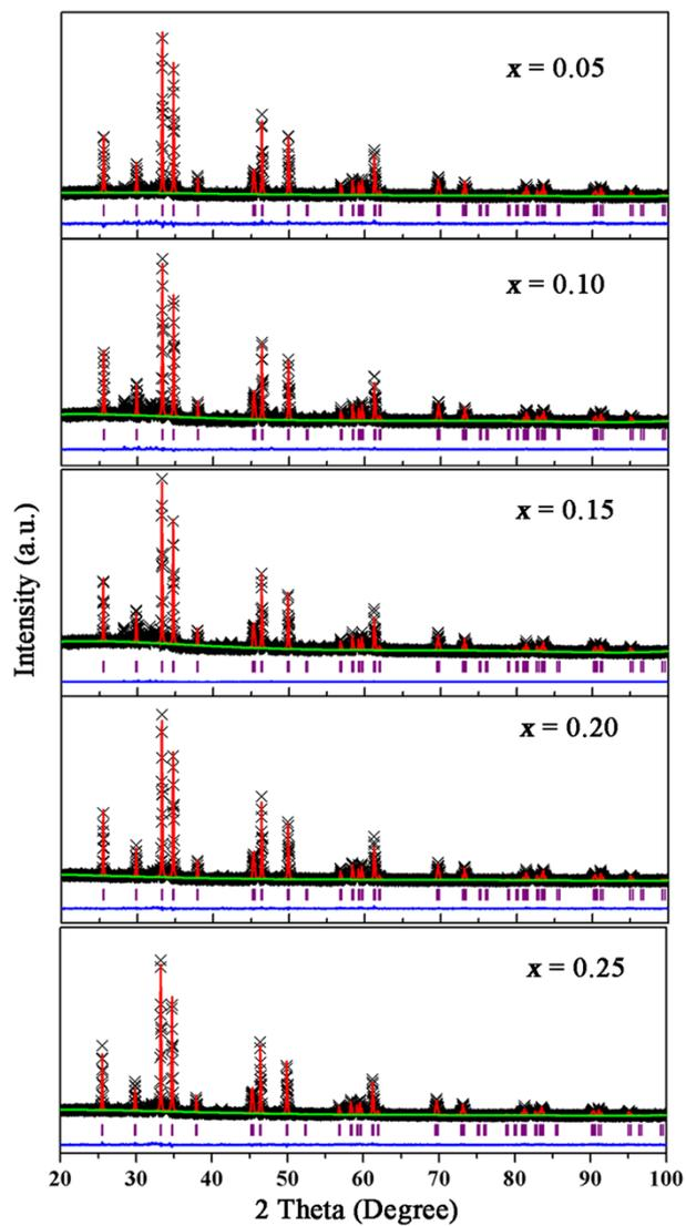
5 **Fig. S1** The Rietveld refinement to XRD patterns for  $\text{Ca}_{0.99+x}\text{Gd}_{1-x}\text{Al}_{1-x}\text{Si}_x\text{O}_4:\text{Eu}_{0.01}$  ( $x = 0.05-0.25$ ), respectively.
