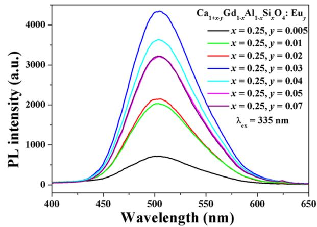
5 Fig. S6 The influence of doping concentration of Eu ions on the emission intensity of the obtained Ca<sub>1+x-y</sub>Gd<sub>1-x</sub>Al<sub>1-x</sub>Si<sub>4</sub>O<sub>4</sub>:Eu<sub>y</sub> ( $x = 0.25, y = 0.005-0.07$ ) phosphors,  $\lambda_{ex} = 335 \text{ nm}$ .
