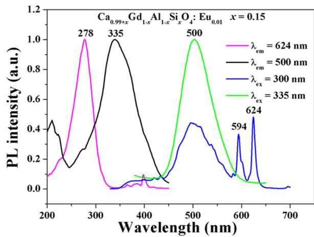
5 **Fig. S4** The PLE and PL spectra Ca<sub>0.99+x</sub>Gd<sub>1-x</sub>Al<sub>1-x</sub>Si<sub>x</sub>O<sub>4</sub>:Eu<sub>0.01</sub> ( $x = 0.15$ ) sample.
