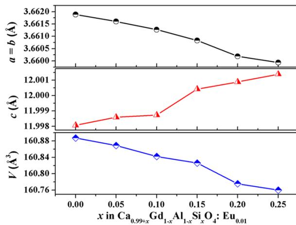
5 **Fig. S2** Unit cell parameters of  $\text{Ca}_{0.99+x}\text{Gd}_{1-x}\text{Al}_{1-x}\text{Si}_x\text{O}_4:\text{Eu}_{0.01}$  ( $x = 0-0.25$ ) obtained from Rietveld refinement, reflecting the effects of the  $\text{Si}^{4+}$ - $\text{Ca}^{2+}$  incorporation.
