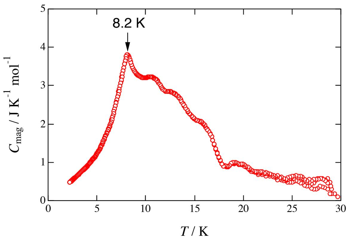
Figure S5. Temperature dependence of the specific heat capacity  $C_{\text{mag}}$  in BBDTA•Au(CN)<sub>2</sub>.
