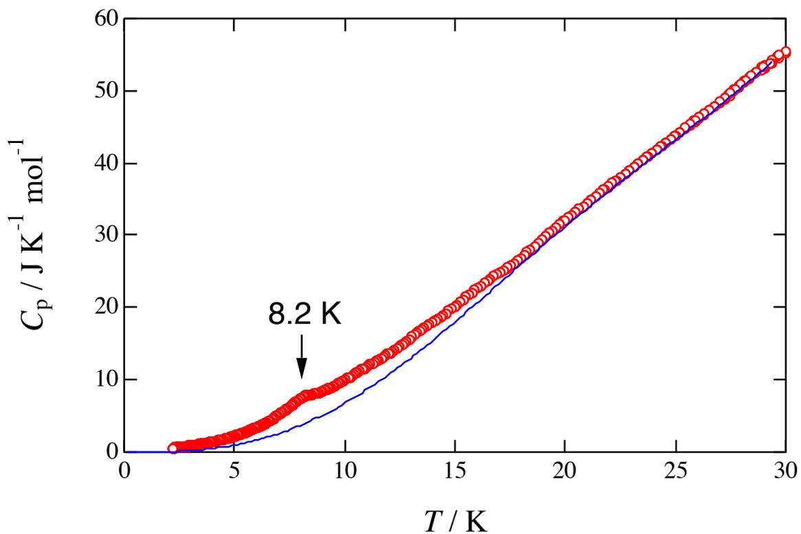
Figure S4. Temperature dependence of the total heat capacity  $C_{\text{mag}}$  in BBDTA•Au(CN)<sub>2</sub>. The blue solid line expresses the contribution of the lattice,  $C_{\text{lattice}}$ .
