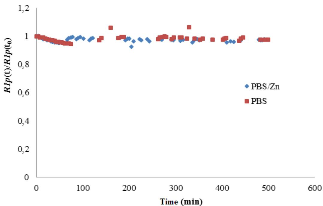
**Figure SII2.** Time evolution of the relative water proton paramagnetic relaxation rate  $R1p(t)/R1p(t_0)$  (20 MHz, 25 °C) for a solution of  $GdL_2@AuNPs$  (1.30 mM in PBS 10 mM, pH 7.1) ( $\blacksquare$ ) and following addition of 0.75 mM  $ZnCl_2$  ( $\blacklozenge$ ).
