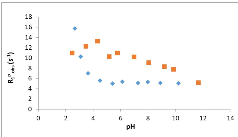
**Figure SI3.** pH dependence of the water proton longitudinal relaxation rate for GdL<sub>1</sub> (20 MHz, 1.0 mM, 25 °C (■)) and for GdL<sub>2</sub> (20 MHz, 1.13 mM, 25 °C (◆)).
