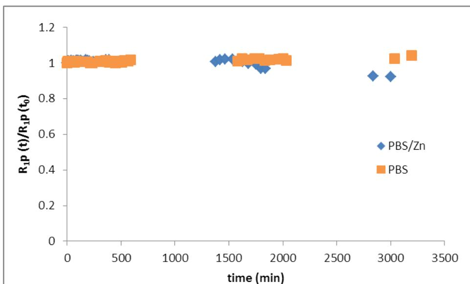
**Figure SI4.** Time evolution of the relative water proton relaxation rate  $R_{1P}(t)/R_{1P}(0)$  (20 MHz, 37 °C) for a solution of GdL<sub>2</sub> (1.13 mM in PBS 2.5 mM, pH 7.1) (◆) and following addition of ZnCl<sub>2</sub> 0.75 mM (■).
