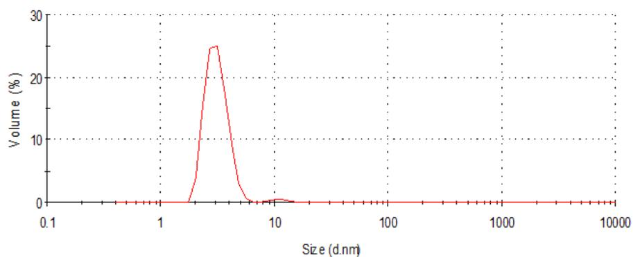
**Figure S12.** Size distribution (%Volume) for GdL<sub>2</sub> (5.67 mM, pH 7.1, 25 °C).
