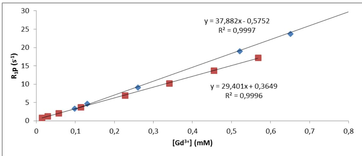
**Figure SI9.** Concentration dependence of the paramagnetic water proton relaxation rate  $R_{1p}$  ( $R_{1p} = R_{1obs} - R_{1d}$ ) for GdL1@NPs (■) and GdL2@NPs (◆) (20 MHz, 25 °C, pH 7.1).
