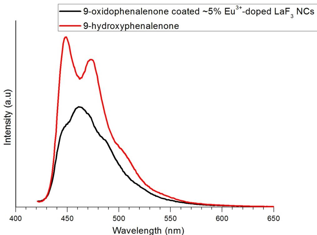
**Figure S8:** An overlap of the ligand fluorescence spectra of 9-hydroxyphenalenone ligand (red) and 9-oxidophenalenone coated ~5% Eu<sup>3+</sup>-doped LaF<sub>3</sub> NCs (black) in THF.
