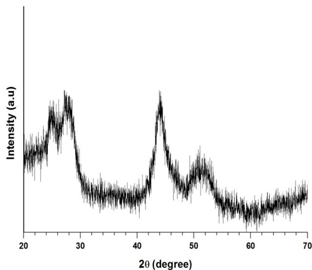
**Figure S1:** Powder XRD pattern of citrate capped 5%  $\text{Eu}^{3+}$ -doped  $\text{LaF}_3$  NCs. The diffraction peaks are indexed to the  $\text{LaF}_3$  tysonite structure (ICDD code: 01-082-0690).
