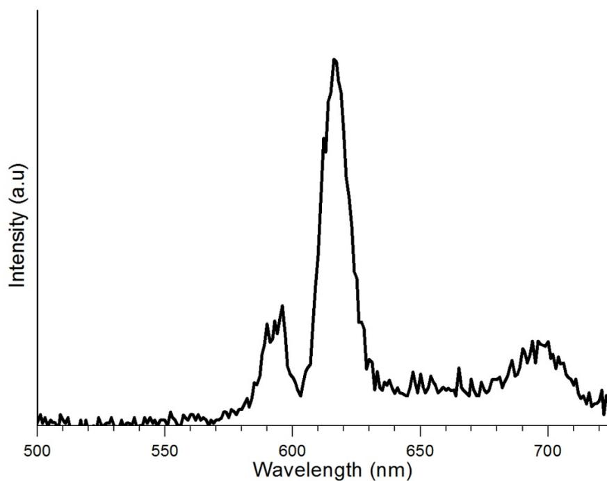
**Figure S9:** Emission spectrum of a dried (solid) sample of 9-oxidophenalenone coated ~5% Eu<sup>3+</sup>-doped LaF<sub>3</sub> NCs collected upon excitation of the organic capping ligands at 457 nm, with 0.1 ms delay time (phosphorescence mode).
