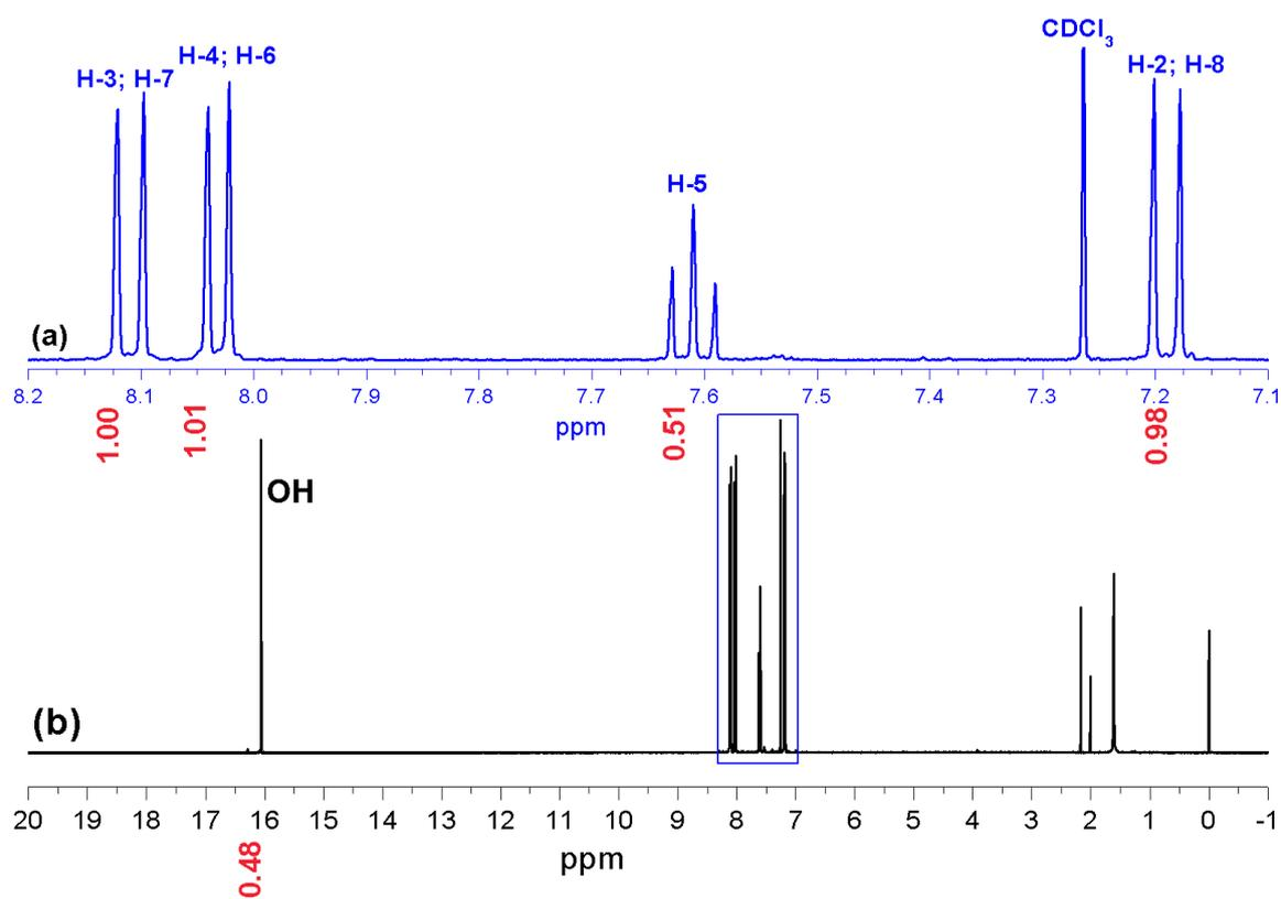
**Figure S5:** The  $^1\text{H}$  NMR spectrum of 9-hydroxyphenalenone in  $\text{CDCl}_3$ , (a) full spectrum and (b) expansion of 7.1-8.2 ppm region. The spectrum was recorded on 400 MHz Bruker Avance III spectrometer. The proton resonances are assignments according to the literature (*J. Chem. Edu.*, 2008, **85**, 413).
