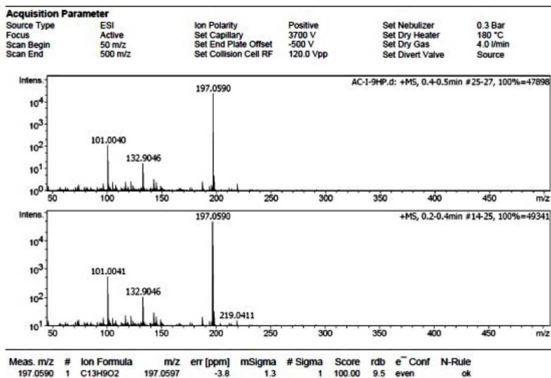
**Figure S4:** Electrospray ionisation mass spectrum in positive ion mode (ESI-MS<sup>+</sup>) of 9-hydroxyphenalenone ligand recorded on Bruker Maxis Impact mass spectrometer.
