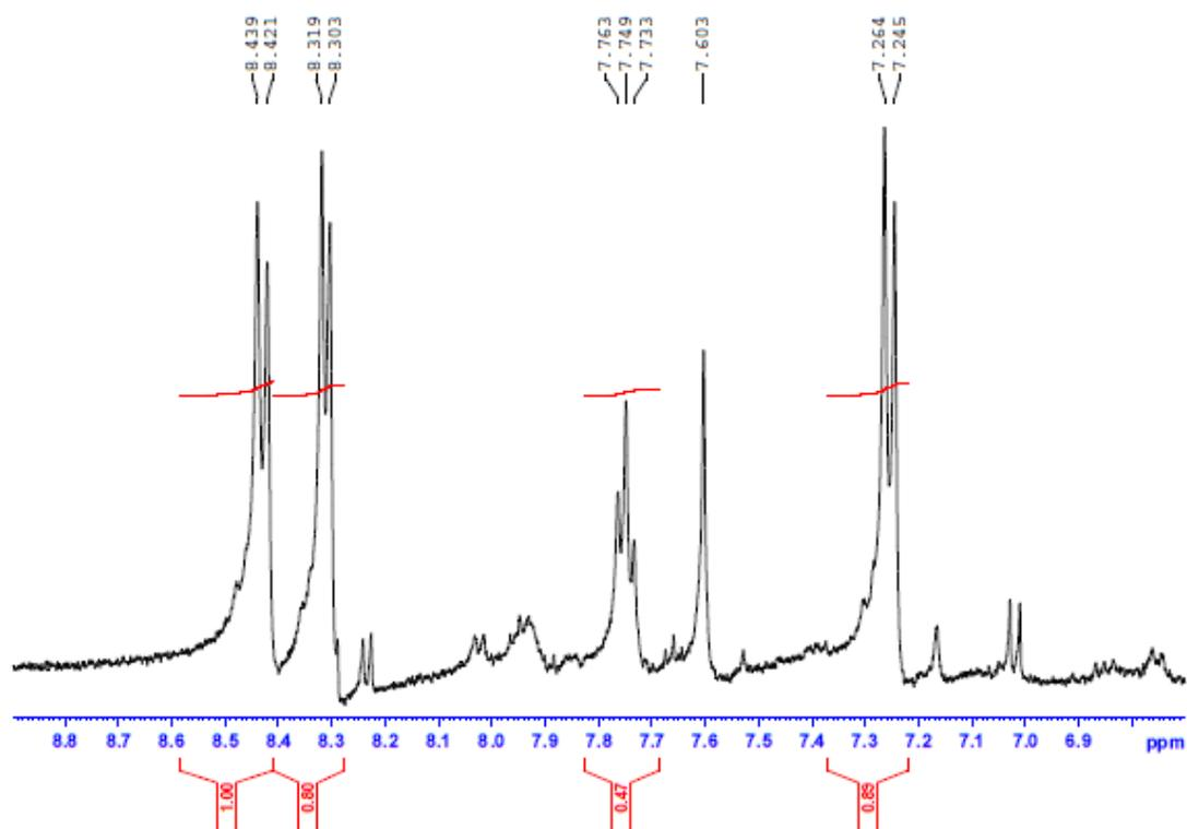
**Figure S6:** The  $^1\text{H}$  NMR spectrum 9-oxidophenalenone coated  $\sim 5\%$   $\text{Eu}^{3+}$ -doped  $\text{LaF}_3$  NCs in  $\text{DMSO-d}_6$ . The spectrum was recorded on 400 MHz Bruker Avance III spectrometer.
