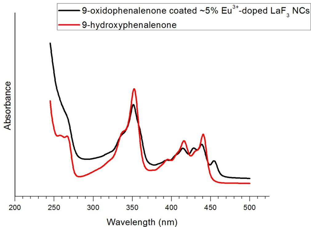
**Figure S7:** An overlap of the absorption spectra of 9-hydroxyphenalenone ligand (red) and 9-oxidophenalenone coated ~5% Eu<sup>3+</sup>-doped LaF<sub>3</sub> NCs (black) in THF.
