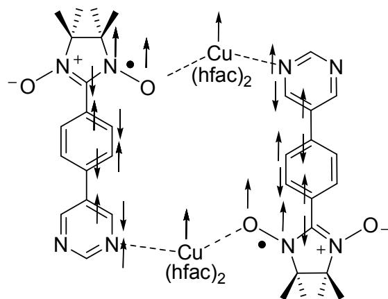
**Chart S1.** Spin polarization mechanism for the magnetic coupling mediated by NITPhPyrim ligand.
