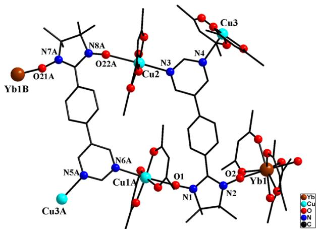
**Figure S4.** Crystal structure of complex **3**. Hydrogen atoms and fluorine atoms are not shown for the sake of clarity. (A: $1+x, y, z$ ; B: $x, 3/2-y, -1/2+z$ )
