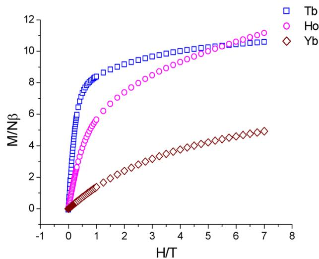
**Figure S7.**  $M$  versus  $H/T$  plots for complexes **1-3** at 2.0 K.
