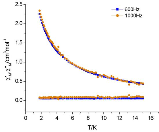
**Figure S8.** Temperature dependence of the in-phase and out-of-phase components of the ac magnetic susceptibility for **2** in zero dc fields with an oscillation of 3.0 Oe.
