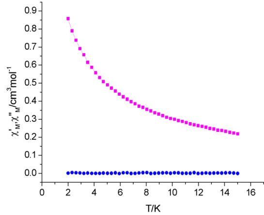
**Figure S9.** Temperature dependence of the in-phase and out-of-phase components of the ac magnetic susceptibility for **3** in zero dc fields with an oscillation of 3.0 Oe. (AC frequency:100Hz)
