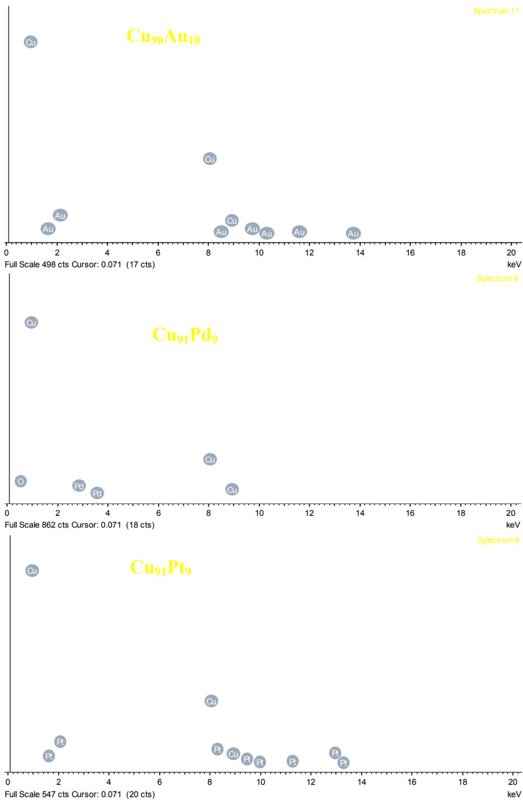
**Fig. 13 EDS spectra of various kind of bimetallic nanostructures with the Au, Pt and Pd.**
