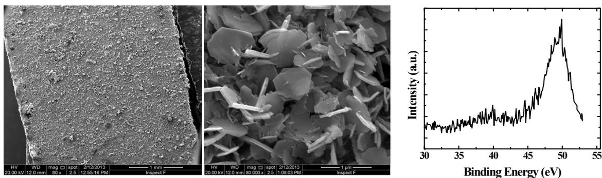
Fig.7 (A & B) SEM images of  $\text{Mg}(\text{OH})_2$  nanostructures formation on Mg foil surfaces when we performed the experiment in absence of acid medium. (C) XPS spectrum of Mg 2p in  $\text{Mg}(\text{OH})_2$  (corresponding of to the binding energy 49.6 eV).<sup>1</sup>
