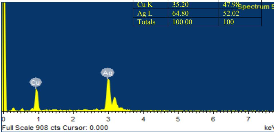
Fig. SEM images with different magnifications and EDS spectra of  $Ag_{65}Cu_{35}$ .
