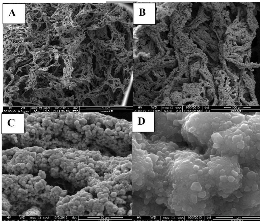
Fig.6 SEM images of spongy Cu obtained with 2.5 ml of 0.2 M  $\text{CuSO}_4 \cdot 5\text{H}_2\text{O}$  solution and 0.5 ml of 5M  $\text{H}_2\text{SO}_4$ . No change in morphology was observed when 0.1 M  $\text{CuSO}_4 \cdot 5\text{H}_2\text{O}$  solution was used. However, the amount was half in quantity.
