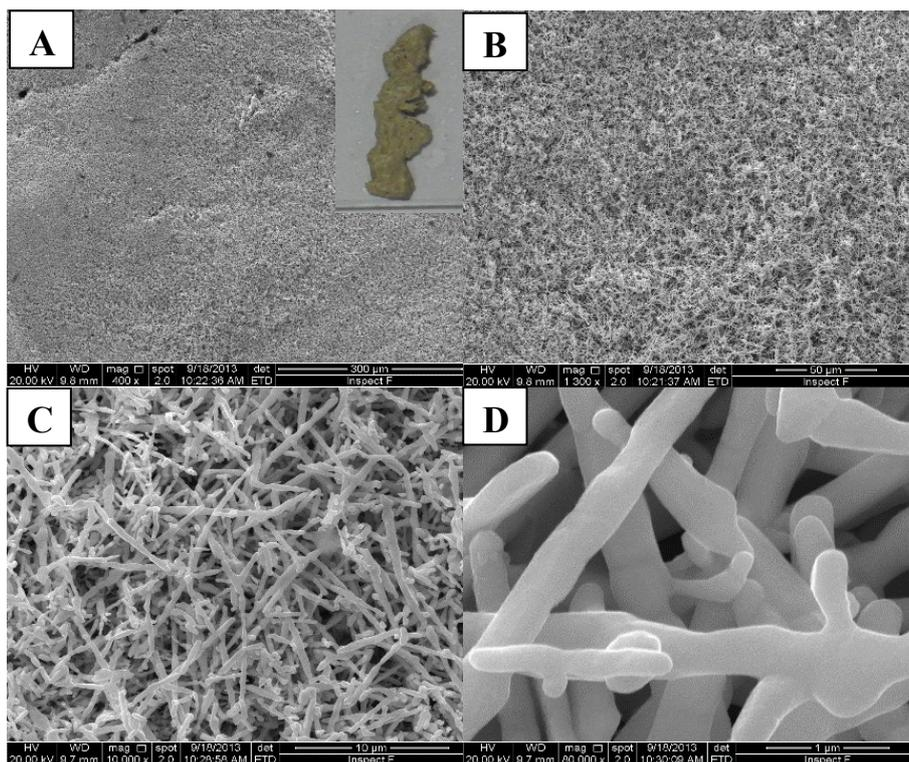
**Fig.3 (A-D) SEM images of different magnification of spongy Ag nanostructures obtained with 2.5 ml of 0.05 M AgNO<sub>3</sub> and 0.6 ml of 5M H<sub>2</sub>SO<sub>4</sub>.**
