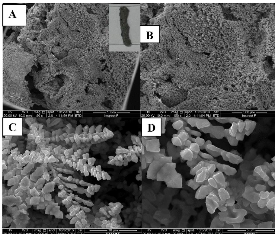
Fig.5 SEM images of spongy Sn obtained with 2.5 ml of 0.2 M  $\text{SnCl}_2 \cdot 2\text{H}_2\text{O}$  and 0.6 ml of 5M  $\text{H}_2\text{SO}_4$ .
