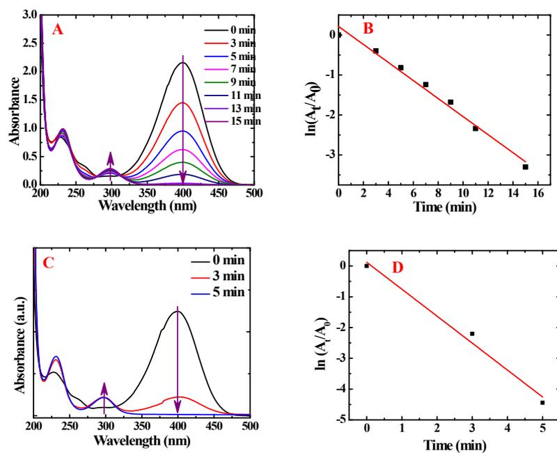
**Fig. 16 (A and B) 4-NP reduction by commercially available bulk Cu powder (10 ml of 1 mM 4-NP and 10 ml of 50 mM  $\text{NaBH}_4$  solution and 5 mg of catalyst) and its pseudo first order rate kinetics plot. (C and D) 4-NP reduction by  $\text{Cu}_{35}\text{Ag}_{65}$  and its pseudo first order rate kinetics plot.**
