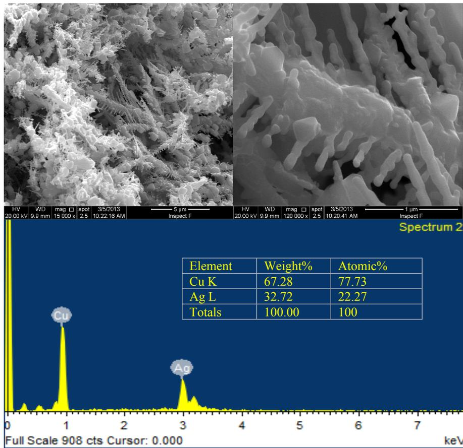
**Fig. 9 SEM images with different magnifications and EDS spectra of  $\text{Ag}_{33}\text{Cu}_{67}$ .**
