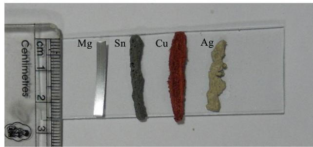
**Fig1.** Photograph of ~2.5 cm of Mg ribbon and Sn, Cu and Ag sponge structures after complete etching of the Mg ribbon.
