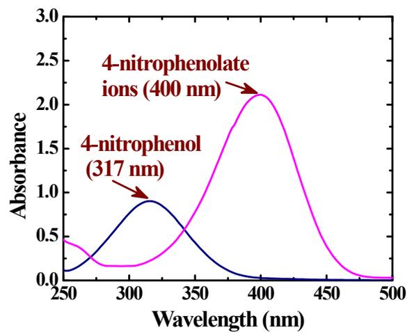
**Fig.15 UV-vis spectra of 4-nitrophenol before and after adding NaBH<sub>4</sub> solution.**
