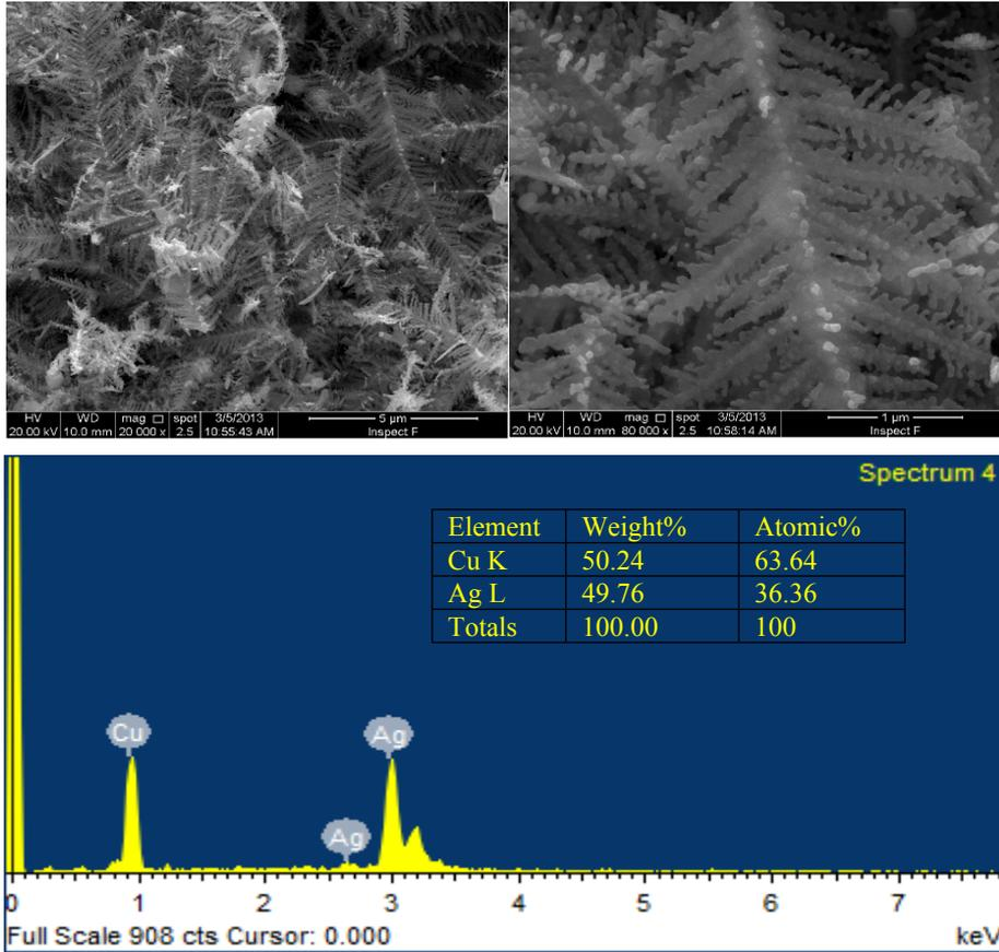
Fig. 10 SEM images with different magnifications and EDS spectra of  $\text{Ag}_{50}\text{Cu}_{50}$ .
