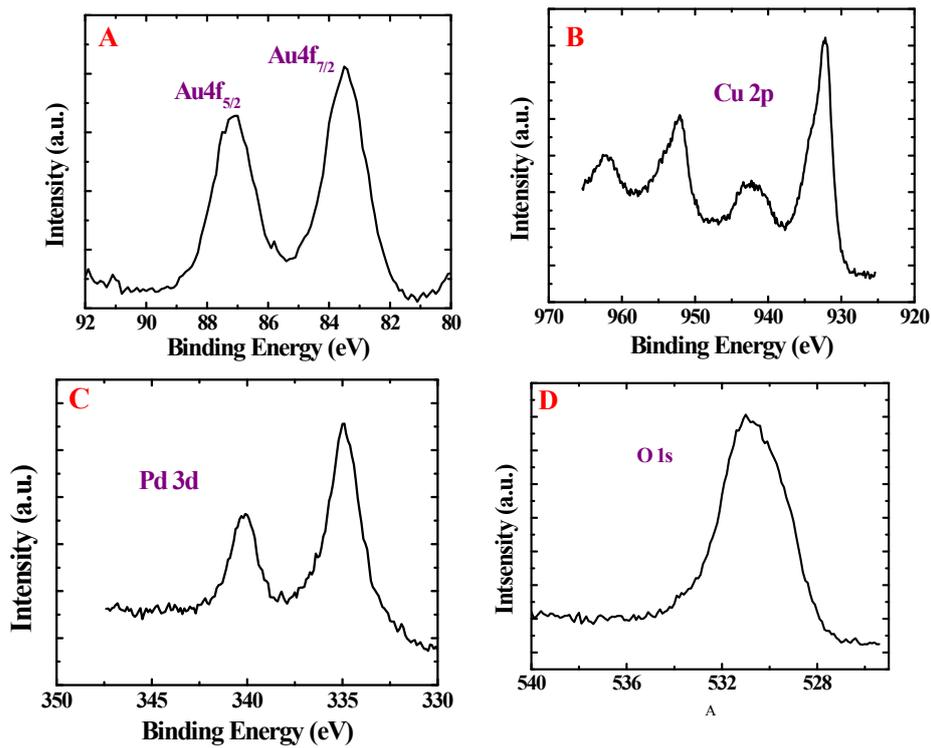
**Fig. 14 (A-D) High resolution XPS spectra of individual Cu, Pd, Au and O in CuPdAu dendritic nanostructures.**
