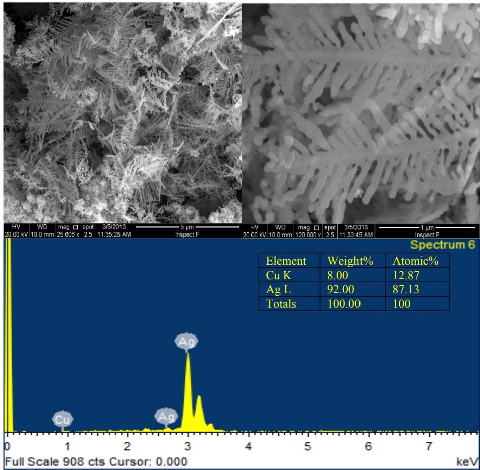
Fig. 12 SEM images with different magnifications and EDS spectra of  $\text{Ag}_2\text{Cu}_8$ .
