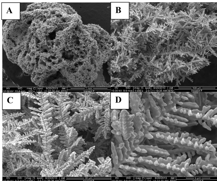
Fig.4 SEM images of spongy Sn obtained with 2.5 ml of 0.1M  $\text{SnCl}_2 \cdot 2\text{H}_2\text{O}$  and 0.6 ml of 5 M  $\text{H}_2\text{SO}_4$ .
