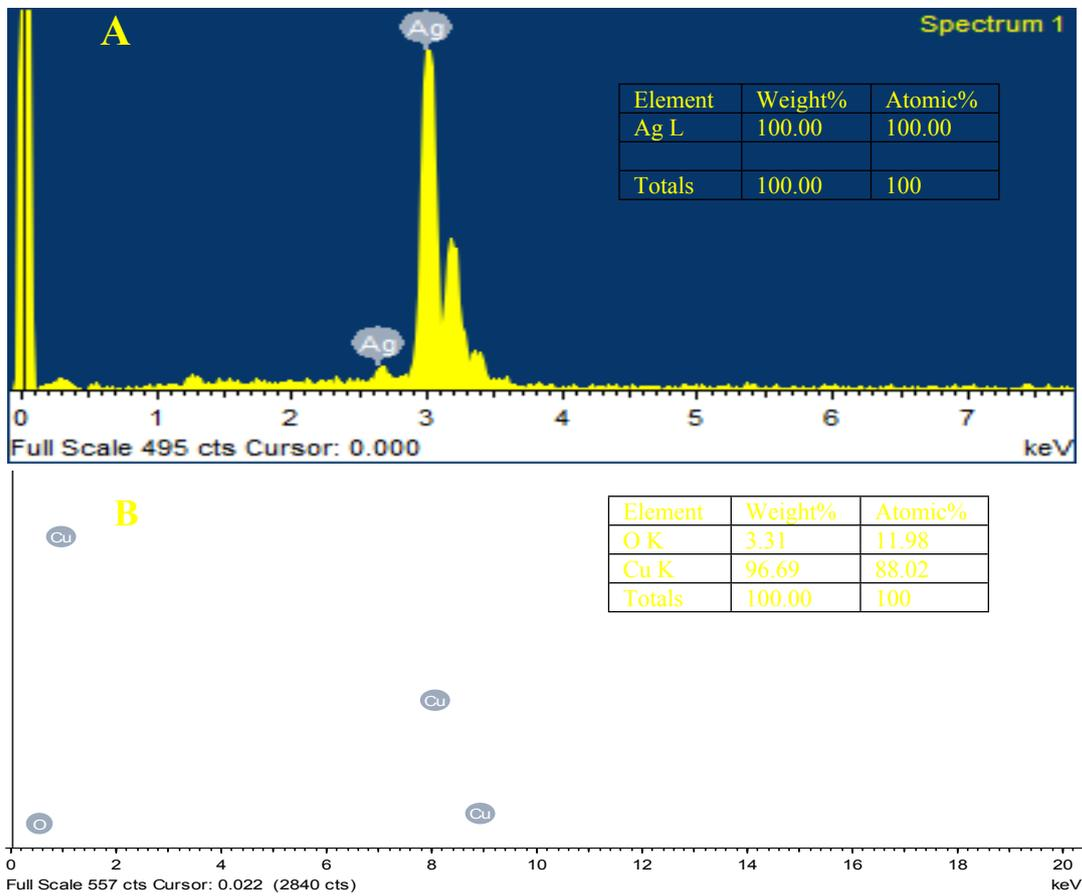
**Fig. 8.** (A and B) EDS spectra of spongy Ag and Cu nanostructures .
