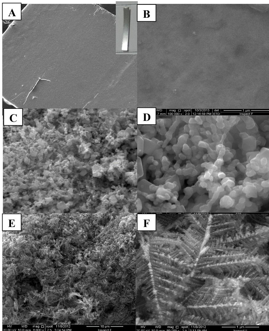
**Fig.2** SEM images of Mg ribbon (A & B) and Cu (C & D) and Ag (E & F) nanostructures grown on the Mg ribbon (inset) in absence of acid.
