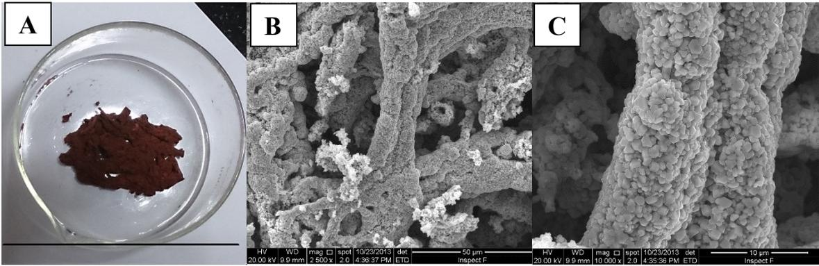
**Fig.8** Photograph and SEM images of spongy structures of gram scale synthesis of Cu. The scale bar corresponds to 9 cm.
