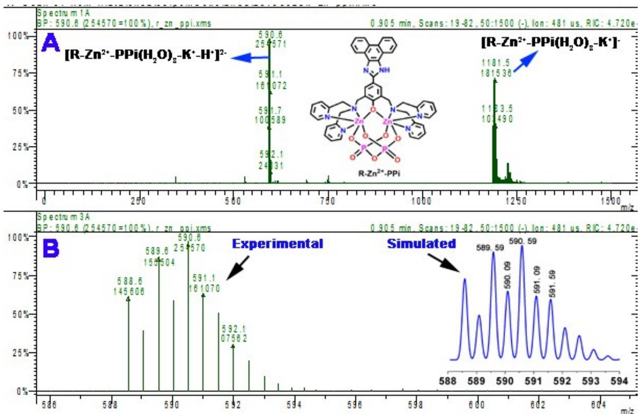
**Fig. S11** (A) Mass spectrum of  $R-Zn^{2+}-PPi$  obtained in negative mode. Peaks at  $m/z = 590$  and 1181, correspond to  $[C_{47}H_{55}N_8O_{16}P_2Zn_2]^{2-}$  ( $= [R-Zn^{2+}-PPi (H_2O)_8 -K^+-H^+]^{2-}$ ) and  $[C_{47}H_{56}N_8O_{16}P_2Zn_2]^{-}$  ( $= [R-Zn^{2+}-PPi (H_2O)_8 - K^+]^{-}$ ), respectively. (B) Measured and simulated isotopic distributions of peak at  $m/z = 590$ .
