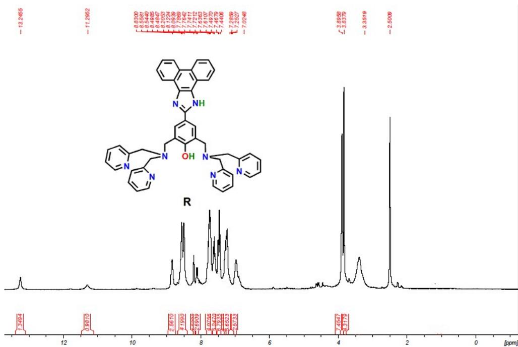
Fig. S3 <sup>1</sup>H NMR spectrum of **R** recorded in DMSO-d<sup>6</sup>.
