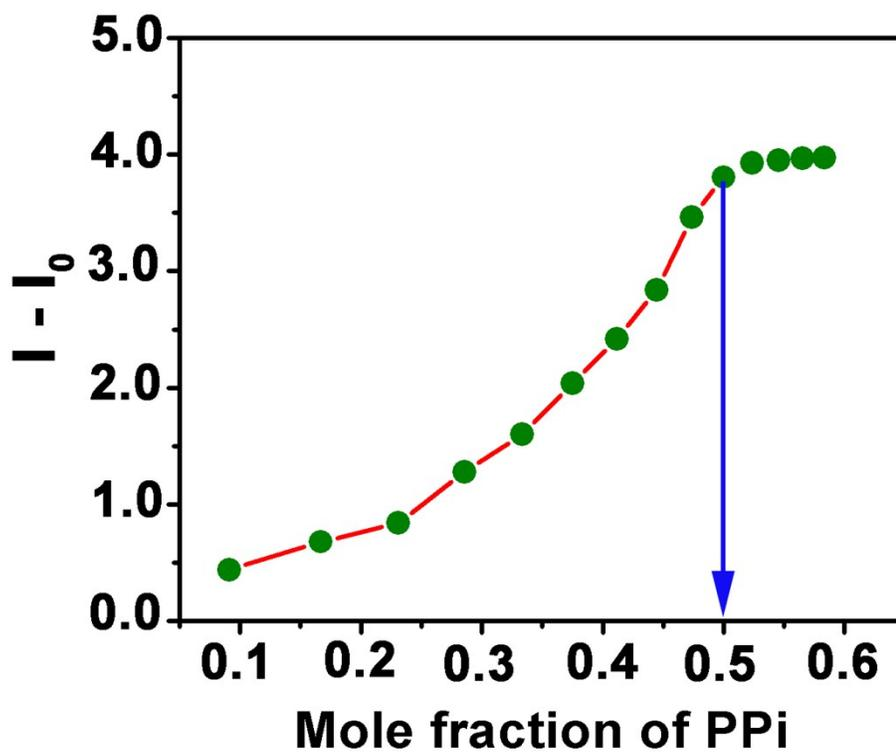
**Fig. S9** Stoichiometry plot of  $(F-F_0)$  against mole fraction of PPI ( $F$  and  $F_0$  are the fluorescent intensities of  $\mathbf{R-Zn}^{2+}$  at a particular concentration of PPI and in the absence of PPI, respectively).
