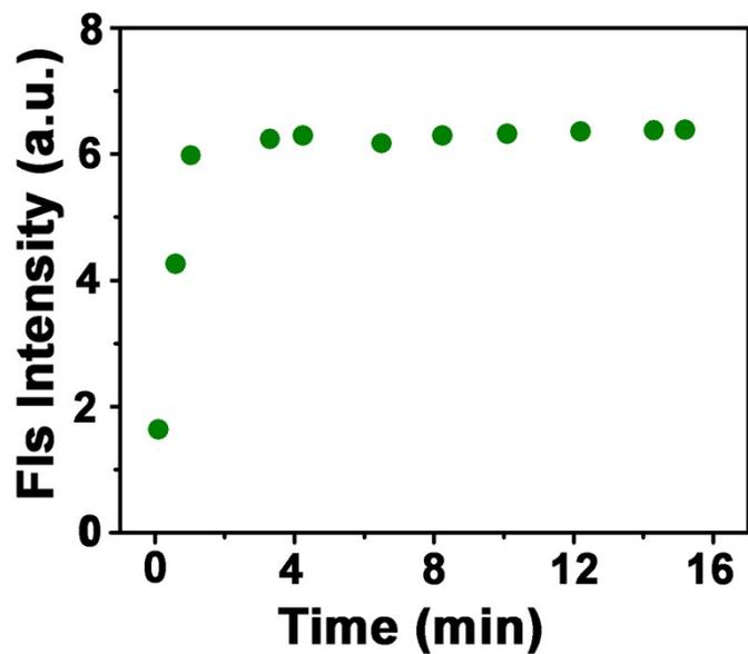
**Fig. S14** Time dependence of the fluorescence intensity of probe  $R-Zn^{2+}$  ( $5 \mu M$ ) in the presence of PPI ( $5 \mu M$ ) in  $0.02 M$  HEPES at  $pH = 7.8$ .
