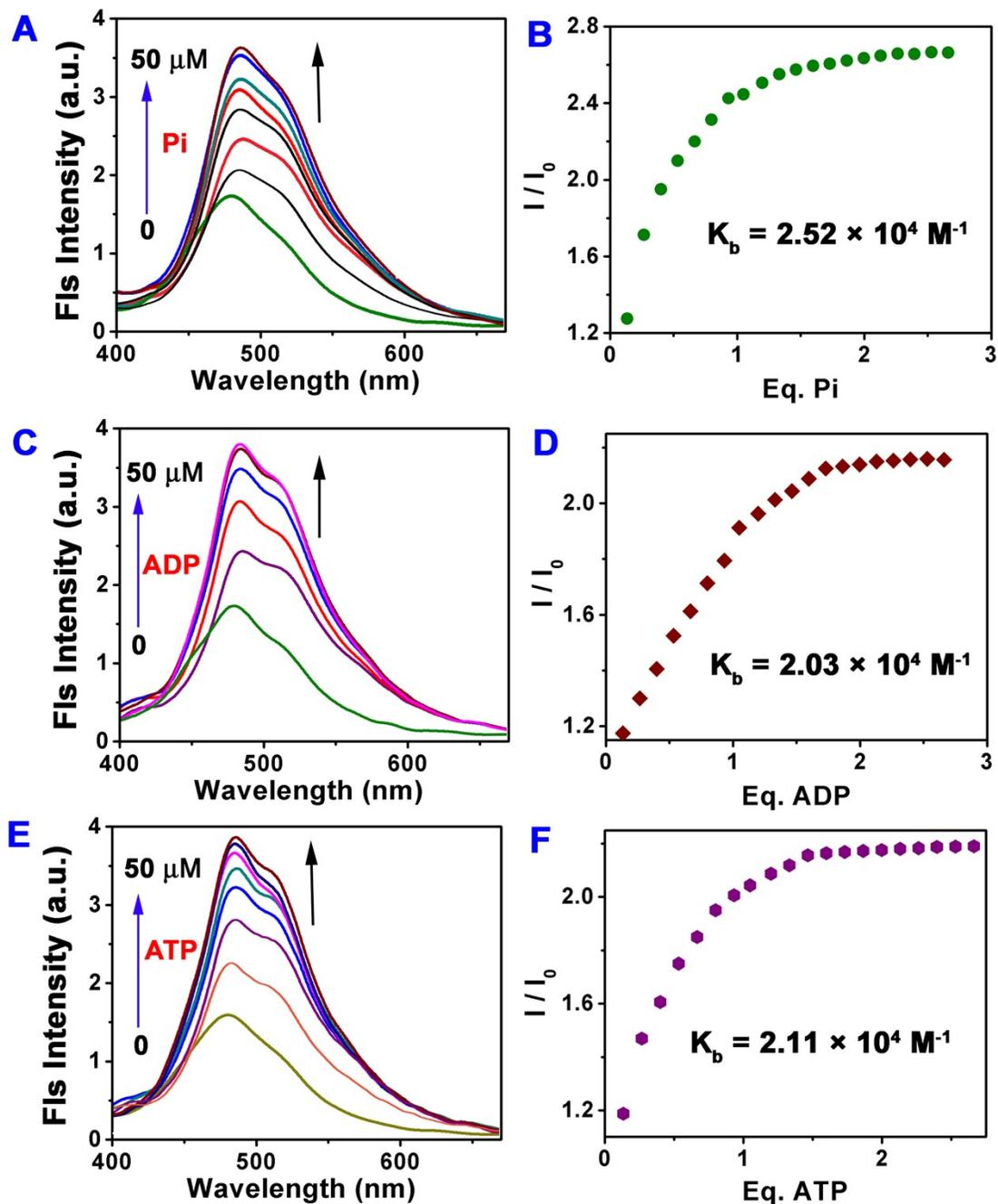
**Fig. S10** Change in the initial fluorescence intensities of probe **R-Zn<sup>2+</sup>** (5 μM) upon gradual increase in concentration of Pi (A), ADP (C) and ATP (E) (0–50 μM) in 0.02 M HEPES at pH = 7.8, and corresponding binding isotherms (B, D and F).
