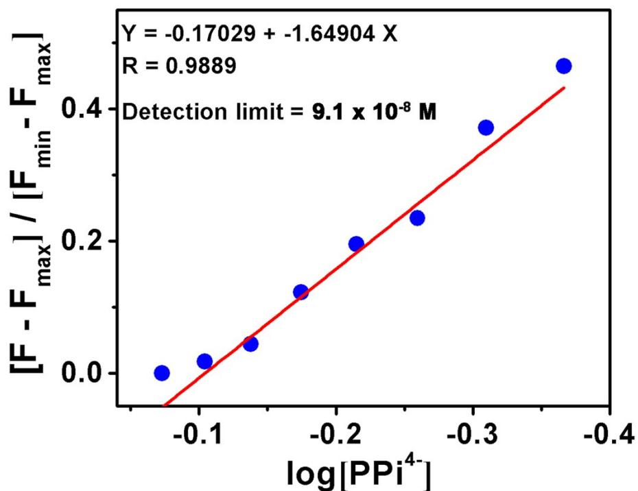
**Fig. S13** Detection limit plot of  $[(F - F_{\max}) / (F_{\min} - F_{\max})]$  against  $\log[\text{PPi}^{4-}]$  (concentration in nM) (D), where  $F_{\min}$ ,  $F$  and  $F_{\max}$  indicate the emission intensity in absence of, at intermediate and at infinite concentration of PPi, respectively.
