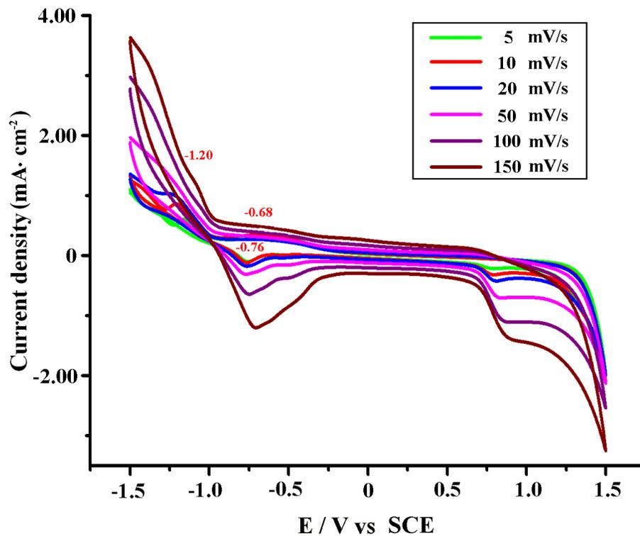
**Fig. S7** Cyclic voltammograms of **1-GCE (a)**, **L-GCE (b)**, **1,4-H<sub>2</sub>bdc-GCE (c)** and **2-GCE (d)** in a 0.05 M NaNO<sub>3</sub> aqueous solution (50 mL) at different sweep rates.
