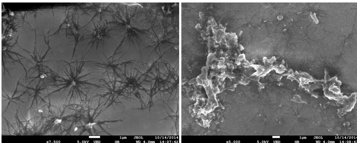
**Fig. S2** The SEM images of the separator membrane of MOF 1 before (**a, b**) and after the charge-discharge experiments (**c, d**). The SEM images of the separator membrane of MOF 2 before (**e, f**) and after the charge-discharge experiments (**g, h**).
