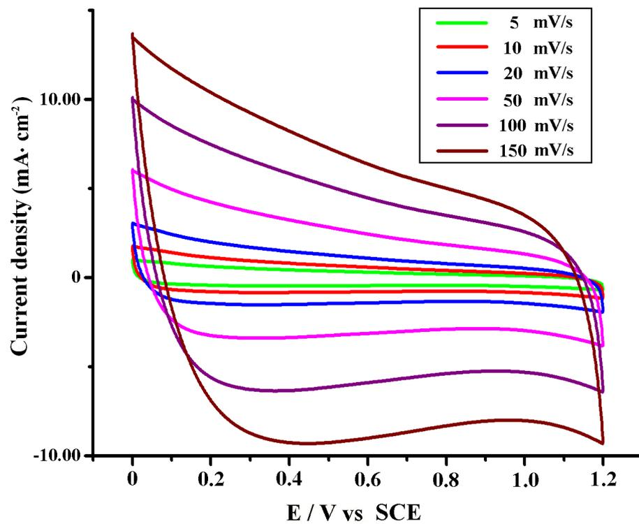
**Fig. S12** CVs of the supercapacitor in the presence of the separator membrane of **1a** at different sweep rates. Supporting electrolyte = 0.05 M  $\text{NaNO}_3$  aqueous solution.
