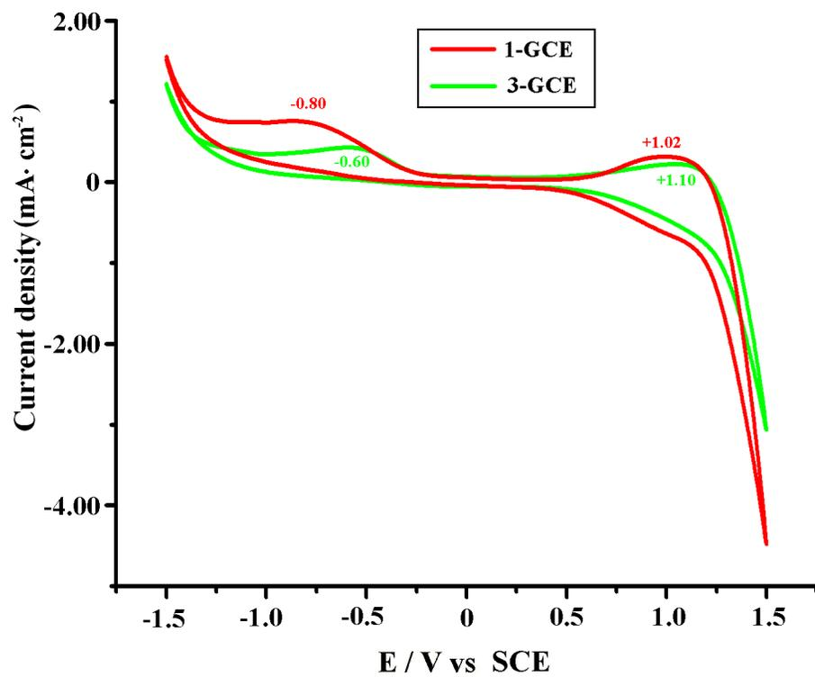
**Fig. S15** CVs of 1-GCE (red) and 3-GCE (green) in a 0.05 M NaNO<sub>3</sub> aqueous solution (50 mL) at a scan rate of 10 mV·s<sup>-1</sup>.
