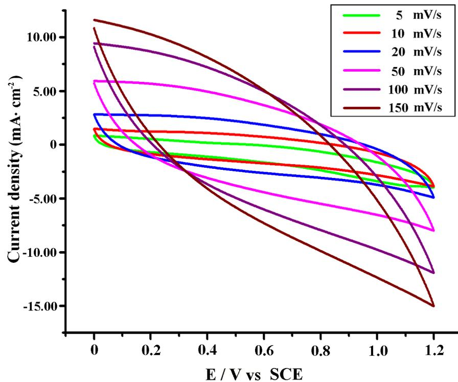
**Fig. S18** CVs of the supercapacitor in the presence of the separator membrane of **3b** at different sweep rates. Supporting electrolyte = 0.05 M NaNO<sub>3</sub> aqueous solution.
