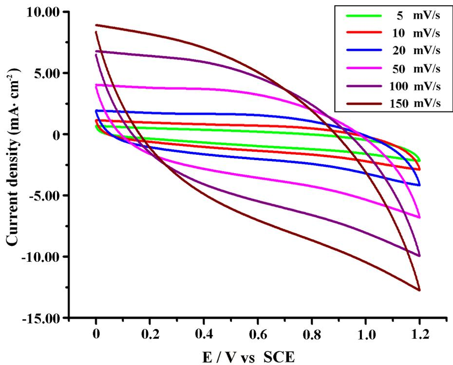
**Fig. S14** CVs of the supercapacitor in the presence of the separator membrane of **1a** at different sweep rates. Supporting electrolyte = 0.05 M phosphate buffer aqueous solution (pH 6.8, H<sub>3</sub>PO<sub>4</sub>/NaOH).
