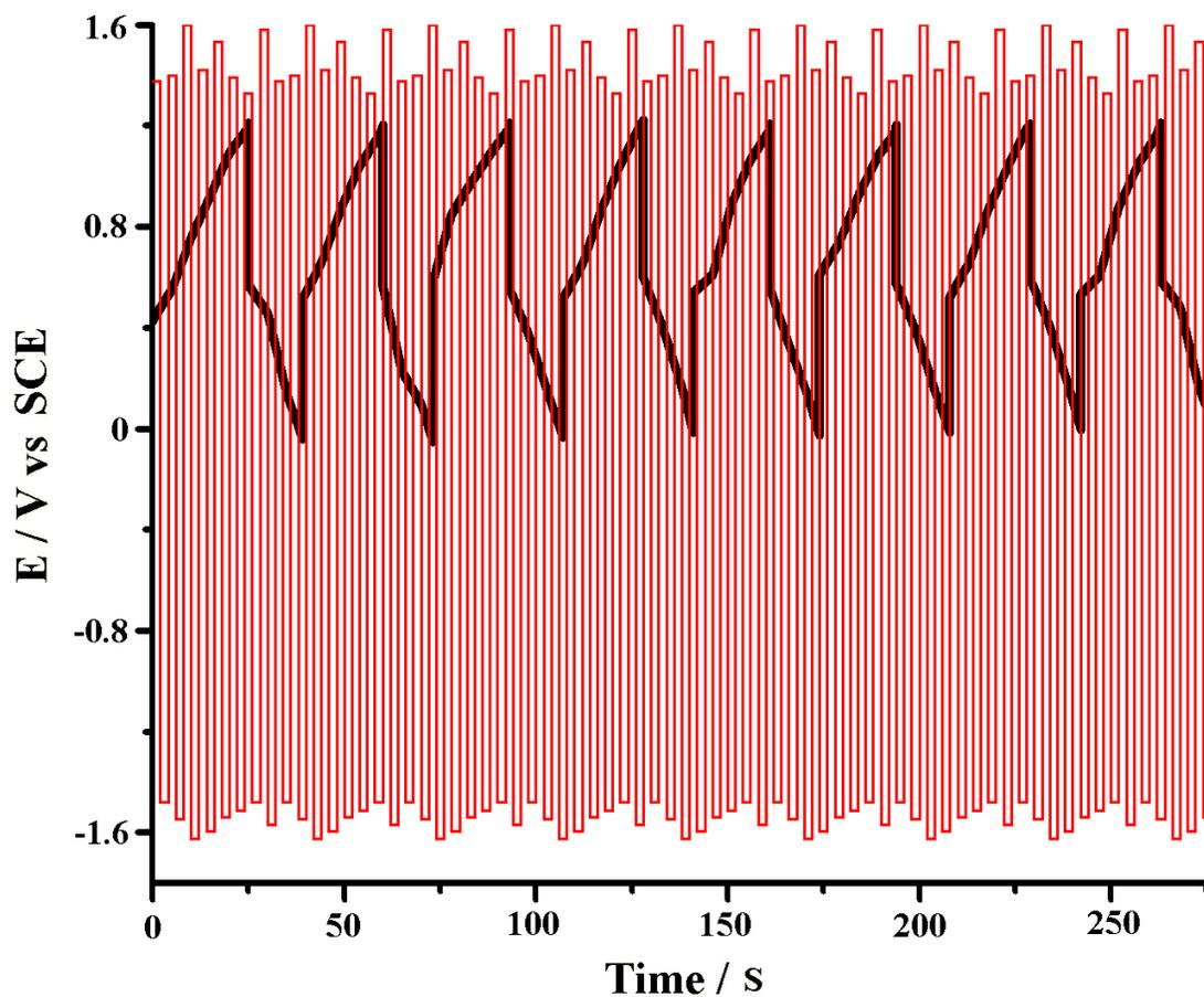
**Fig. S10** Typical charge-discharge cycles obtained in the presence (red) and absence (black) (c) of the separator membrane of MOF **1** at  $3.0 \text{ A}\cdot\text{g}^{-1}$  (a) and  $2.0 \text{ A}\cdot\text{g}^{-1}$  (b), respectively. Supporting electrolyte =  $0.05 \text{ M NaNO}_3$  aqueous solution.
