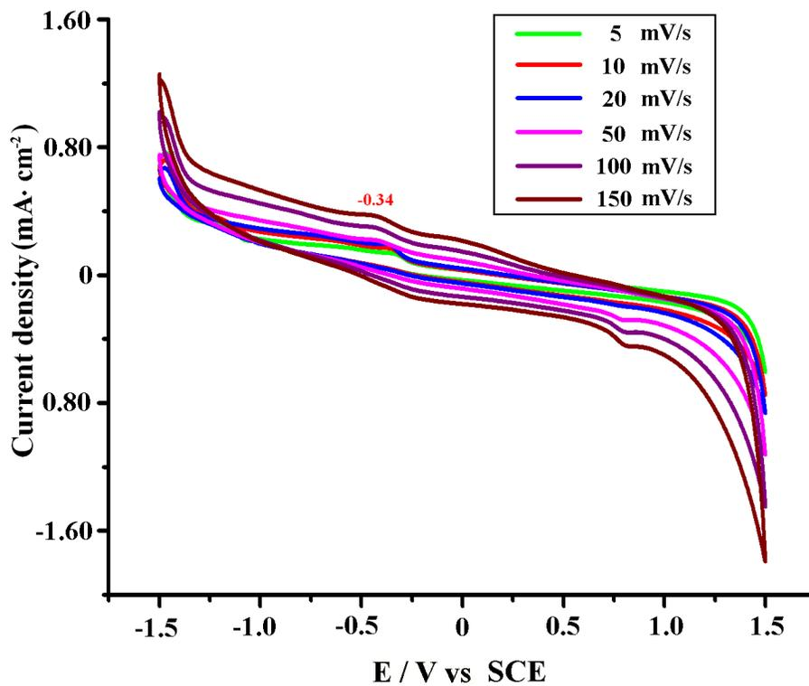
**Fig. S8** Cyclic voltammograms of the bare GCE in a 0.05 M NaNO<sub>3</sub> aqueous solution (50 mL) at different sweep rates.
