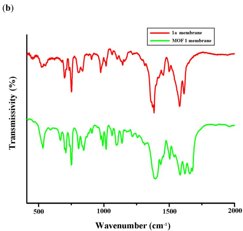
Fig. S13 The IR spectra of the separator membranes of **1a** and **1** in different scales (a, b).
