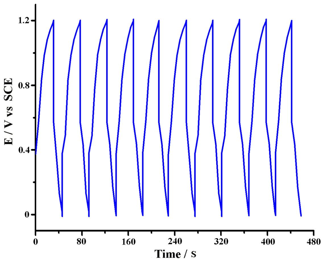
**Fig. S11** Typical charge-discharge cycles obtained in the presence of the separator membrane of MOF **2** at  $0.3 \text{ A}\cdot\text{g}^{-1}$  (**a**) and  $0.2 \text{ A}\cdot\text{g}^{-1}$  (**b**), respectively. Supporting electrolyte =  $0.05 \text{ M NaNO}_3$  aqueous solution.
