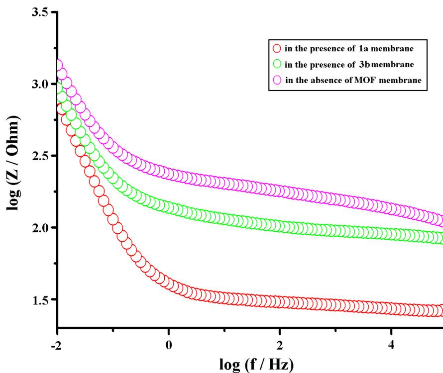
**Fig. S19** Bode plots (log of impedance magnitude vs. log f) the supercapacitors at the initial potential of 0 V in the absence and presence of the separator membrane of MOF **1a** and **3b**. Supporting electrolyte = 0.05 M NaNO<sub>3</sub> aqueous solution.
