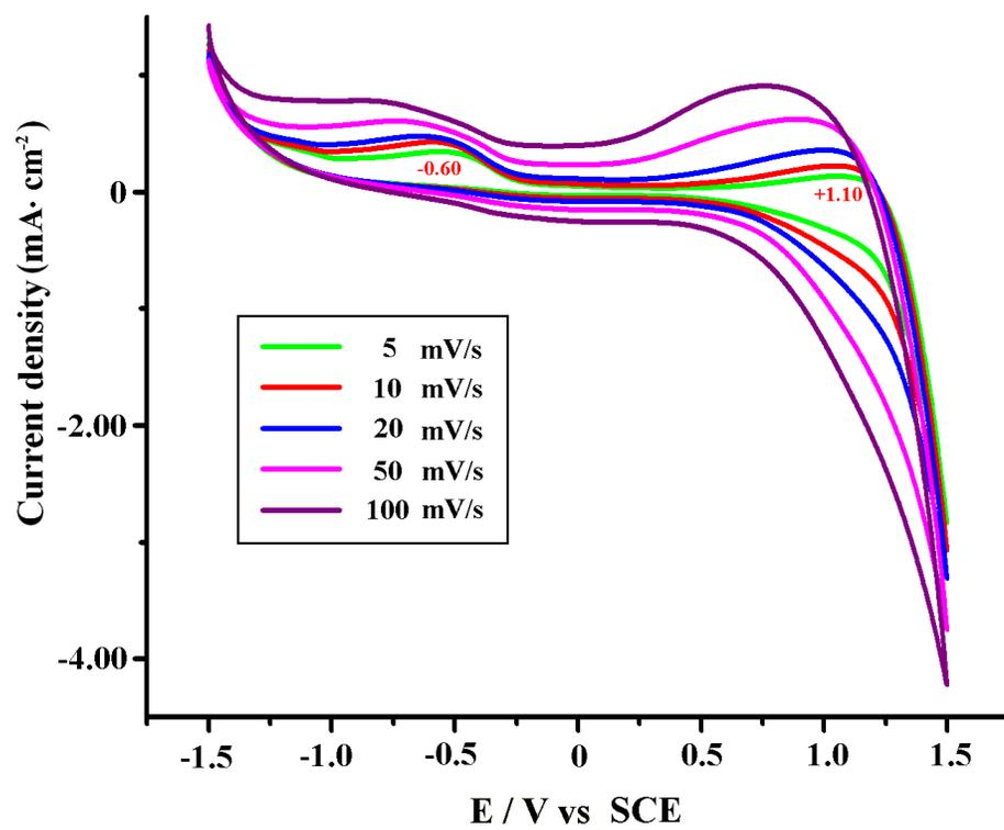
**Fig. S16** Cyclic voltammograms of **3-GCE** in a 0.05 M NaNO<sub>3</sub> aqueous solution (50 mL) at different sweep rates.
