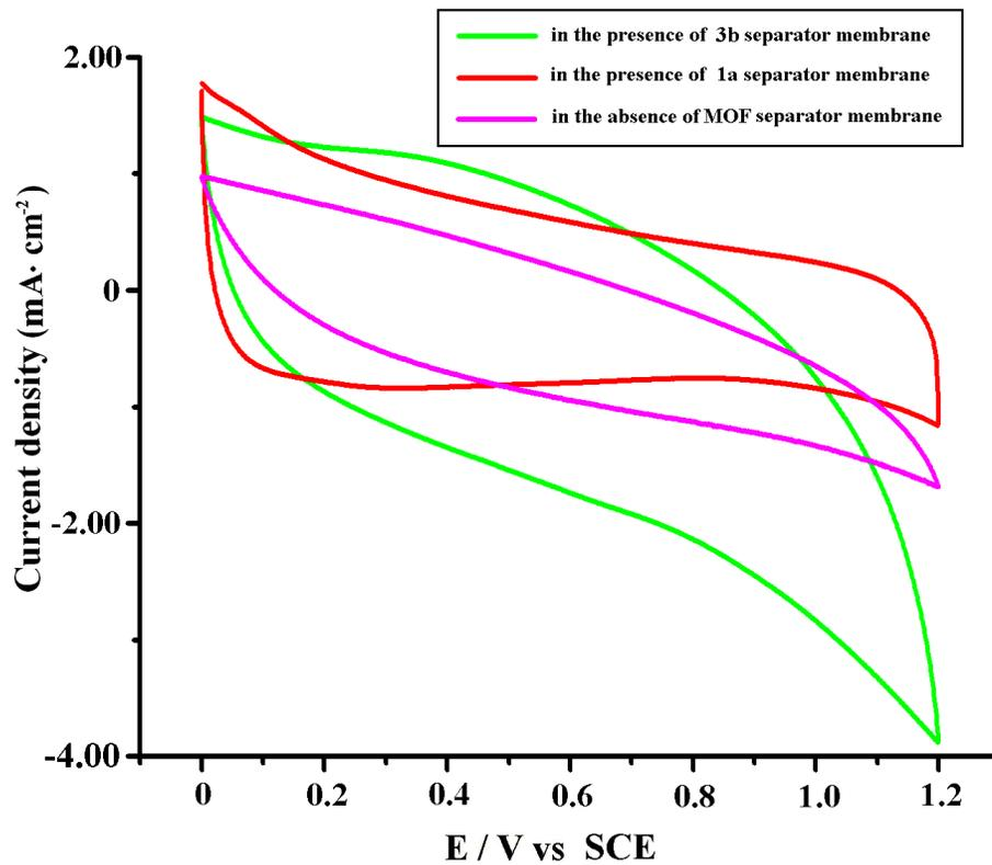
**Fig. S17** CVs of the supercapacitors in the absence and presence of the separator membrane of **1a** and **3b** at a scan rate of 10 mV·s<sup>-1</sup>. Supporting electrolyte = 0.05 M NaNO<sub>3</sub> aqueous solution.
