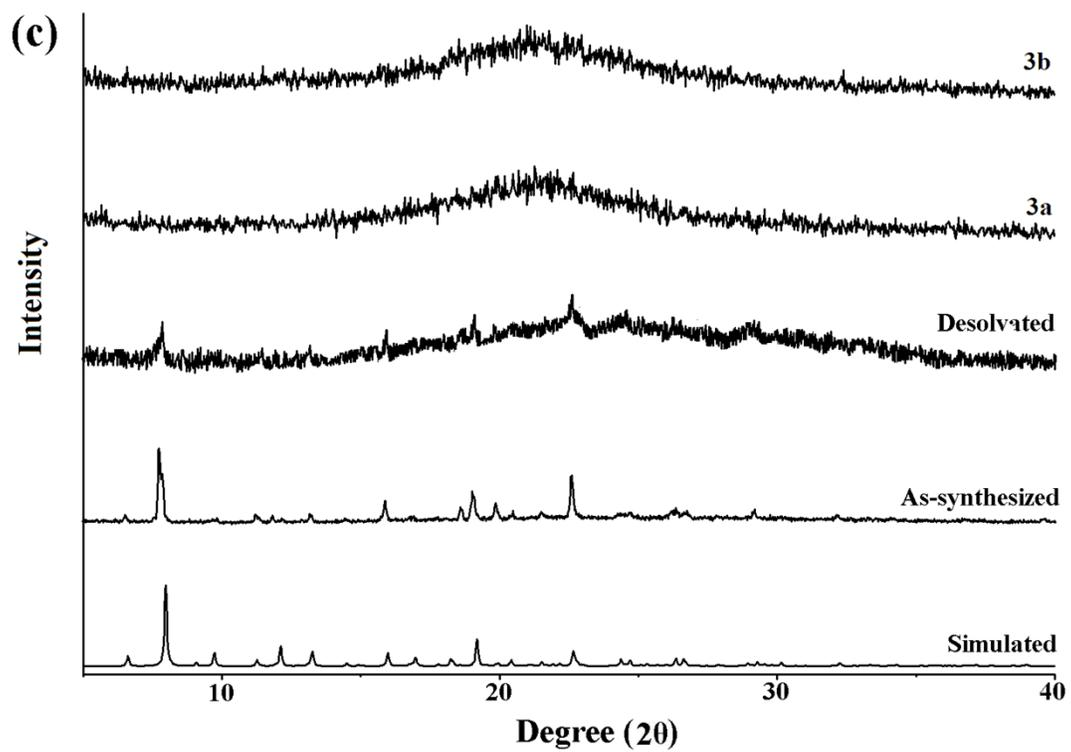
**Fig. S6** The PXRD patterns of MOFs **1** (a), **2** (b) and **3** (c).
