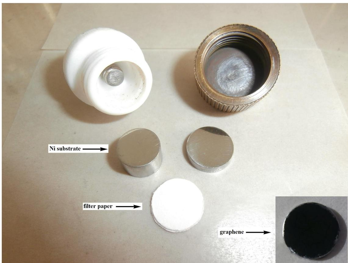
**Fig. S3** The images of the supercapacitor, in which two Ni substrates were used as current collectors, and each piece of the collector was covered by 0.25 mg graphene as electrode material. The separator membrane of MOF was sandwiched by two pieces of filter papers with two drops of the  $\text{NaNO}_3$  aqueous solution on each side as the electrolyte.
