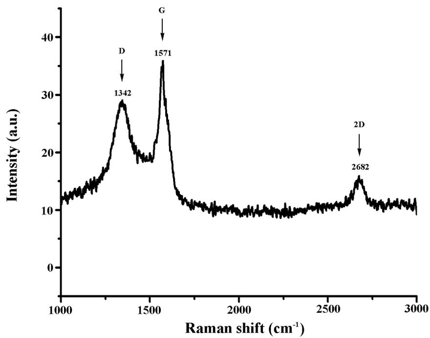
**Fig. S4** The image (a) and the Raman spectra (b) ( $\lambda_{\text{ex}} = 514.5 \text{ nm}$ ,  $0.4 \text{ mW}$ ) of the graphene in supercapacitor.
