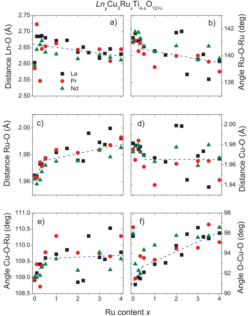
**Figure 3.** Structural data of  $Ln_y Cu_3 Ru_x Ti_{4-x} O_{12+\delta}$ . a)  $Ln\text{-O}$  distances, b)  $Ru\text{-O}\text{-Ru}$  angles, c)  $Ru\text{-O}$  bond lengths, d)  $Cu\text{-O}$  bond lengths, e)  $Cu\text{-O}\text{-Ru}$  angles, and f)  $O\text{-Cu}\text{-O}$  angles. Dashed blue lines are drawn to guide the eye.
