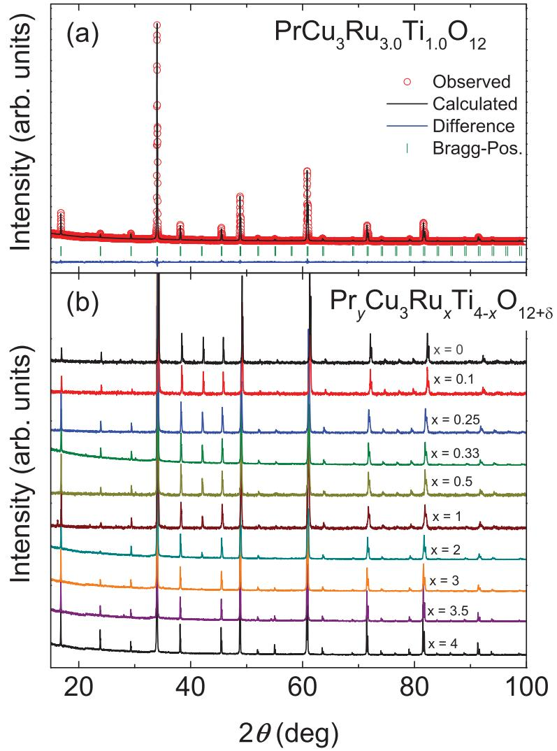
**Figure 1.** (a) Representative Rietveld-refinement of the x-ray diffraction pattern of  $\text{PrCu}_3\text{Ru}_{3.0}\text{Ti}_{1.0}\text{O}_{12}$  measured at room temperature. (b) X-ray diffraction patterns of  $\text{Pr}_y\text{Cu}_3\text{Ru}_x\text{Ti}_{4-x}\text{O}_{12+\delta}$  for different Ru contents  $x$ , normalized to the intensity of (2 2 0).
