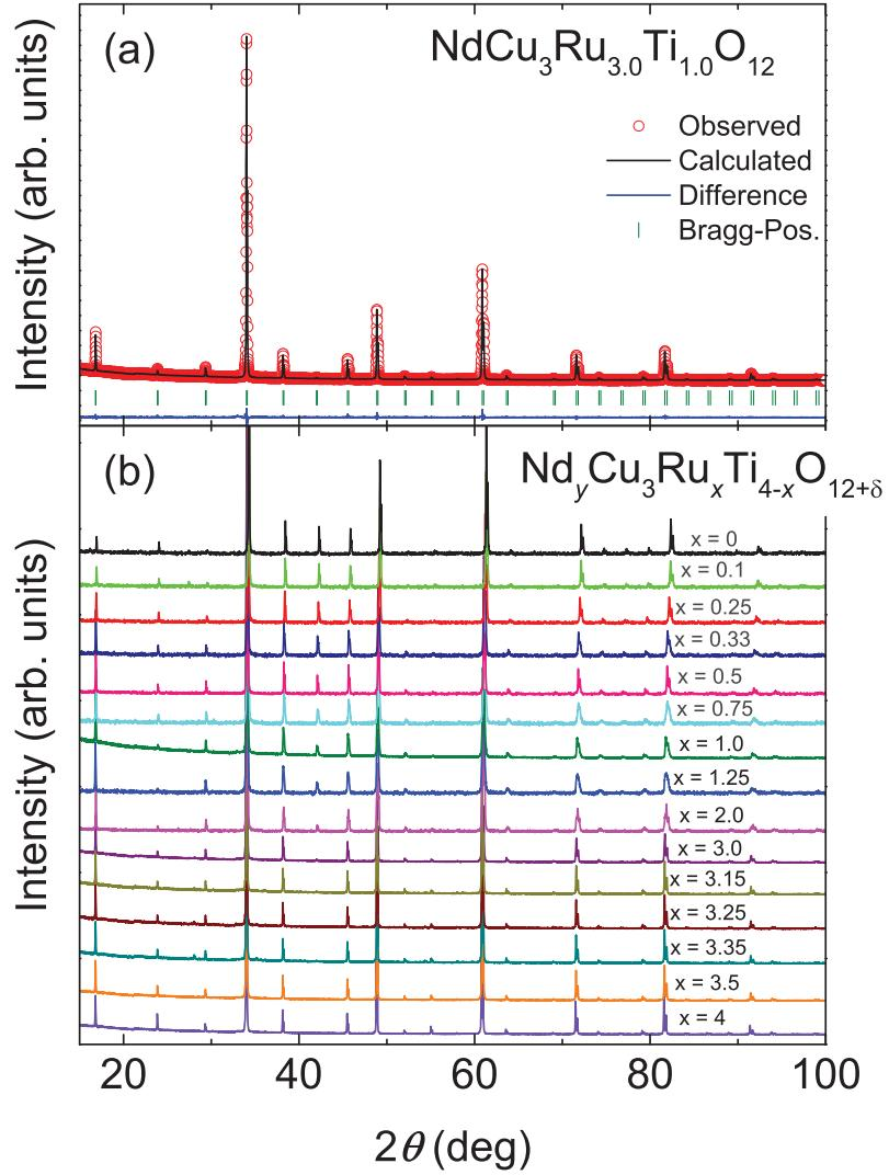
**Figure 2.** (a) Representative Rietveld-refinement of the x-ray diffraction pattern of  $\text{NdCu}_3\text{Ru}_{3.0}\text{Ti}_{1.0}\text{O}_{12}$  measured at room temperature. (b) X-ray diffraction patterns of  $\text{Nd}_y\text{Cu}_3\text{Ru}_x\text{Ti}_{4-x}\text{O}_{12+\delta}$  for different Ru contents  $x$ , normalized to the intensity of (2 2 0).
