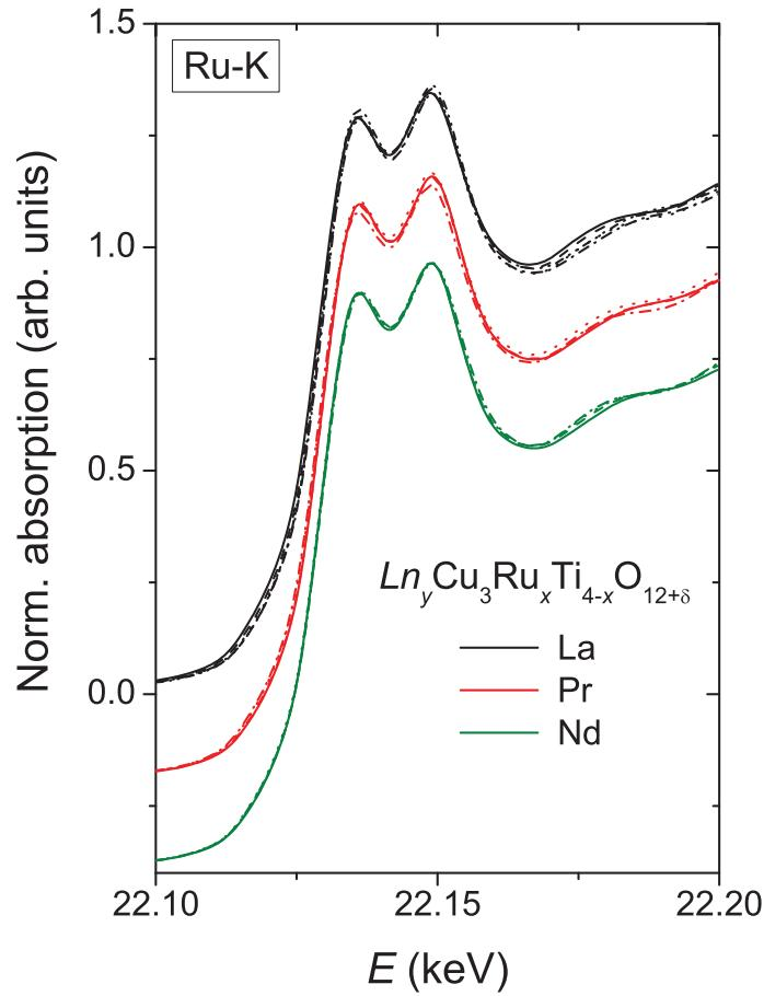
**Figure 4.** Ru-K edge XANES spectra of  $Ln_yCu_3Ru_xTi_{4-x}O_{12+\delta}$  for the three investigated  $A$ -site rare-earth elements: La (top), Pr (center), Nd (bottom). The spectra are grouped for each element and each group is shifted by a constant value to increase clarity.
