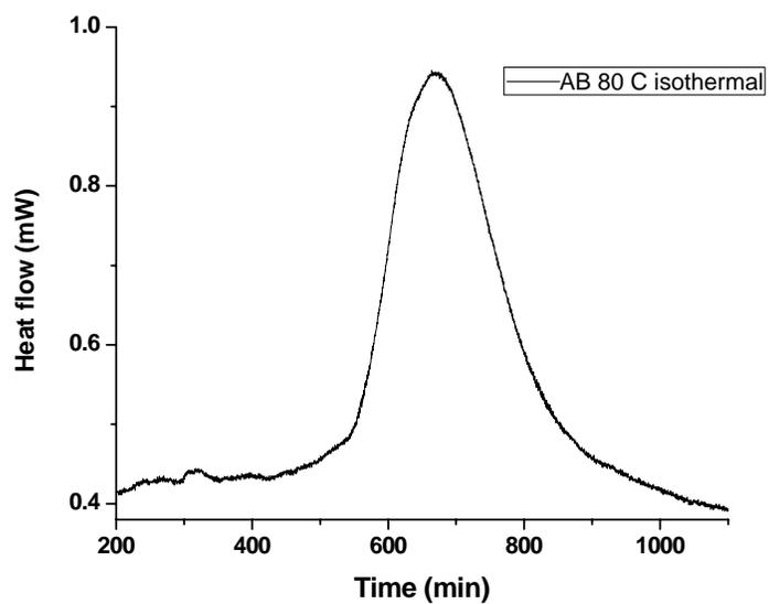
Figure 4S. Isothermal DSC for Ammonia borane at 80 °C.
