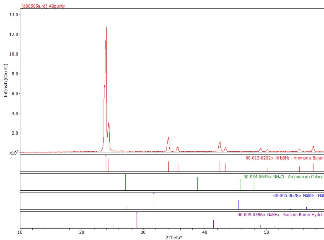
Figure 3S. XRD of synthesized AB
