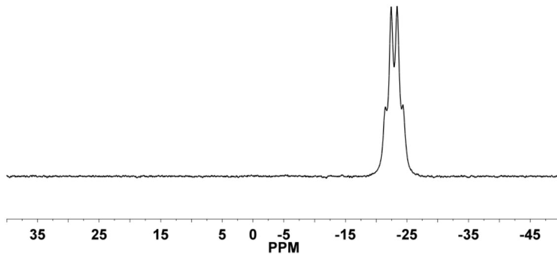
Figure 2S.  $^{11}\text{B}$  NMR (7 Tesla Boron) of synthesized AB in MeCN. Ref to  $\text{BF}_3:\text{OEt}_2$ , 0 ppm.  $J_{\text{B-H}} = 94$  Hz.
