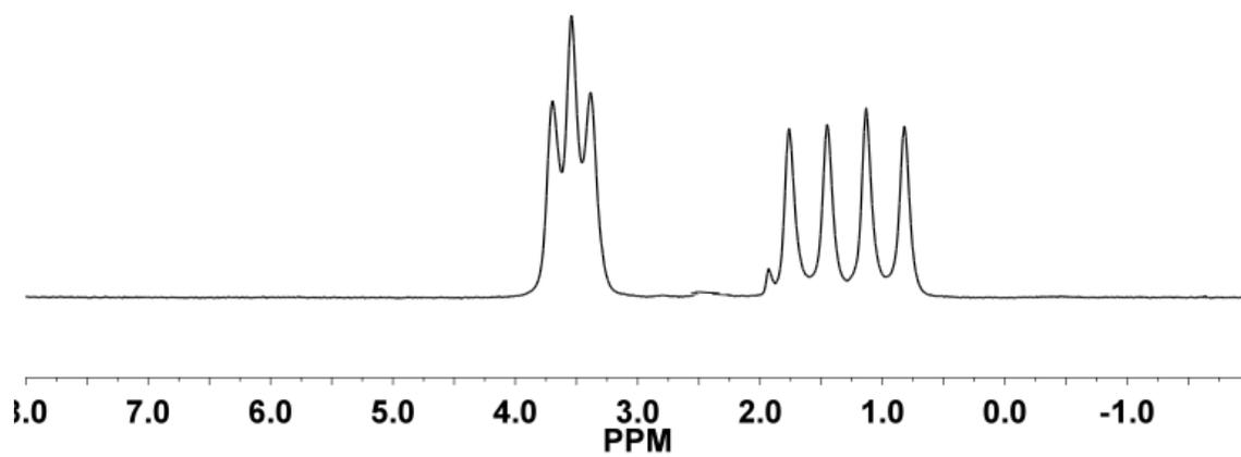
Figure 1S. <sup>1</sup>H NMR (300 MHz) of synthesized AB in *d*-MeCN. Ref. to MeCN, 1.94 ppm.  $J_{B-H} = 94$  Hz,  $J_{N-H} = 45$  Hz.
