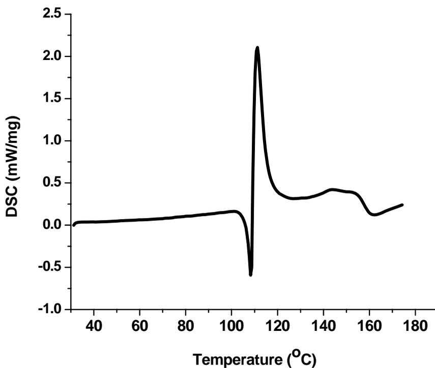
Figure 5S. Ramp DSC experiment for Ammonia borane at 30-180 °C.
