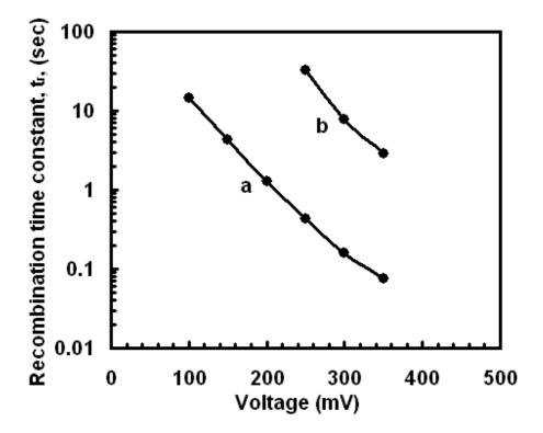
Supplimentary Figure: The electron lifetimes in (a) SnO<sub>2</sub> nanoparticles and (b) SnO<sub>2</sub> nanowires.
