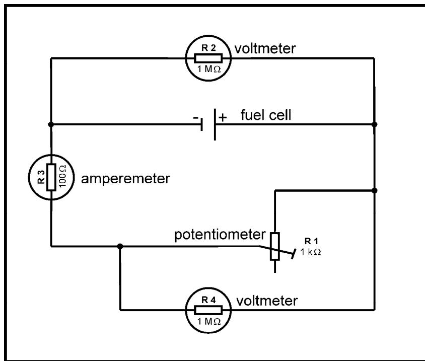
Scheme of the experimental setup: Internal resistances of the instruments are indicated in the scheme below the resistance symbols. The potentiometer represents the load resistance which can be varied between 0 and 1 kΩ. The current, the cell potential and the voltage at the adjustable resistance were recorded during the measurements. The performance curves given refer to the potential at the potentiometer and the overall current in the circuit.
