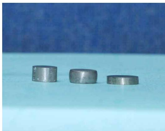
**Figure S2.** Photographs of the Bi<sub>0.5</sub>Sb<sub>1.5</sub>Te<sub>3</sub> samples: ‘initial  $\phi$  10 mm disk, the deformed sample, and the final  $\phi$  12.7 mm disk’ from left to right, indicating that the sample continuously deformed during hot press.
