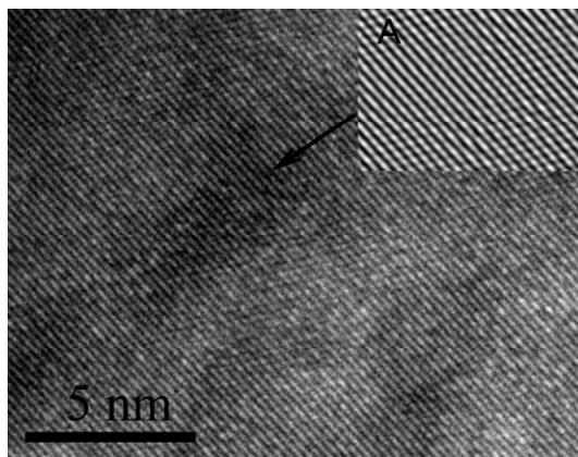
**Figure S1.** HRTEM image of the initial hot pressed sample without hot forging.
