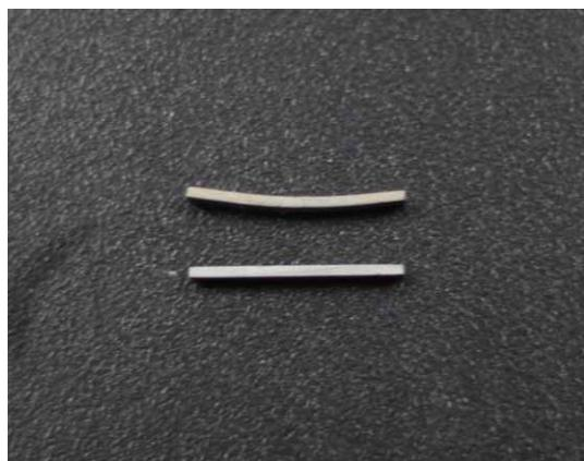
**Figure S3.** Photograph of the Bi<sub>0.5</sub>Sb<sub>1.5</sub>Te<sub>3</sub> bars before and after simple three-point bending test from room temperature to 573K at a load of 5N.
