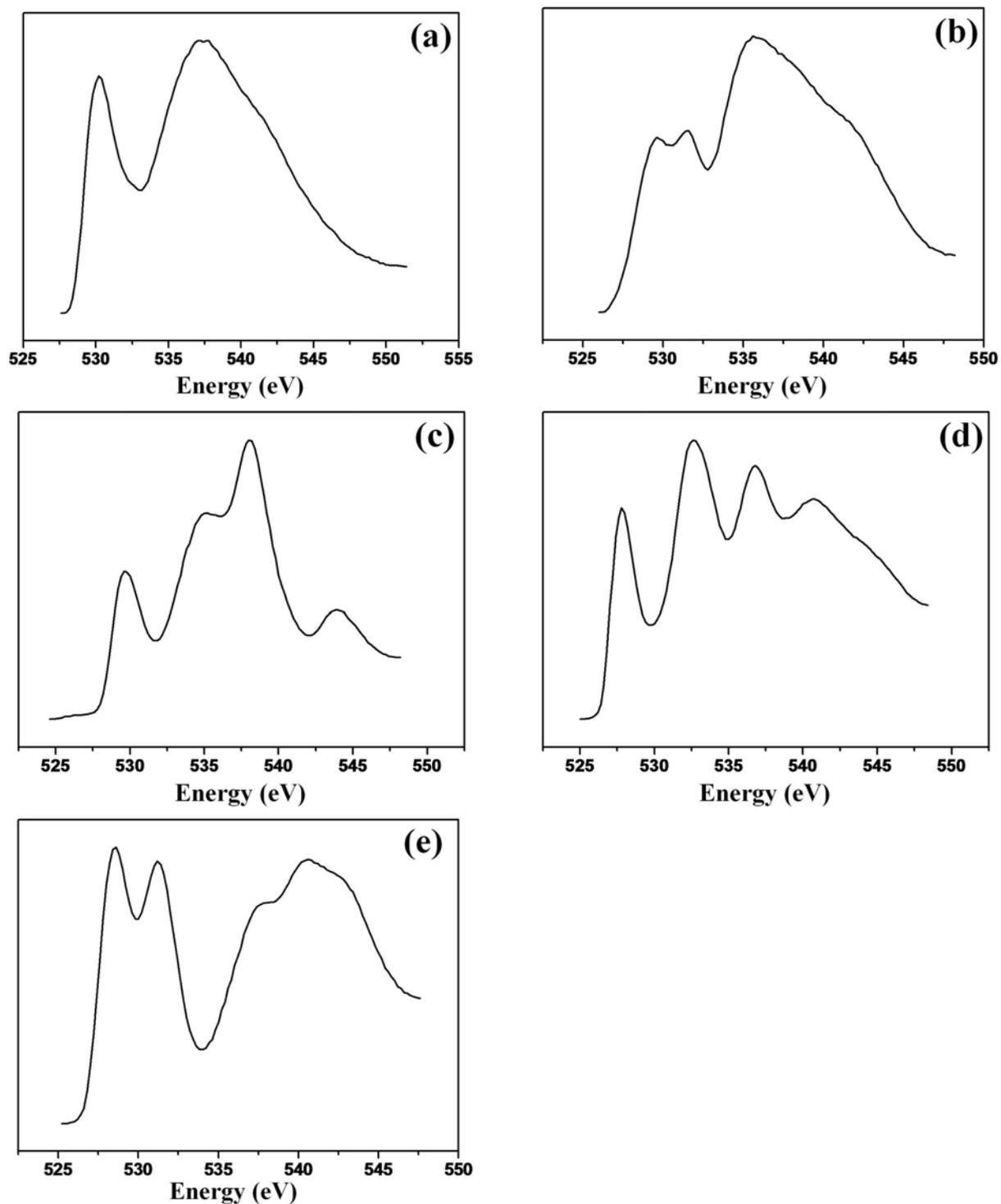
The oxygen K-edge Near Edge X-ray Absorption Fine Structure (NEXAFS) data were collected by Pohang accelerator in Pohang, Republic of Korea. There are clear differences between the data of LDHs and the data of the pure oxides. Therefore, we find that the bonding nature of oxygen in LDHs is not same with the pure oxides. It assists that the synthesized LDHs consist of the  $M^{II}$ -O-Ti<sup>4+</sup> bonding.
