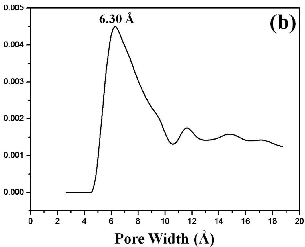
The pore distribution of the two materials is calculated by HK method based on low temperature N<sub>2</sub> sorption hysteresis (Fig. 5). The peak is located at 6.67 Å for (Ni/Ti)LDH and 6.30 Å for (Cu/Ti) LDH. These values are similar to the values by calculated from (003) peak of powder x-ray diffraction pattern (Fig. 2).
