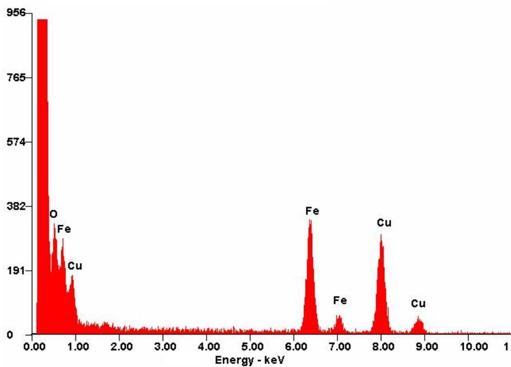
Figure S2. EDS spectrum of ultrathin single crystal lepidocrocite nanosheets.
