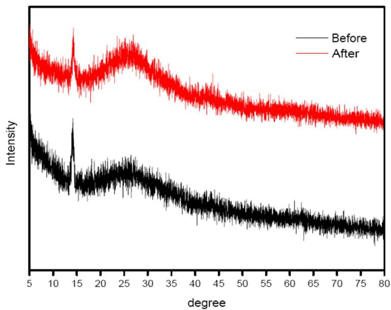
Figure S6. XRD patterns of Fe-G 20% before and after phenol treatment.
