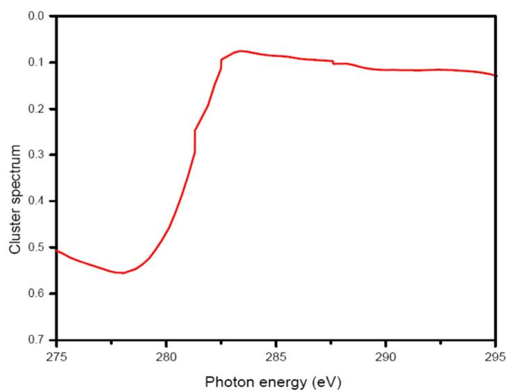
Figure S4. NEXAFS spectrum of reduced graphene oxide in Fe-G 20% nanocomplex.
