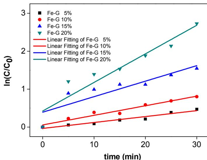
Figure S5. Data fitting with the first-rate reaction kinetics for phenol degradation with Fe-G nanostructures of different Fe contents (shown in Fig. 5e).
