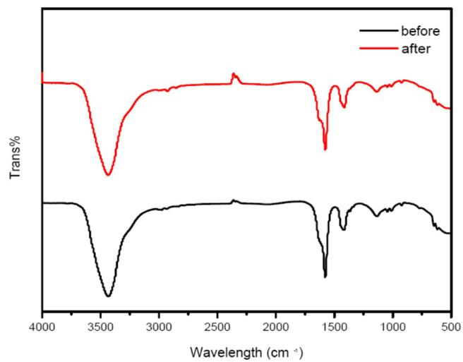
Figure S7. FTIR spectra of Fe-G 20% before and after phenol treatment.
