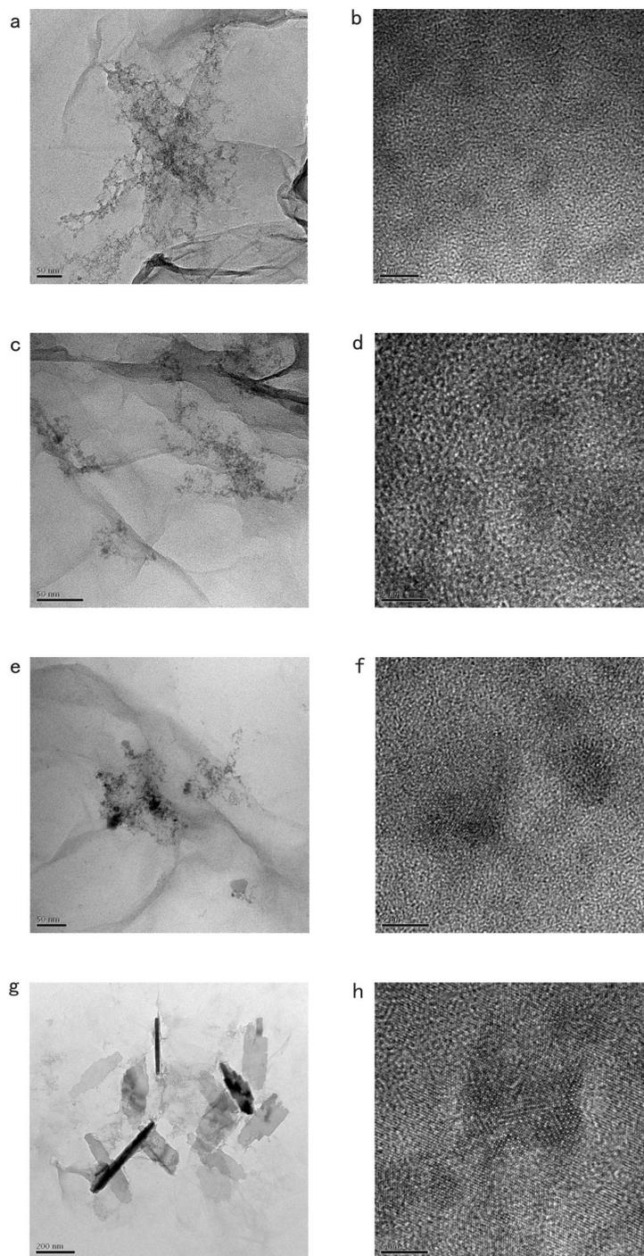
Figure S1. TEM and HRTEM imaging of ultrathin single crystal lepidocrocite nanosheets. a, TEM image of Fe-G 5%. b, HRTEM image of Fe-G 5%. c, TEM image of Fe-G 10%. d, HRTEM image of Fe-G 10%. e, TEM image of Fe-G 15%. f, HRTEM image of Fe-G 5%. g, TEM image of Fe-G 20%. h, HRTEM image of Fe-G 20%.
