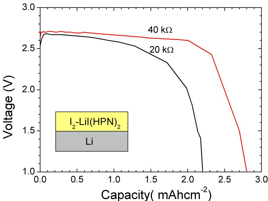
**Figure S4.** The discharging curves of an Li/I<sub>2</sub>-LiI(HPN)<sub>2</sub> battery using a 20 kΩ and 40 kΩ loading.
