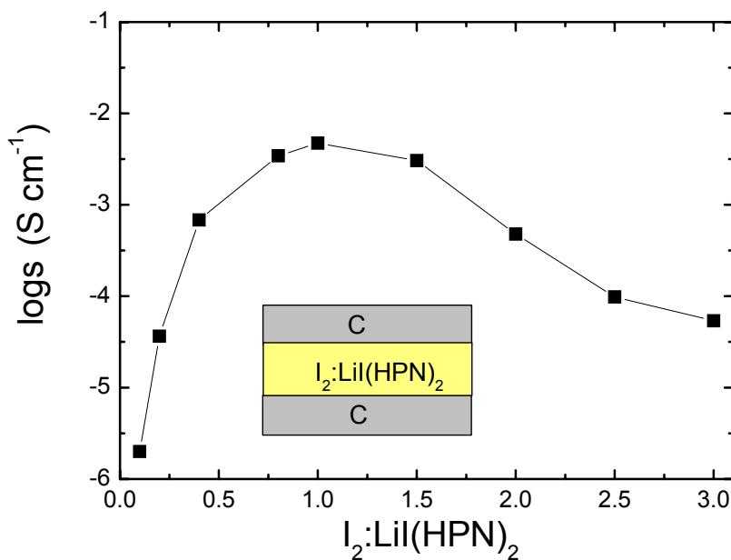
**Figure S5** Conductivity of a complex mixture of iodine and  $\text{LiI}(\text{HPN})_2$  with different molar ratio of  $\text{I}_2/\text{LiI}(\text{HPN})_2$ .
