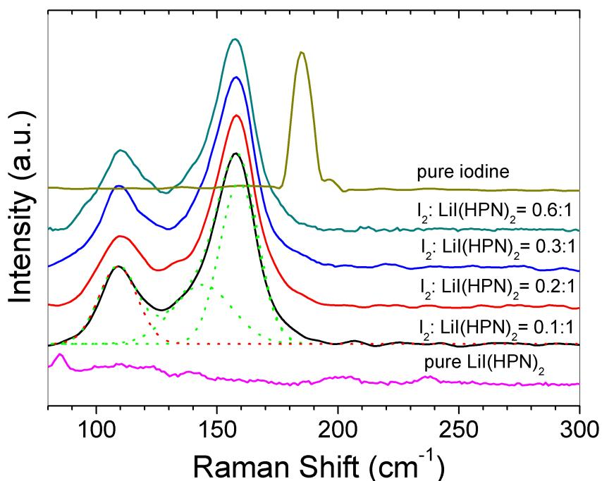
**Figure S3** Raman spectra of the pure iodine, pure electrolyte LiI(HPN)<sub>2</sub> and a complex mixture of iodine and LiI(HPN)<sub>2</sub> with different molar ratio of I<sub>2</sub>/LiI(HPN)<sub>2</sub>.
