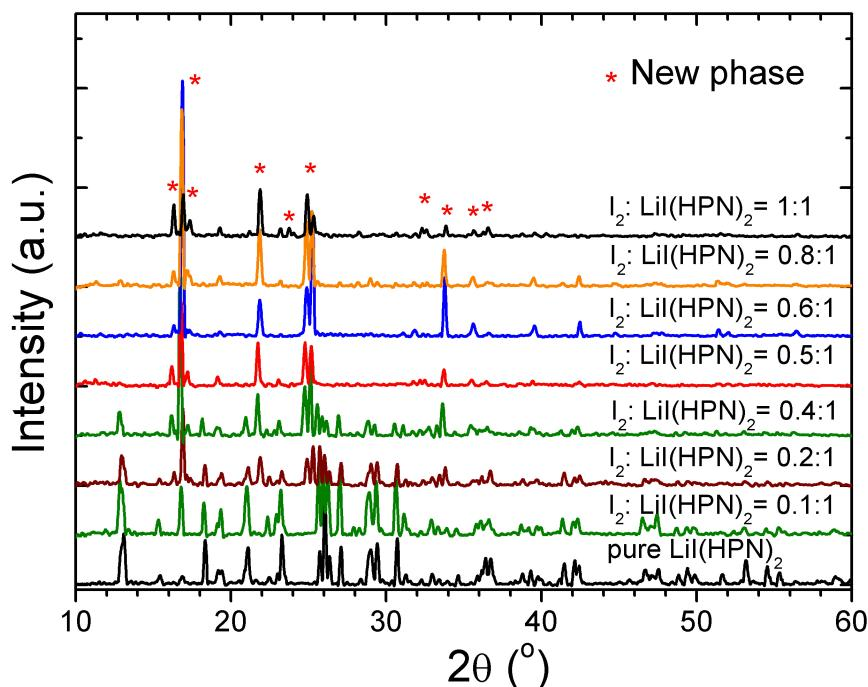
**Figure S2** XRD patterns of a complex mixture of iodine and  $LiI(HPN)_2$  with different molar ratio of  $I_2/LiI(HPN)_2$ . XRD pattern of the pure electrolyte  $LiI(HPN)_2$  is included for comparison.
