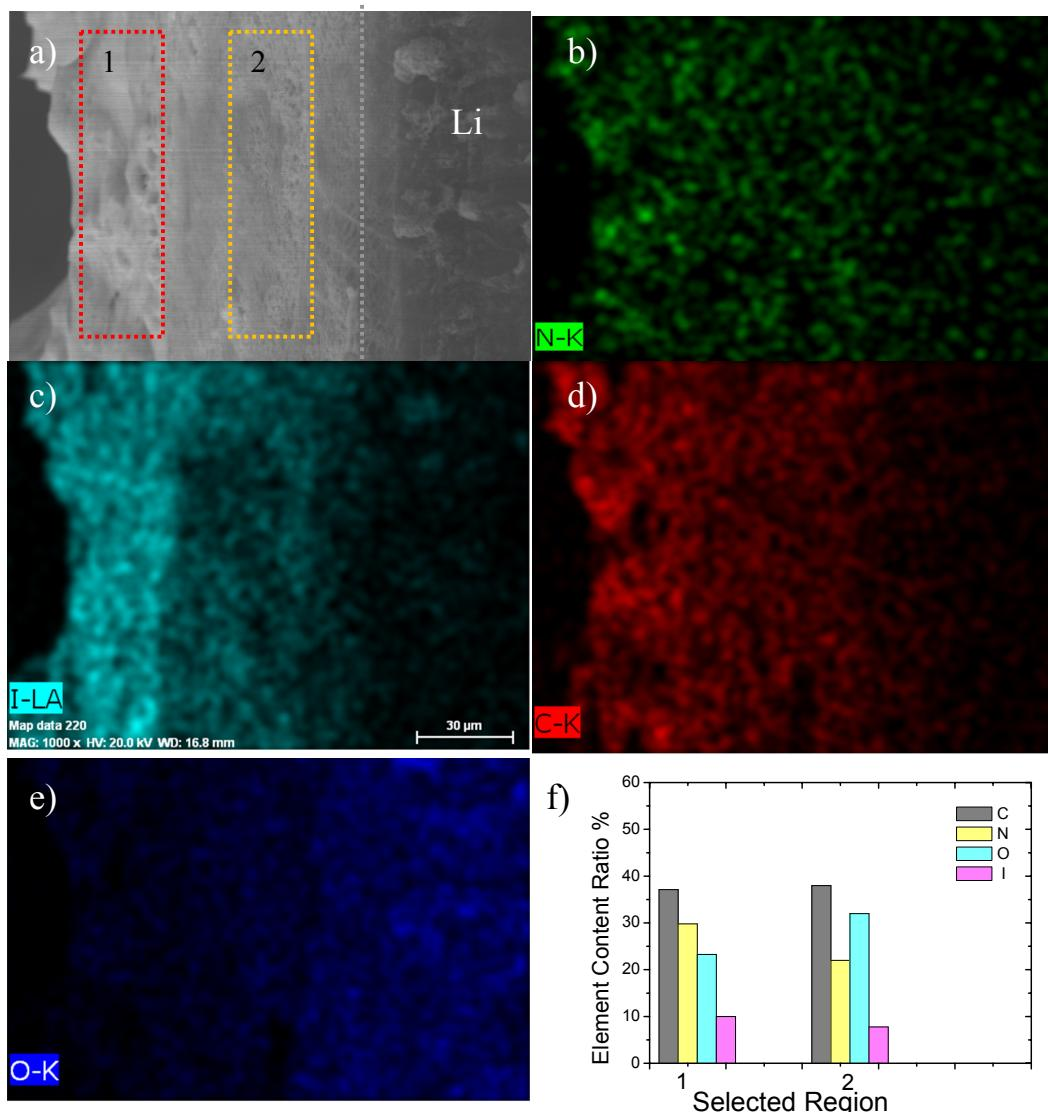
**Figure S1.** a) Cross-sectional backscattered electron images of Li/LiI(HPN)<sub>2</sub>/ LiI(HPN)<sub>2</sub>-I<sub>2</sub> cell, and the corresponding energy-dispersive X-ray spectrometry mappings of b) N; c) I; d) C and (e) O; (f) the average molar concentration ratio of I/C/N/O from corresponding EDX spectra in two selected regions( 1 and 2).
