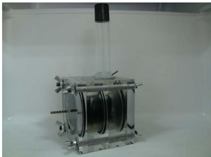
**Figure S1.** Single-chamber MEC shown with gas collection tube (top).
