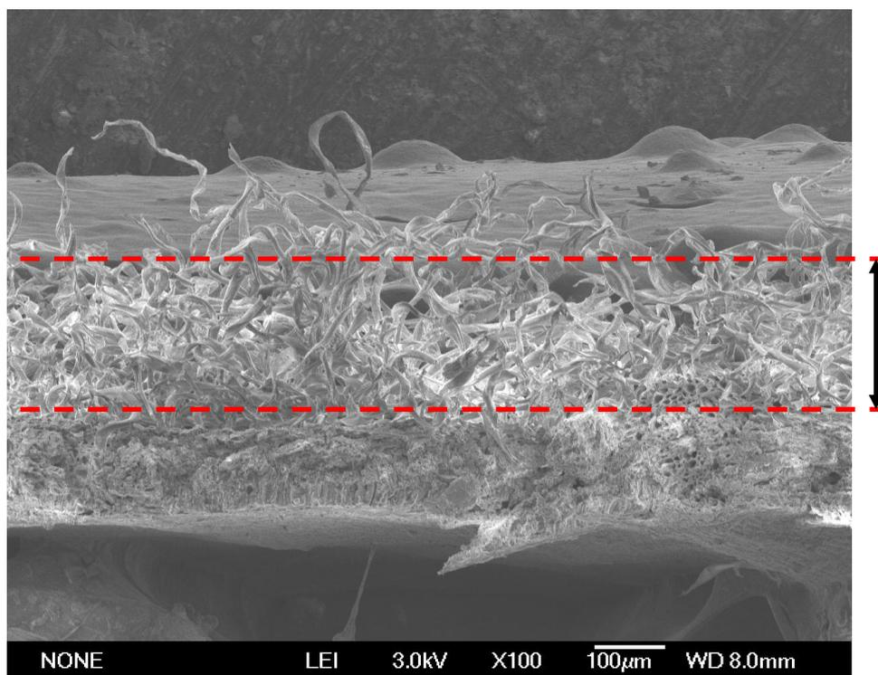
**Fig. S1** SEM image of the cross section of the leaf. The thickness of the hairs layer is approximately 200 µm.
