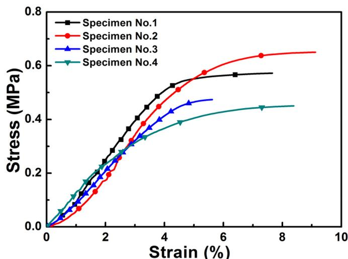
**Fig. S9** The typical stress-strain curves of PSt fibrous films. The PSt fibrous films were cut into 7 mm wide and 40 mm long strips for tensile tests. The mechanical properties were performed on a dynamic mechanical analysis machine (DMA Q800, TA instrument Inc.), using the controlled-force mode with a speed of 0.01 N/min and gauge length of 10 mm under room temperature.
