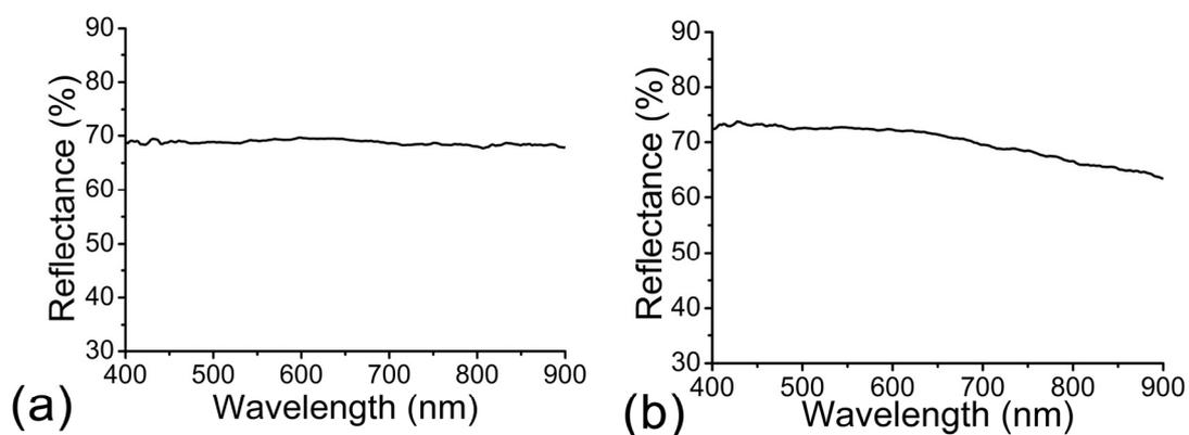
**Fig. S8** Two common polymers are also suitable for such a mimic fabrication of the fibrous films: (a) poly- vinylpyrrolidone (PVP); (b) poly(vinylidene fluoride) (PVDF). The size of the prepared fibrous films is around 16  $\mu\text{m}$  in fiber width and 400-450  $\mu\text{m}$
