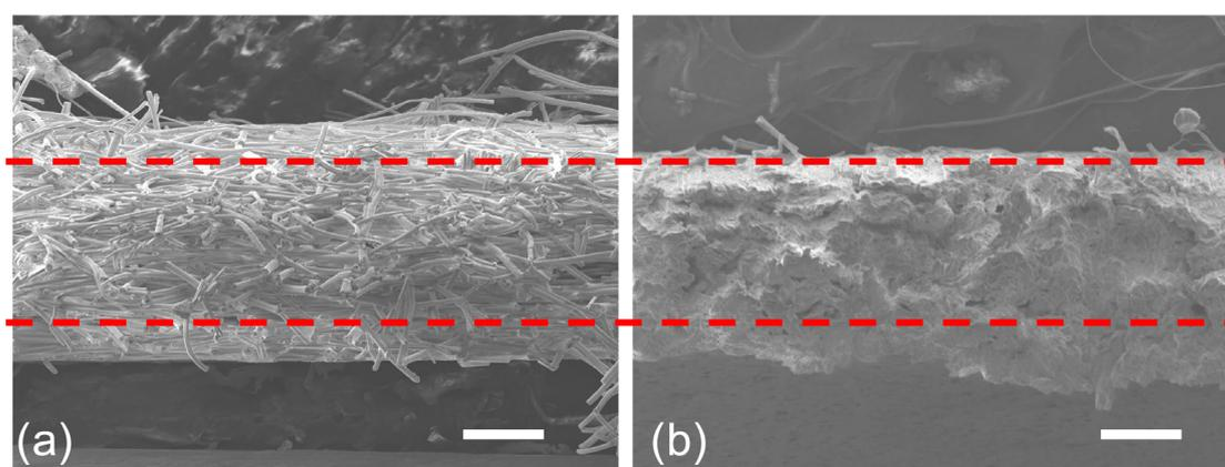
**Fig. S7** (a) The cross-section of the fibrous film.(b) The cross-section of the control film. They have similar thickness around 400  $\mu\text{m}$ . Bars: 100  $\mu\text{m}$
