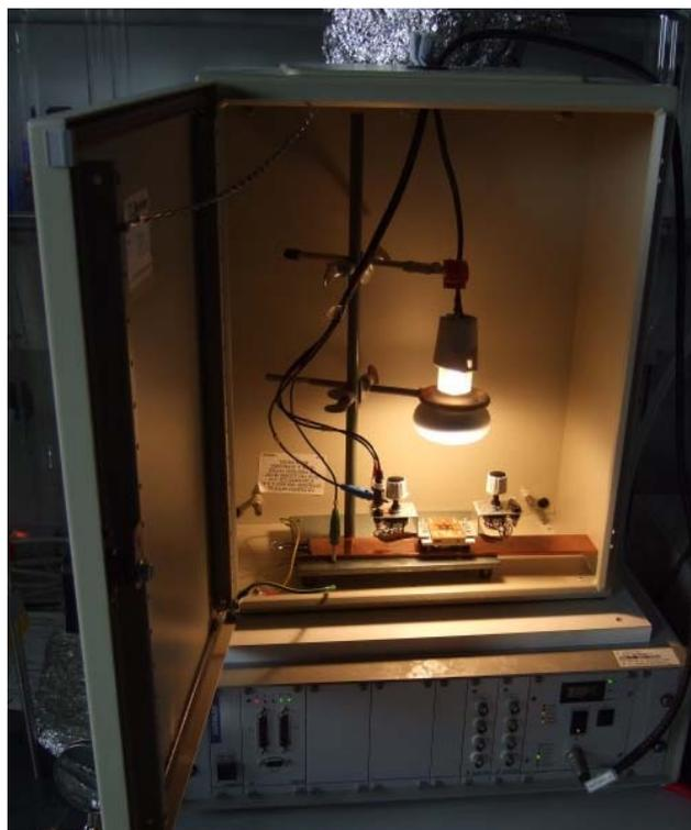
**Figure S2.** Setup for measuring the I-V characteristics under our standard indoor illumination conditions with a 60 W incandescent lamp (having a reflecting backside coating) from 10 cm distance.
