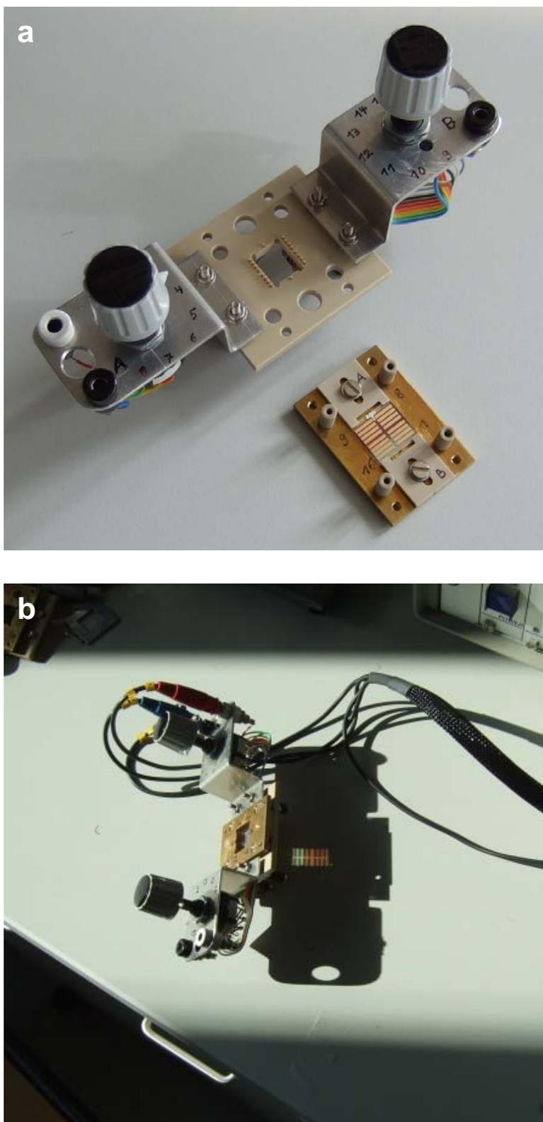
**Figure S1.** Pictures of the home built mounting (contacting) device for the I-V measurements of ss-DSSCs and DASCs, a) before contacting the reference ss-DSSC partly coated with a  $\text{TiO}_2$  layer of 13 nm sized particles and sensitized by the ruthenium dye N719, b) ready contacted and illuminated from the FTO side by natural sunlight.
