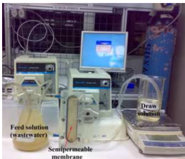
Figure S2. Laboratory setup for the forward osmosis process. Peristaltic pumps are used to circulate the feed and draw solutions which are separated by the flat-sheet semipermeable FO membrane (cellulose triacetate). Fresh water naturally diffuses from the feed solution (wastewater) to the draw solution ( \text{Al}_2(\text{SO}_4)_3 ) in a forward osmosis mode without intensive energy of hydraulic pressure or heat. The weight change of the draw solution with time is recorded by an electric balance. Experimental conditions: 0.5 M \text{Al}_2(\text{SO}_4)_3 as draw solution, wastewater as feed solution, crossflow rate of 0.2 L/min for both feed and draw solutions, and temperature of both feed and draw solutions at 25 ^{\circ}\text{C} .
