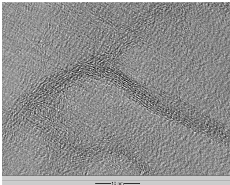
Figure S2. A TEM image showing wrinkles on the surface of RGO.
