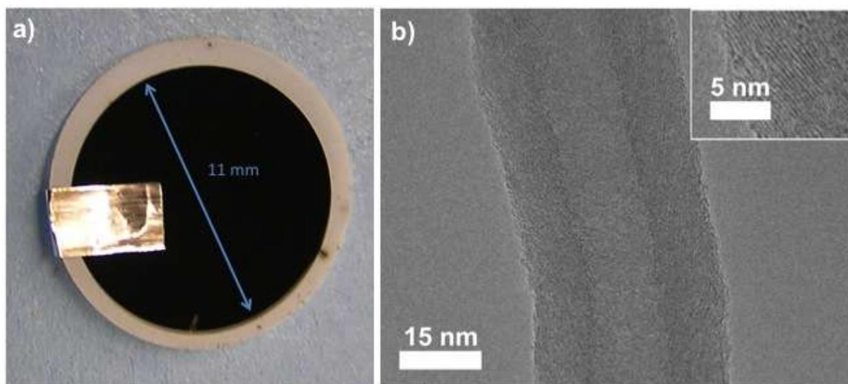
**Fig. S1:** Electrode Fabrication. a, Photograph of the filter after nanofiber synthesis. The filter diameter is 13 mm, and the area covered by CNFs has an 11 mm diameter. To prepare the electrode, a piece of aluminum foil is wrapped around one edge. b, High-resolution Transmission Electron Microscope (HR-TEM) bright field image of a typical nanofiber synthesized using this process. The average diameter of the fibers used in this study is roughly ~30 nm.
