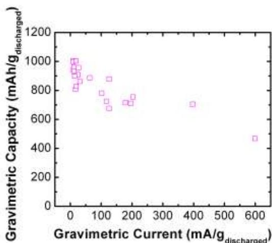
**Fig. S4:** Reproducibility of discharge capacity normalized to the weight of discharged electrodes (C + Li<sub>2</sub>O<sub>2</sub>) of CNF electrodes in O<sub>2</sub> cells tested over a range of gravimetric electrode currents (lower cutoff of 2.0 V vs. Li).
