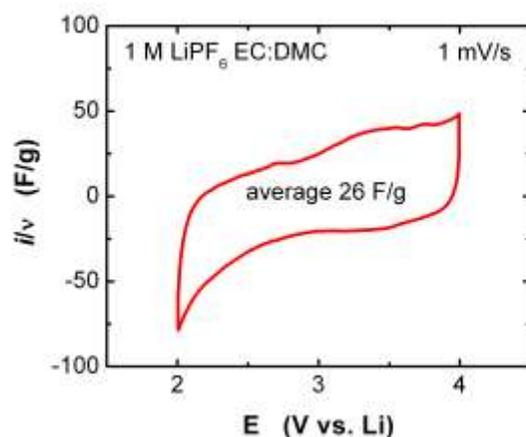
**Fig. S2:** Cyclic voltammetry of a CNF electrode in a Li cell (1 M LiPF<sub>6</sub> electrolyte in EC:DMC) indicated that CNF electrodes have an average capacitance of 26 F/g in the range 2.0 – 4.0 V vs. Li.
