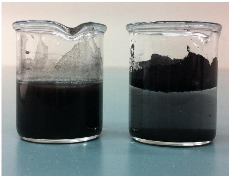
**Fig. S2.** Photos showing that Fe<sub>3</sub>O<sub>4</sub>/C particles are fully dispersed in water after addition of a small amount of polyvinylpyrrolidone as a dispersant (left), and the majority of Fe<sub>3</sub>O<sub>4</sub>/C particles still float on water after stirring overnight, and boiling and ultrasonication for hours (right).
