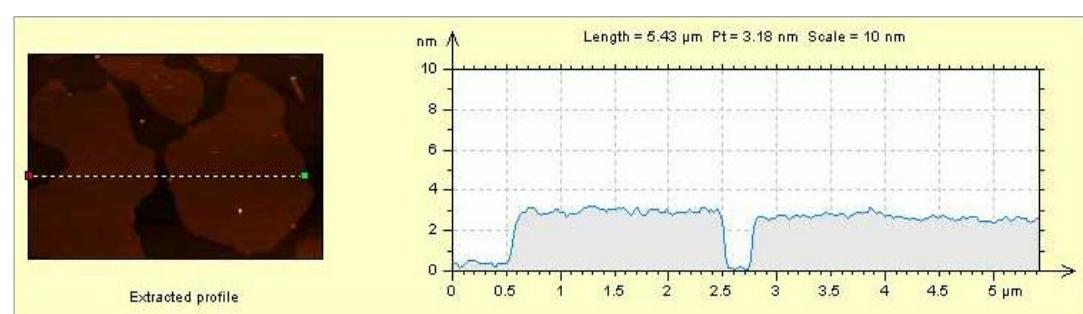
**Figure S2.** AFM images and the corresponding height profile of GO nanosheets.
