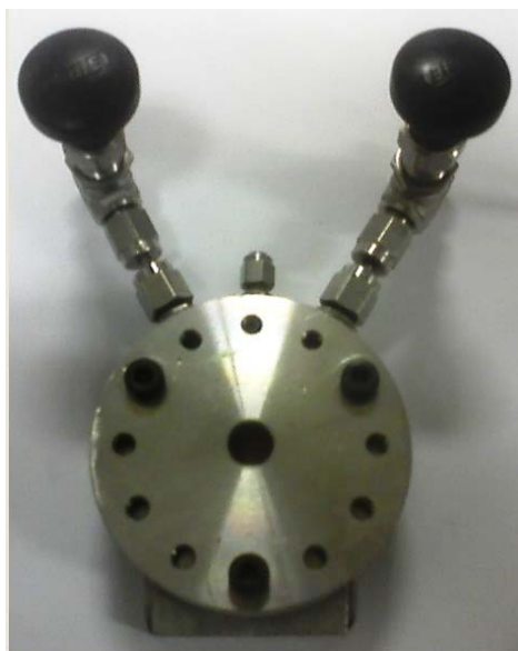
Fig. S-6 A photograph of a high pressure FT-IR cell.
