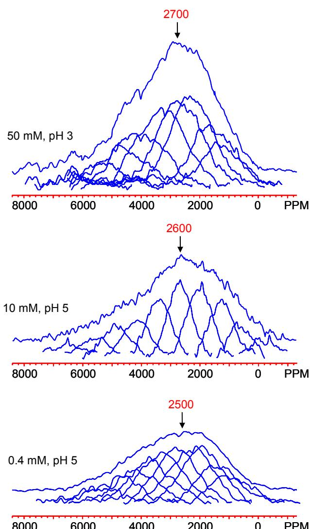
Figure S6. Spin echo mapping  $^{31}\text{P}$  NMR spectra of phosphate-adsorbed goethite at various phosphate concentrations and pH. The NMR spectra of 0.4 and 10 mM samples are normalized according to the number of scans (free induction decays) used to acquire each individual spectrum.
