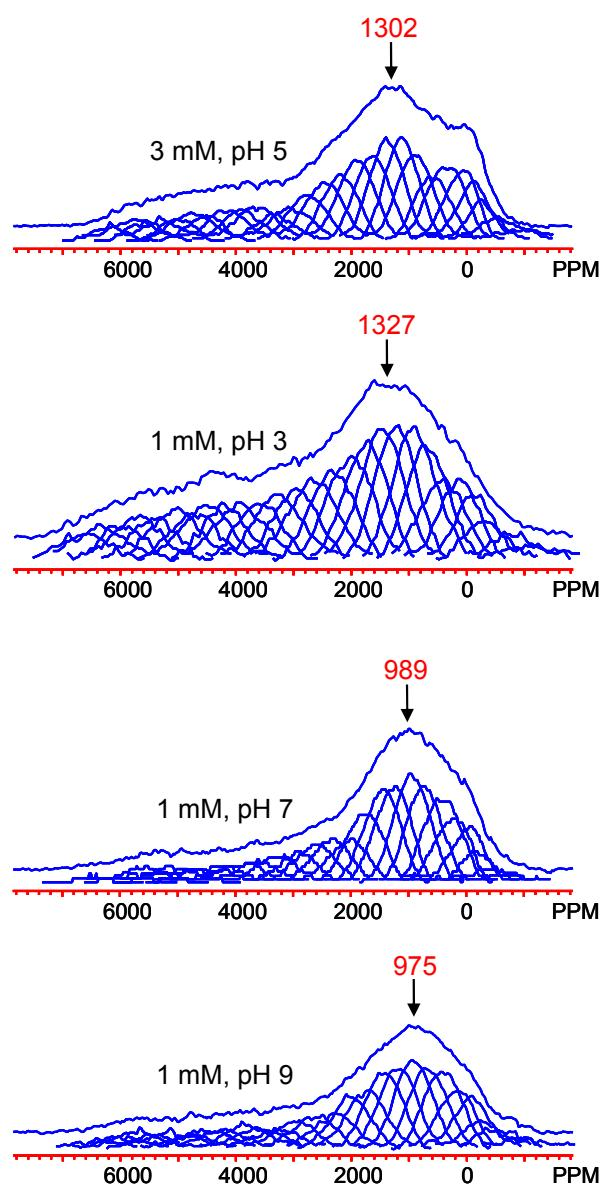
Figure S8. Spin echo mapping  $^{31}\text{P}$  NMR spectra of phosphate adsorbed akaganeite at a 3mM phosphate concentration and pH 5 and as a function of pH at a 1mM phosphate concentration. The NMR spectra, except for pH 3 sample, are normalized.
