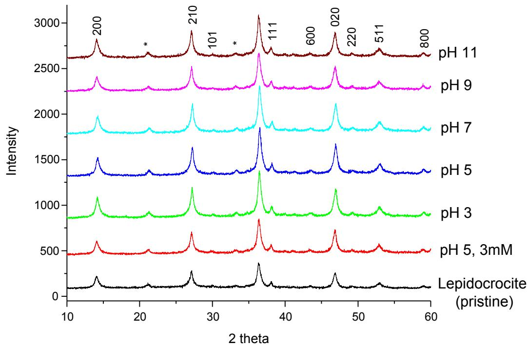
Figure S3. X-ray powder diffractions for phosphate adsorbed lepidocrocite samples at a 1mM initial phosphate concentration as a function of pH and at a 3mM initial phosphate concentration and pH 5. (\*) denotes the reflection due to the goethite impurity, present in all the samples.
