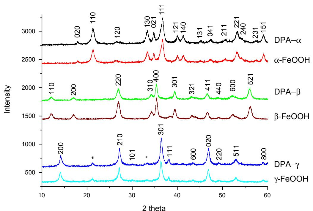
Figure S4. X-ray powder diffractions for dimethyl phosphinic acid (DPA) adsorbed FeOOH samples at a 10 mM initial phosphate concentration and pH 5. (\*) denotes the reflection due to the goethite impurity. The DPA-sorbed goethite, akaganeite, and lepidocrocite samples were labeled as DPA- $\alpha$ , DPA- $\beta$ , and DPA- $\gamma$ , respectively.
