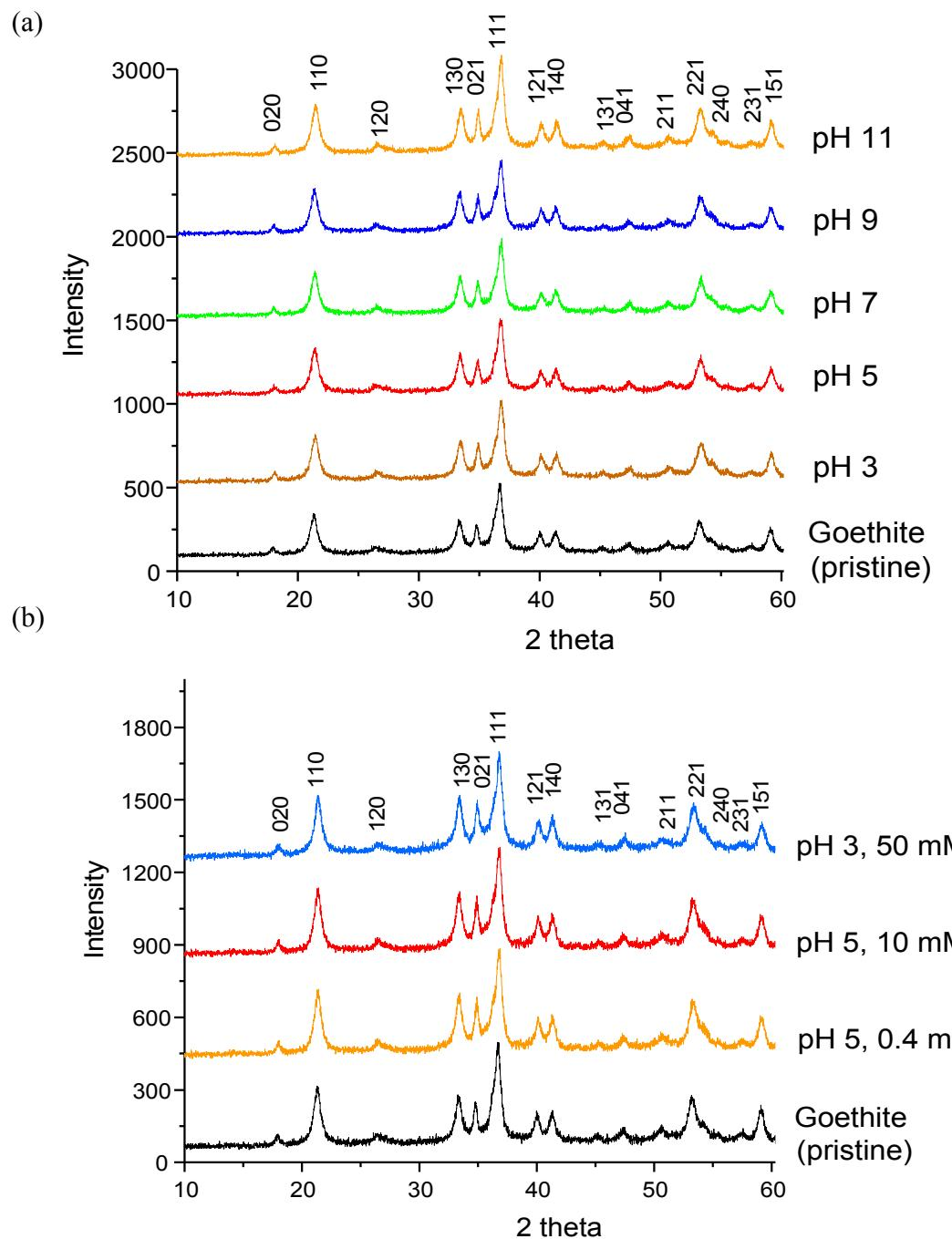
Figure S1. X-ray powder diffractions for phosphate-adsorbed goethite samples (a) at 1mM initial phosphate concentration as a function of pH and (b) at various pH values and initial concentrations.
