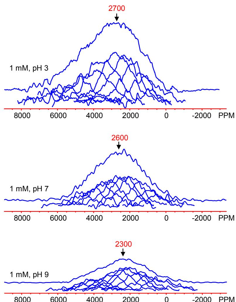
Figure S7. Spin echo mapping  $^{31}\text{P}$  NMR spectra of phosphate adsorbed goethite at a 1mM phosphate concentration as a function of pH. The NMR spectra have been normalized according to the number of scans used for each experiment.
