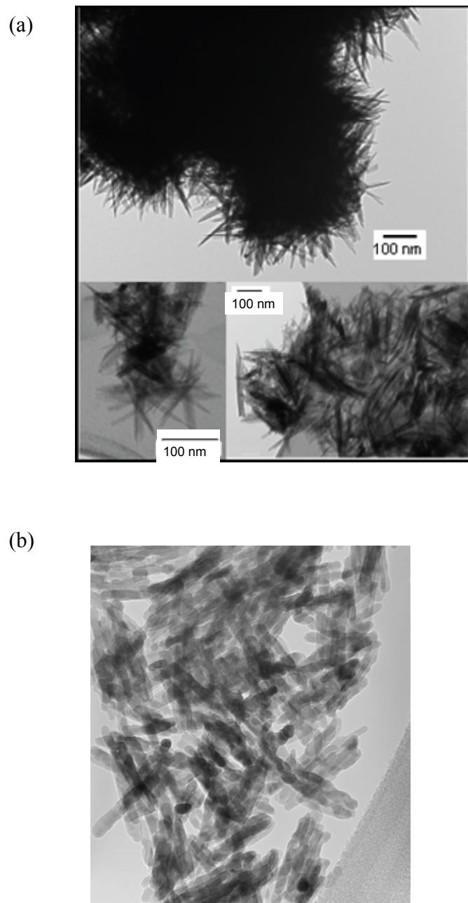
Figure S5. Transmission Electron Microscope (TEM) images of (a) goethite and (b) akaganeite.
