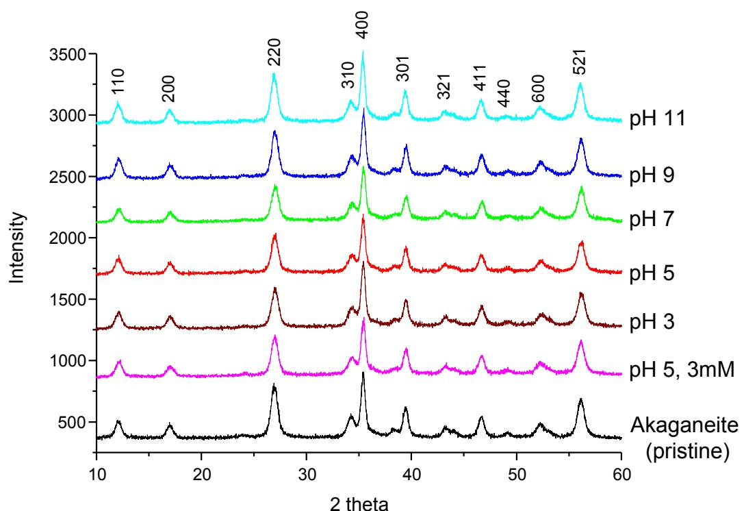
Figure S2. X-ray powder diffractions for phosphate-adsorbed akaganeite samples at a 1mM initial phosphate concentration as a function of pH, and at a 3mM initial phosphate concentration and pH 5.
