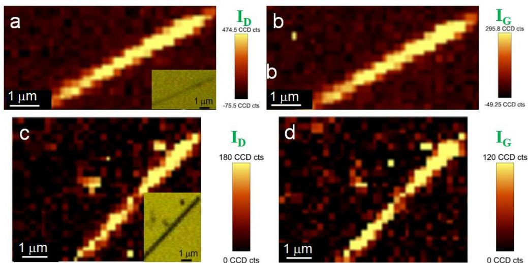
**Fig. S4.** Raman mapping images of the D and G bands of graphene for different individual graphene@SnO<sub>2</sub> NWs, revealing the full coverage along the SnO<sub>2</sub> NW. Insets in Fig. S4a and S4c show the optical images of the selected graphene@SnO<sub>2</sub> NWs.
