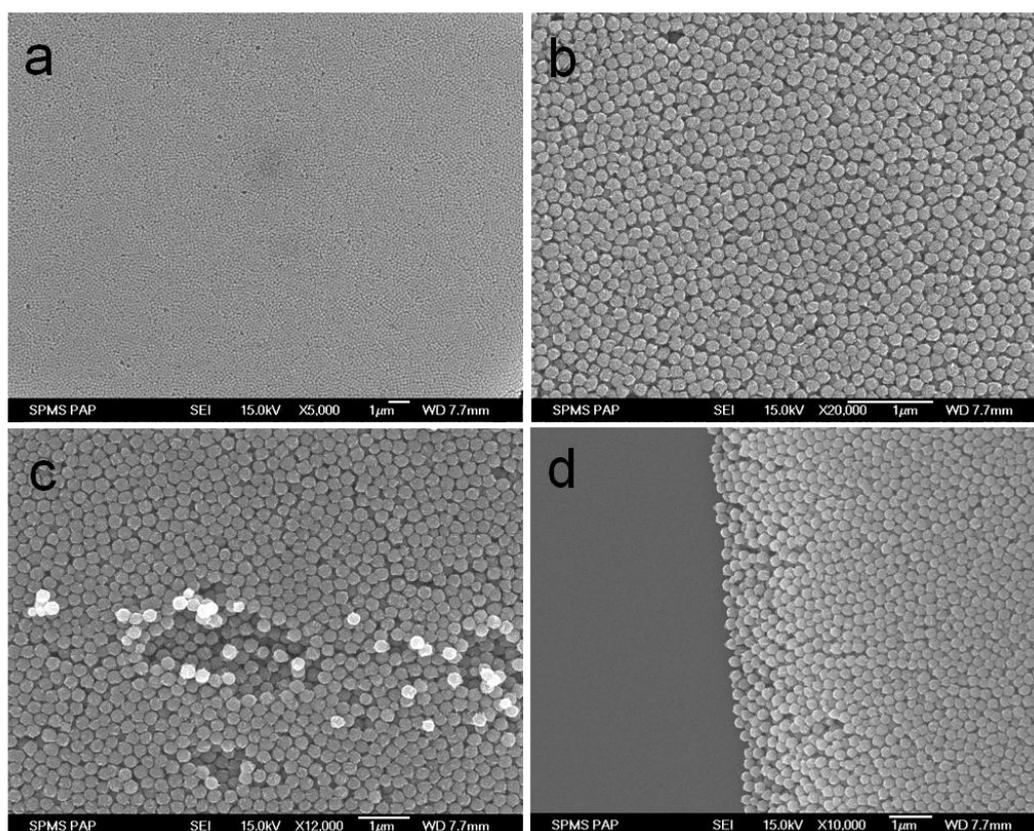
**Fig. S7.** SEM images of the as-obtained  $\alpha$ - $\text{Fe}_2\text{O}_3$  precursor, revealing a highly ordered stacking fashion.
