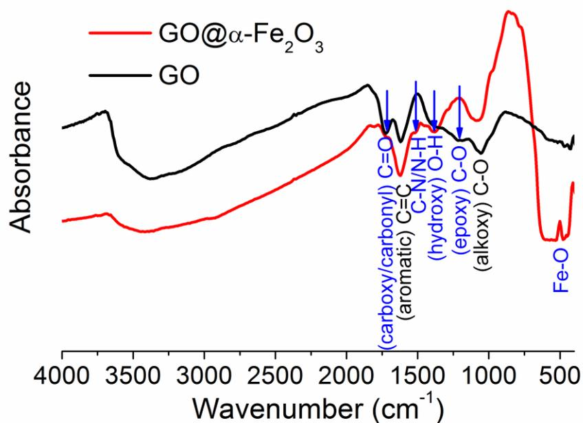
**Fig. S10.** FT-IR spectra of GO and GO@ $\alpha$ -Fe<sub>2</sub>O<sub>3</sub>. Compared with pure GO, the epoxy C-O stretch at 1220 cm<sup>-1</sup> disappears in the FT-IR spectrum of GO@ $\alpha$ -Fe<sub>2</sub>O<sub>3</sub>. As GO contains reactive epoxy groups, its exposure to amine groups could lead to a ring-opening reaction, creating new C-N and O-H bonds.<sup>3</sup> An appearance of a new peak at 1510 cm<sup>-1</sup>, which corresponds to a stretching of the new C-N bonds and
