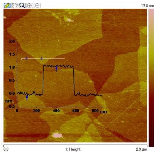
**Fig. S2.** AFM image of the as-obtained GO platelets. Inset is depth profile of the line of interest on the GO platelets, the height difference between two arrows is about 1 nm, indicating a single layer GO sheet.
