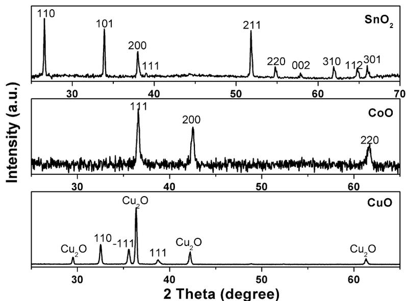
**Fig. S1.** XRD patterns of the as-obtained oxide NWs. The Cu<sub>2</sub>O phase appearing in the XRD pattern of CuO is believed to exist as a thin film precursor for growing CuO NWs during the oxidation of Cu plate.<sup>1,2</sup>
