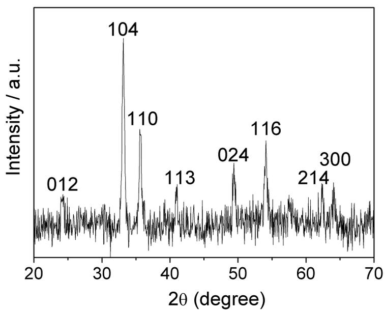
**Fig. S8.** XRD pattern of the as-prepared  $\alpha$ - $\text{Fe}_2\text{O}_3$  NPs (JCPDS 33-0664).
