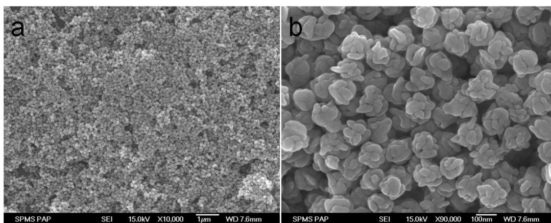
**Fig. S9.** SEM images of the as-obtained  $\alpha$ -Fe<sub>2</sub>O<sub>3</sub> NPs, showing high uniformity.
