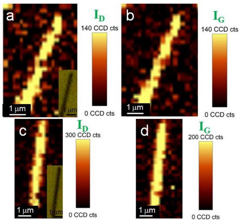
**Fig. S5.** Raman mapping images of the D and G bands of graphene for different single graphene@CuO NWs. Insets in Fig. S5a and S5c show the optical images of the selected graphene@CuO NWs.
