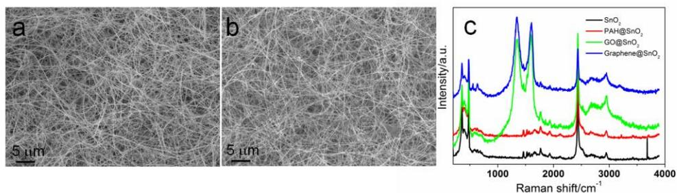
**Fig. S3.** Low-magnification SEM images of the SnO<sub>2</sub> NWs: (a) before, and (b) after graphene coating. (c) Raman spectra of the products at different steps, corresponding to the scheme illustrated in Fig. 1c.
