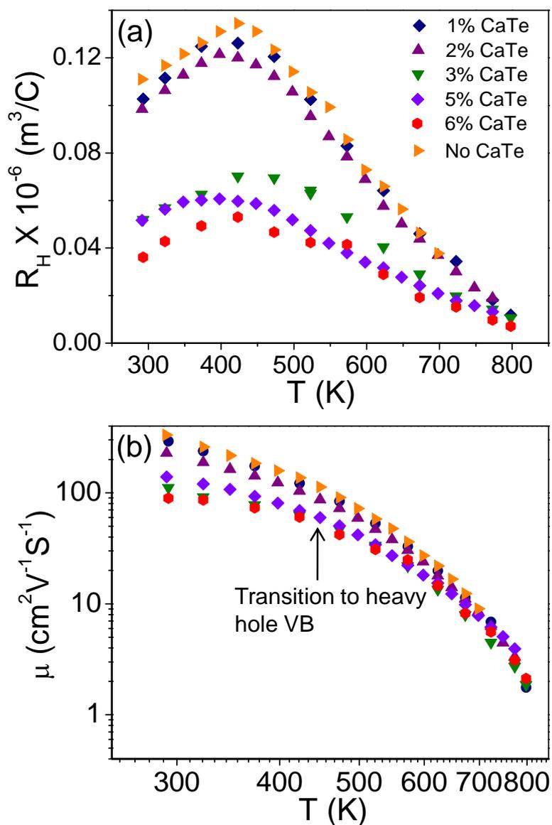
**Fig. S1** Temperature dependent (a) Hall coefficient and (b) hole mobility data (log-log scale plot) of PbTe-CaTe samples doped with 1 % Na<sub>2</sub>Te and a control sample, PbTe doped with 1 % Na<sub>2</sub>Te. Decrease in the mobility was observed at ~450 K due to transition to the transition to the heavy hole valence band.
