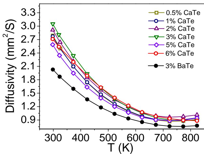
**Fig. S2** Temperature dependent thermal diffusivity data of all the PbTe-CaTe and PbTe-BaTe samples doped with 1% Na<sub>2</sub>Te. Thermal diffusivities were measured using laser flash diffusivity method in a Netzsch LFA-457.
