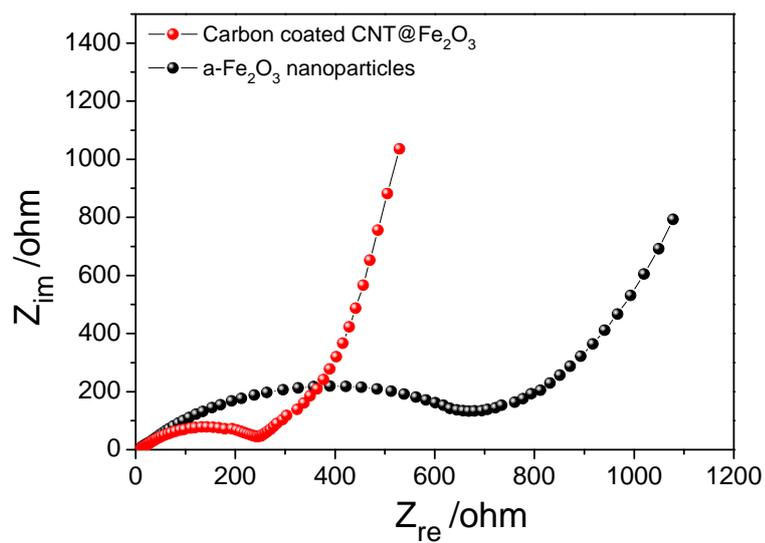
**Figure S9** Nyquist plots of the electrodes composed of the hierarchical structures of carbon coated CNT@Fe<sub>2</sub>O<sub>3</sub> or  $\alpha$ -Fe<sub>2</sub>O<sub>3</sub> nanoparticles.
