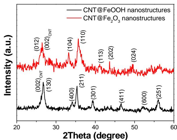
**Figure S1** XRD profiles of CNT@FeOOH and CNT@Fe<sub>2</sub>O<sub>3</sub> hierarchical structures.
