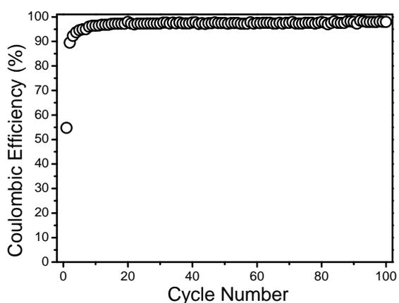
**Figure S8** Coulombic efficiency of carbon coated CNT@Fe<sub>2</sub>O<sub>3</sub> structures cycled between 0.01 – 3V at a current density of 500 mA g<sup>-1</sup>.
