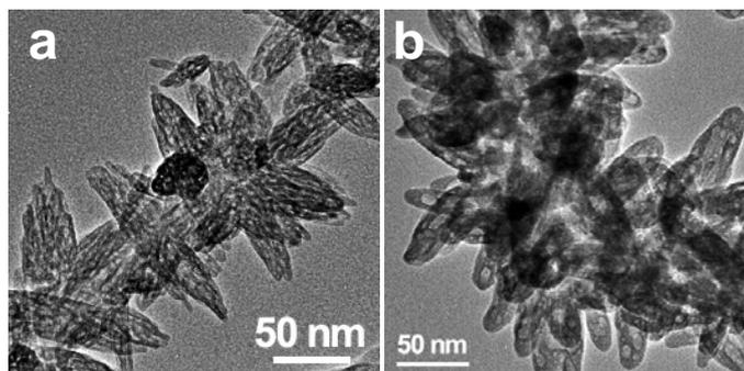
**Figure S4** TEM images of  $\text{CNT@Fe}_2\text{O}_3$  structures obtained by annealing at different temperature: (a) 250 °C, (b) 300 °C.
