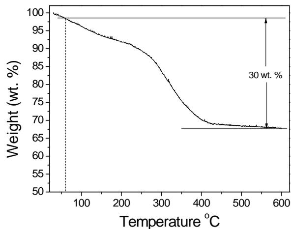
**Figure S6** Thermogravimetric analysis of carbon coated CNT@Fe<sub>2</sub>O<sub>3</sub> structures. The test was conducted in air with a ramp rate of 10 °C min<sup>-1</sup>.
