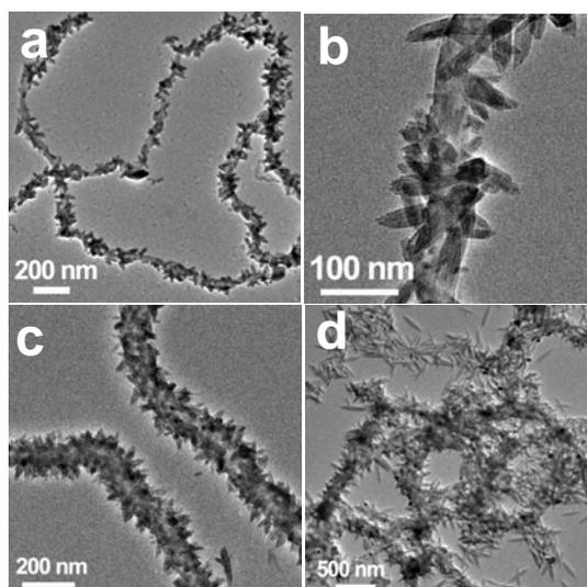
**Figure S3** TEM images of the samples obtained by the hydrolysis of  $\text{FeCl}_3$  with various initial concentration: (a, b) 0.03 M, (c) 0.06 M, (d) 0.36 M.
