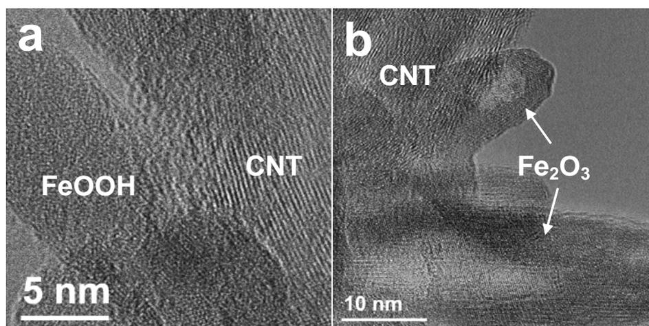
**Figure S2** HRTEM images of CNT@FeOOH and CNT@Fe<sub>2</sub>O<sub>3</sub> hierarchical structures.
