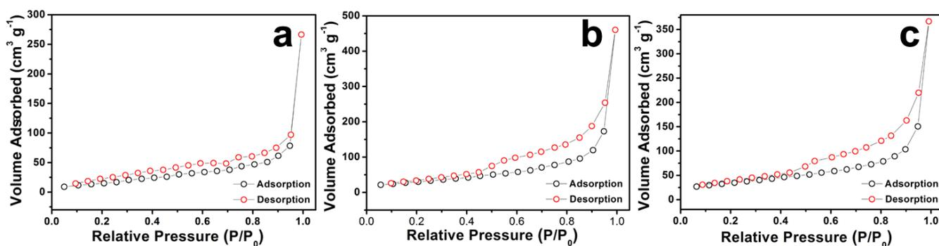
**Figure S5**  $\text{N}_2$  adsorption/desorption isotherms of (a)  $\text{CNT@FeOOH}$ , (b)  $\text{CNT@Fe}_2\text{O}_3$  and (c) carbon coated  $\text{CNT@Fe}_2\text{O}_3$  hierarchical structures.
