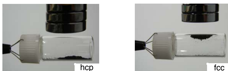
Fig. S4. Difference in magnetic properties between hcp -NiNPs and fcc -NiNPs. fcc -NiNPs are attracted to a magnet.
