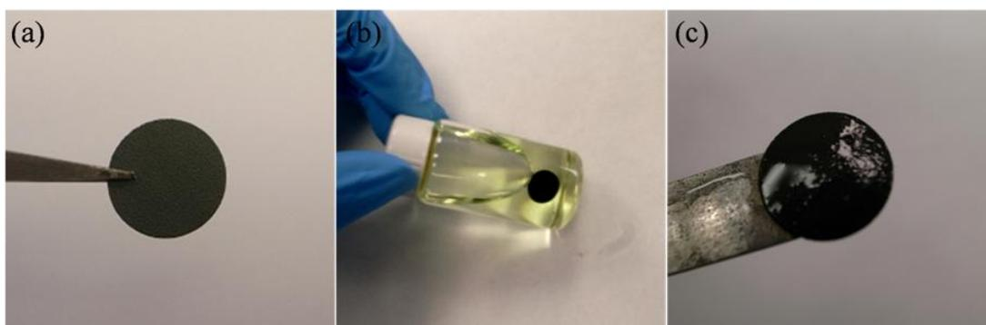
**Figure S6.** (a) A small disc-shape CNT/V<sub>2</sub>O<sub>5</sub> nanocomposite electrode with 25 wt-% of CNTs. (b) The electrode was soaked in 37 wt-% HCl. The light-yellow color indicates the dissolution of V<sub>2</sub>O<sub>5</sub> in the acid. (c) Digital photograph of the free-standing CNT sheets after dissolving V<sub>2</sub>O<sub>5</sub> nanowires, maintaining its structure integrity.
