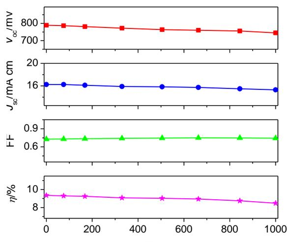
**Fig. S2** Detailed photovoltaic parameters measured under the irradiance of the  $100 \text{ mW cm}^{-2}$  simulated AM1.5G sunlight for a cell with the liquid electrolyte during successive full sunlight soaking at  $60 \text{ }^\circ\text{C}$ .
