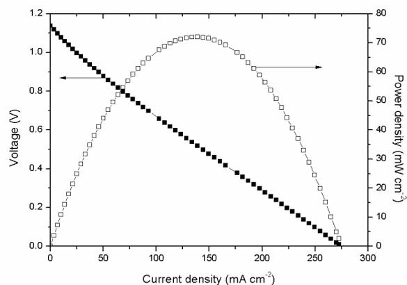
Supplementary Fig. S1 Hybrid direct carbon fuel cell performance and current-voltage characteristics of the cell with a 1 mm thick yttria-stabilized zirconia electrolyte, a NiO/YSZ composite anode and a LSM/YSZ composite cathode by screen printing, pyrolysed medium density fiberboard (PMDF) as the fuel, flow rate of N<sub>2</sub> purge gas is 20 ml/min, tested at 750 °C.
