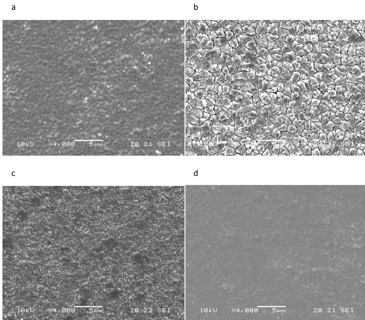
Supplementary Fig. S5 Surface microstructures of 8 mol% yttrium stabilised zirconia pellets. a, before corrosion test; b, etched in lithium-potassium carbonate in air at 700 °C for 10 hrs; c, etched in lithium-potassium carbonate in argon at 700 °C for 10 hrs; d, etched in lithium-potassium carbonate in 5%H<sub>2</sub>/Ar at 700 °C for 10 hrs.
