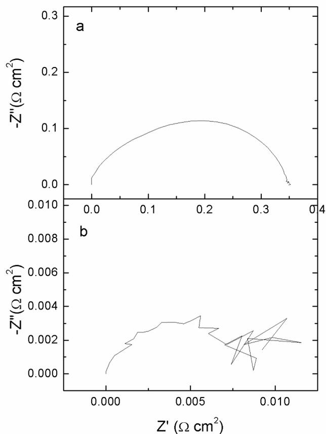
Supplementary Fig. S2 AC impedance spectra of the symmetric cells with a composite electrode of  $(\text{La}_{0.8}\text{Sr}_{0.2})_{0.95}\text{MnO}_3$  and YSZ (50:50 weight ratio) on a YSZ pellet (a);  $\text{La}_{0.6}\text{Sr}_{0.4}\text{CoO}_3$  electrode on a  $\text{Ce}_{0.9}\text{Gd}_{0.1}\text{O}_2$  pellet (b). Note: the ohmic resistance was subtracted.
