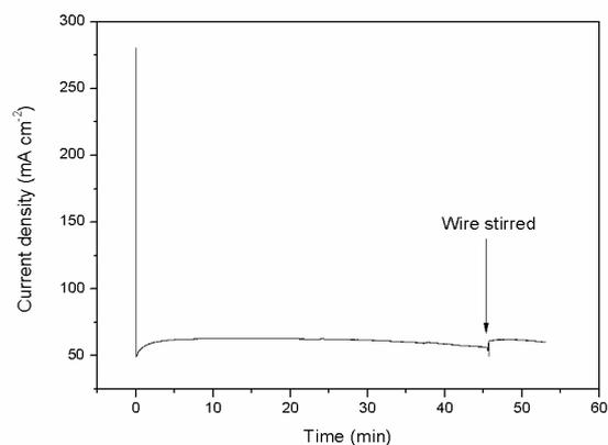
Supplementary Fig. S3 Short term stability of the hybrid direct carbon fuel cell with a 1 mm thick YSZ electrolyte, a screen printed NiO/YSZ (60:40 by weight ratio) anode and a LSM/YSZ cathode in a weight of 50 to 50. The open circuit voltage was 1.10 V and applied voltage was 700 mV. Stirring the current collection wire during the test prevented degrading, which might be from the carbon consumption around the current collection.
