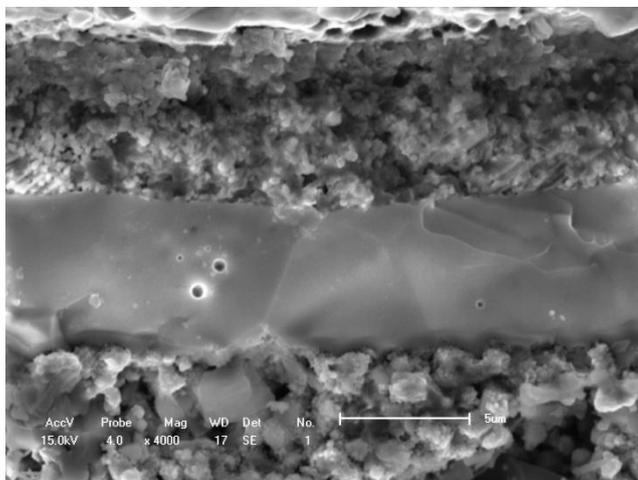
Supplementary Fig. S4 Cross section of the cell with a composite cathode of LSM-YSZ composite cathode, a YSZ electrolyte and a nickel cermet anode after electrochemical measurement. This cell has been operated for 2.5 hours at 500 mV with current density ranging from 384 to 160 mA cm<sup>-2</sup>. The gas flow rate was 20 ml min<sup>-1</sup> CO<sub>2</sub>.
