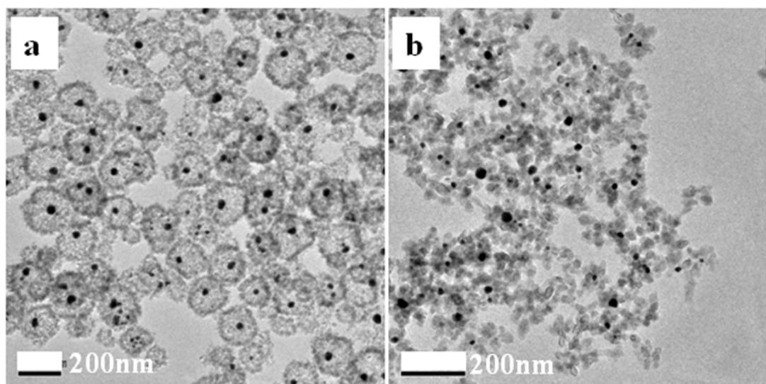
**Fig. S1** TEM images of Au@TiO<sub>2</sub> hollow submicrospheres (thin shell), (a) with ethanol and (b) without ethanol.
