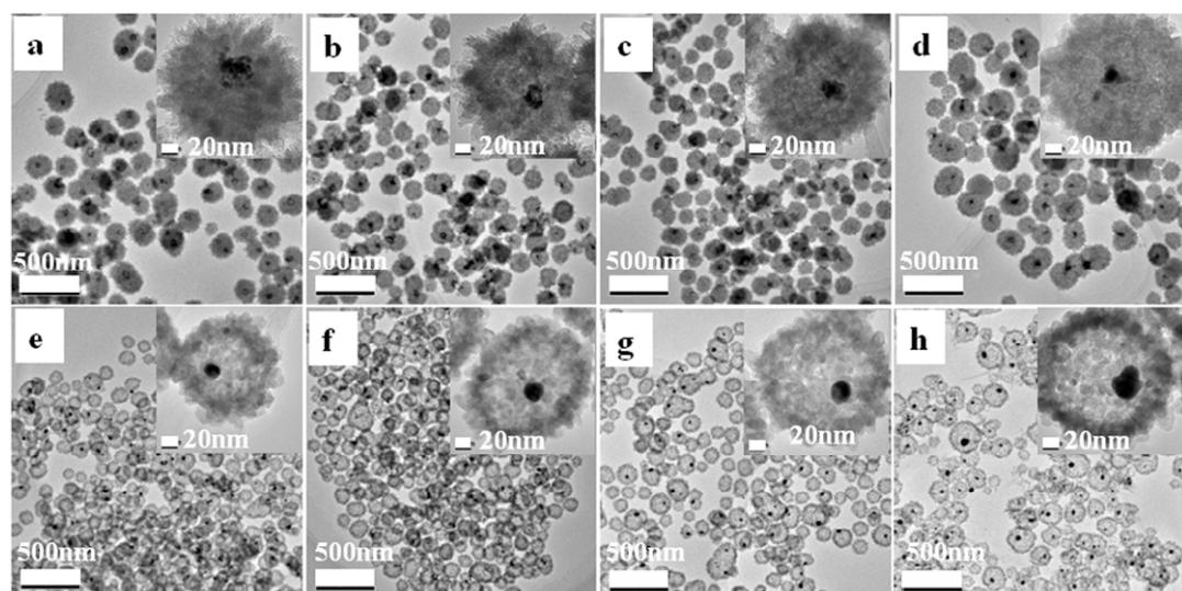
**Fig. S6** TEM images of Au@TiO<sub>2</sub> hollow submicrospheres with thin shell at different crystallization temperatures : a) 50 °C, b) 60 °C, c) 75 °C, d) 100 °C, e) 120 °C, f) 140 °C, g) 160 °C and h) 180 °C for 6 h. Insets in a) – h) are corresponding enlarged TEM images.
