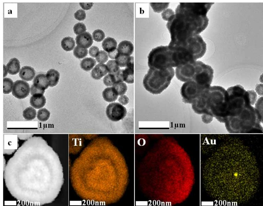
**Fig. S7** TEM images of Au@TiO<sub>2</sub> hollow submicrospheres, a) Au@TiO<sub>2</sub> submicrospheres with single shell, b) Au@TiO<sub>2</sub> submicrospheres with double shells, c) is the HAADF-STEM image and HAADF-STEM-EDS mapping images of b).
