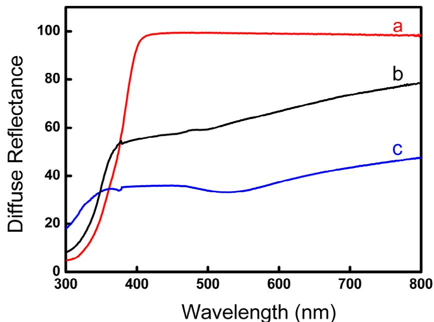
**Fig. S9** Diffuse reflectance of a) P25, b) TiO<sub>2</sub> hollow submicrospheres with thin shell, and c) Au@TiO<sub>2</sub> hollow submicrospheres with thin shell
