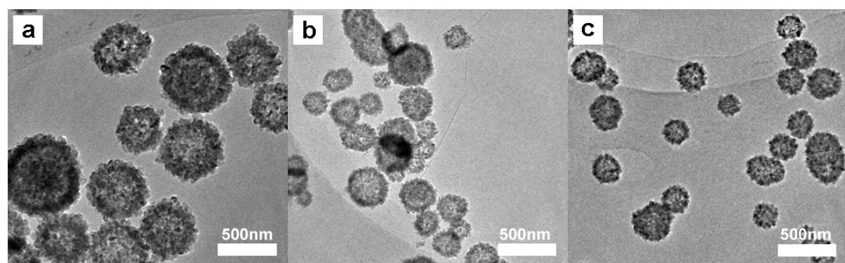
**Fig. S8** TEM images of TiO<sub>2</sub> hollow submicrospheres with a) thick shell, b) medium-thickness shell and c) thin shell.
