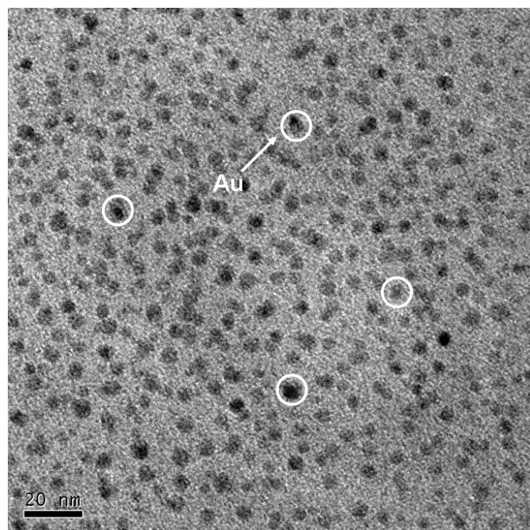
**Fig. S3** TEM image of Au NPs for preparation of Au@TiO<sub>2</sub> hollow submicrospheres.
