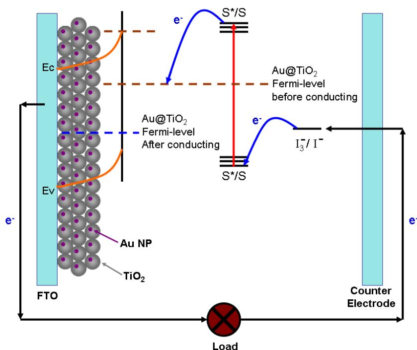
**Fig. S10** Scheme of the charge separation process in the DSSCs with the photoanode of Au@TiO<sub>2</sub> hollow submicrospheres.
