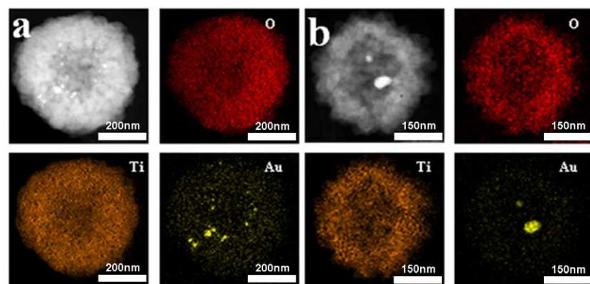
**Fig. S2** HAADF-STEM image and HAADF-STEM-EDS mapping images of Au@TiO<sub>2</sub> hollow submicrospheres with a) thick shell and b) medium-thickness shell.
