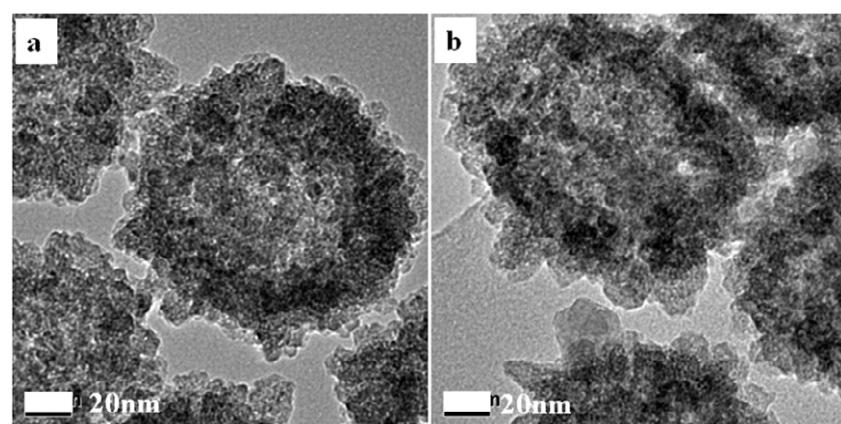
**Fig. S4** TEM images of Au@TiO<sub>2</sub> hollow submicrospheres with thin shell at 180 °C via different crystallization times: a) 1 min or b) 2 min.
