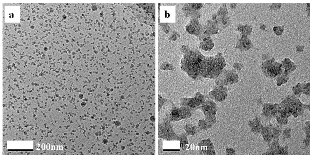
**Fig. S5** TEM image of a) the product synthesized at room temperature for 6 h, b) is corresponding enlarged TEM image.
