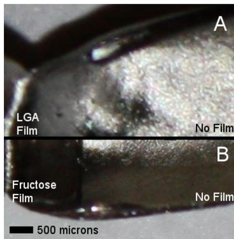
**Figure S1.** Photos of levoglucosan (A) and fructose (B) thin-films within the pyrolysis crucible. Areas with no reflection indicate the presence of a thin-film (far left) while regions with light reflectance indicate no thin-film (far right).
