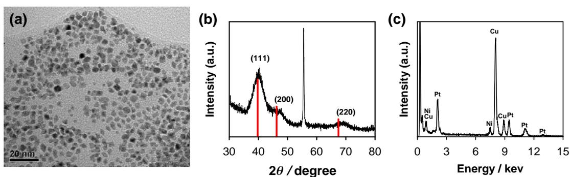
**Fig. S6** TEM image (a), XRD pattern (b), and EDX spectrum (c) of GN-Pt<sub>3</sub>Ni hybrids. Monodisperse nanoparticles grown on GN can be observed (Fig. S6a). The diffraction peaks slightly shift to higher angles compared with those for pure Pt (Fig. S6b), indicating the formation of Pt-Ni alloy. The energy-dispersive X-ray (EDX) analysis suggests that the average molar ratio between Pt and Ni is 3:1. These results clearly indicate the formation of GN-Pt<sub>3</sub>Ni hybrids.
