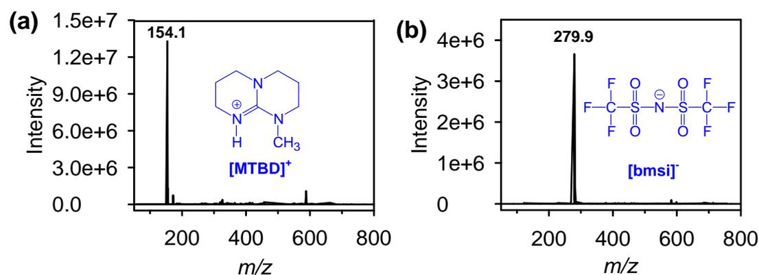
**Fig. S8** Mass spectrum of [MTBD][bmsi] IL recorded in positive ion mode (a) and negative ion mode (b).
