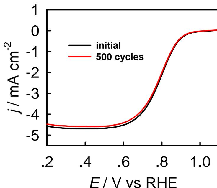
**Fig. S7** ORR polarization curves for GN-Pt-IL catalyst in 0.5 M O<sub>2</sub>-saturated H<sub>2</sub>SO<sub>4</sub> solution at a sweep rate of 10 mV s<sup>-1</sup> and a rotation rate of 1,600 rpm before and after 500 potential cycles. The potential cycles were from 0.5 to 1.0 V in 0.5 M O<sub>2</sub>-saturated H<sub>2</sub>SO<sub>4</sub> solution at room temperature at a sweep rate of 10 mV s<sup>-1</sup> and a rotation rate of 1,600 rpm.
