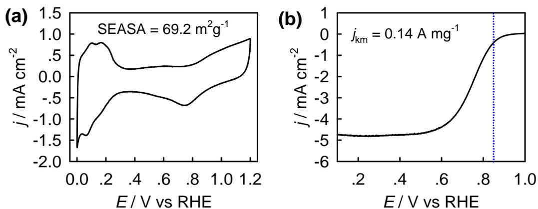
**Fig. S4** (a) Cyclic voltammograms for commercial Pt/C catalyst in 0.5 M H<sub>2</sub>SO<sub>4</sub> aqueous solution at 50 mV s<sup>-1</sup>. (b) ORR polarization curves for commercial Pt/C catalyst recorded at room temperature in an O<sub>2</sub>-saturated 0.5 M H<sub>2</sub>SO<sub>4</sub> aqueous solution at a sweep rate of 10 mV s<sup>-1</sup> and a rotation rate of 1,600 rpm.
