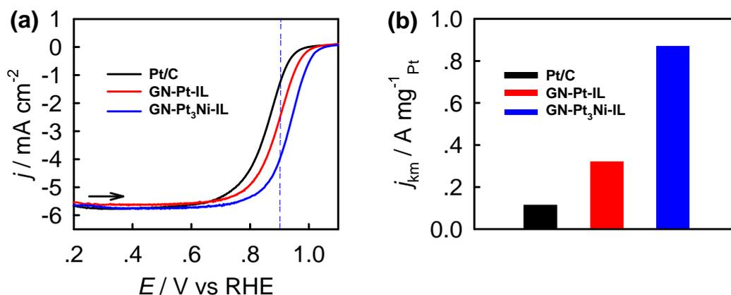
**Fig. S5** (a) ORR polarization curves for Pt/C, GN-Pt-IL, and GN-Pt<sub>3</sub>Ni-IL catalysts in 0.1 M O<sub>2</sub>-saturated HClO<sub>4</sub> solution at a sweep rate of 10 mV s<sup>-1</sup> and a rotation rate of 1,600 rpm. (b) Mass activity ( $j_{\text{km}}$ ) at 0.9 V for these three catalysts, which is given as kinetic current densities ( $j_{\text{k}}$ ) normalized to the Pt mass. the Pt loadings for all catalysts were 15.3  $\mu\text{g cm}^{-2}$ .
