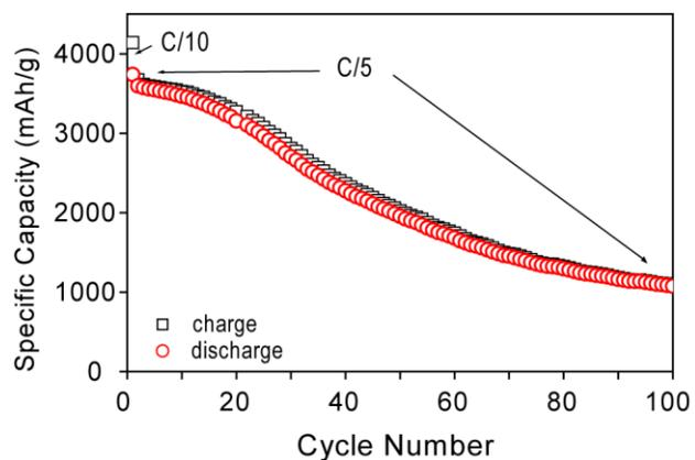
**Figure S3** Capacity vs. cycle number for pristine Si NWs.
