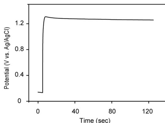
**Figure S1** Potential profile of Si NWs electrode during electrochemical polymerization with 0.1 M LiClO<sub>4</sub> in acetonitrile electrolyte. An Ag/AgCl electrode was used as the reference, and Pt was used as the counter electrode. A current of 1 mA/cm<sup>2</sup> was passed for 2 minutes, which causes the EDOT monomers to become electro-oxidized and to polymerize at a potential of ~1.3 V vs. Ag/AgCl.
