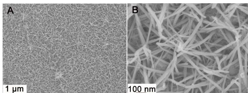
**Figure S2.** Typical FESEM images of the precursor nanowires by adding 48 mmol of urea in the reaction, which is double of the amount used for the product shown in Figure 1 in the maintext.
