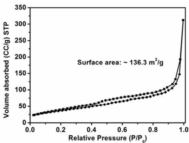
**Figure S4.** N<sub>2</sub> adsorption-desorption isotherm of the NiCo<sub>2</sub>O<sub>4</sub> nanoneedles.
