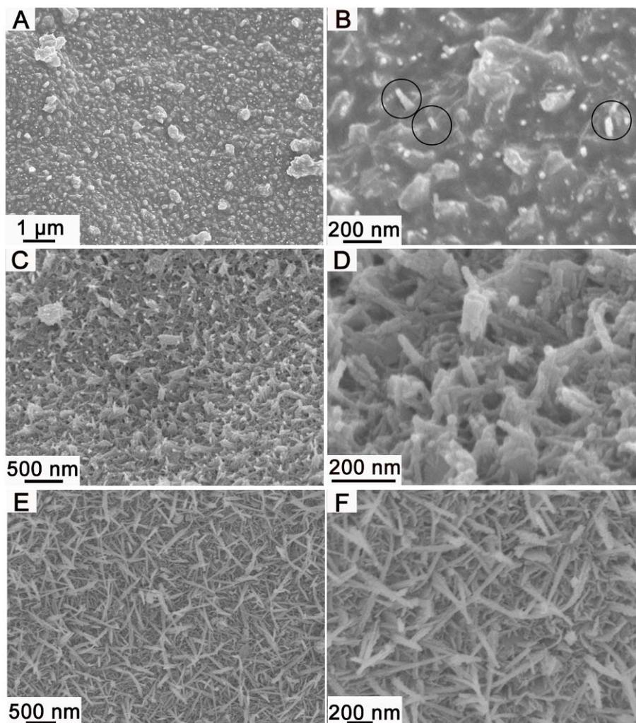
**Figure S3.** FESEM images of precursor nanowires on Ni foam with different reaction durations: (A, B) 30 min; (C, D) 2 h; and (E, F) 3 h.
