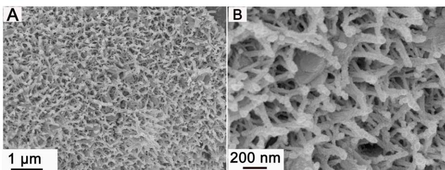
**Figure S5.** FESEM images of the NiCo<sub>2</sub>O<sub>4</sub> nanowire arrays on Ni foam after charged/discharged for 2000 cycles at a current density of 5.56 mA cm<sup>-2</sup>.
