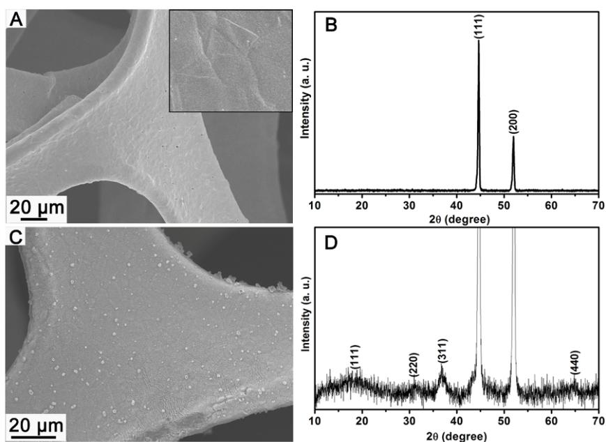
**Figure S1.** Typical FESEM images and corresponding XRD patterns of bare Ni foam and NiCo<sub>2</sub>O<sub>4</sub> nanoneedle arrays/Ni foam hybrid structure: (A) FESEM image of bare Ni foam after the acid etching treatment, and (B) corresponding XRD pattern. (C) FESEM image of Ni foam after growing NiCo<sub>2</sub>O<sub>4</sub> nanoneedles, and (D) corresponding XRD pattern.
