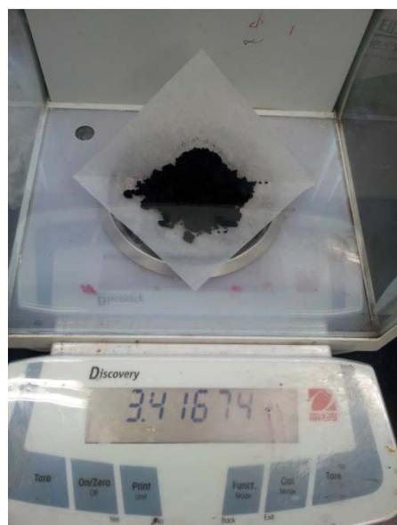
**Figure S9.** Photograph of C-Fe<sub>3</sub>O<sub>4</sub> nanocomposite synthesized in large-scale, showing 3.42 g of the product.
