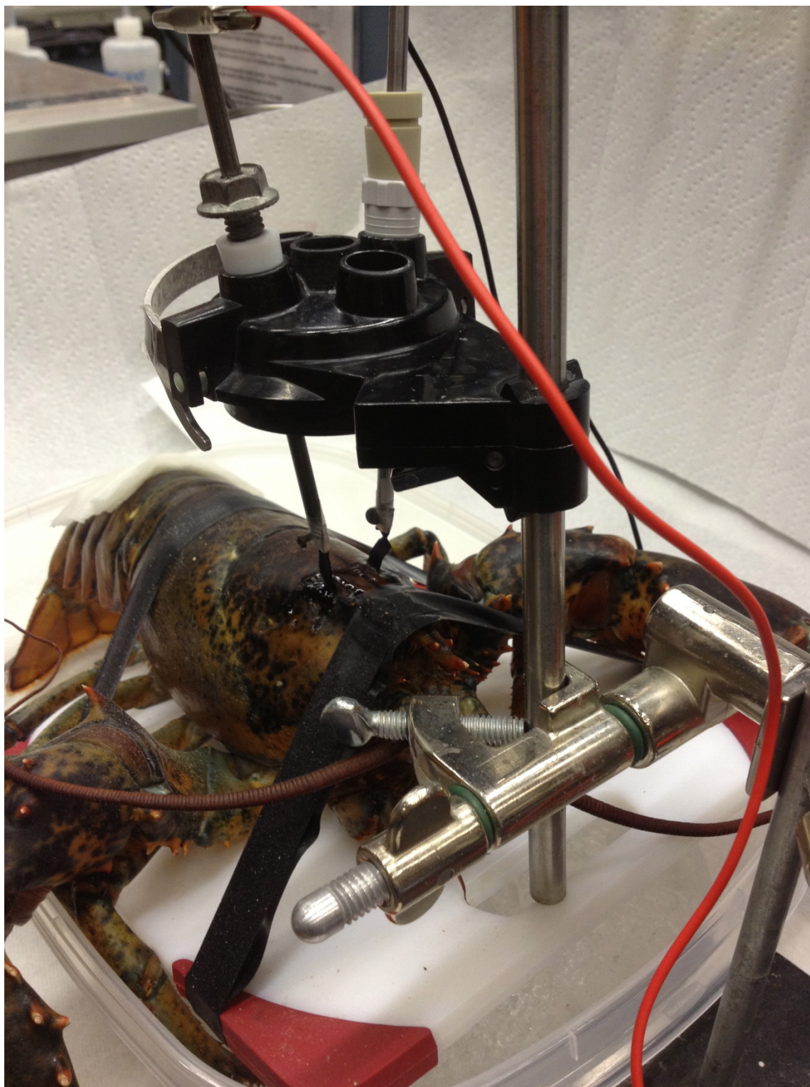
Lobster with the implanted biocatalytic electrodes
